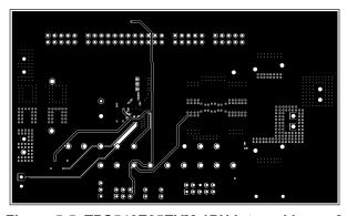
Figure 5-5. TPS546E25EVM-1PH Internal Layer 2 (Top View)
