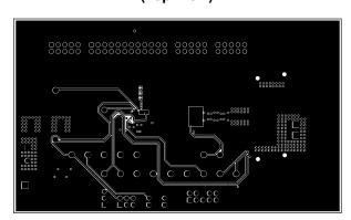
Figure 5-6. TPS546E25EVM-1PH Internal Layer 3 (Top View)
