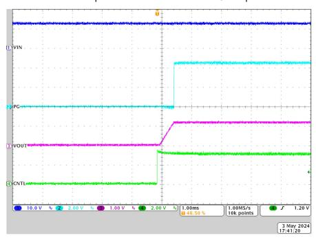
Figure 4-6. Start-Up From Control, 0A Load
