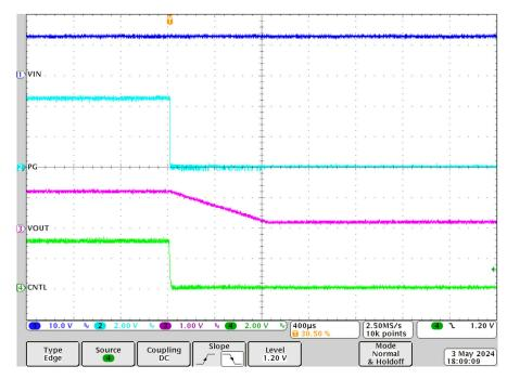
Figure 4-7. Shutdown From Control, 0A Load
