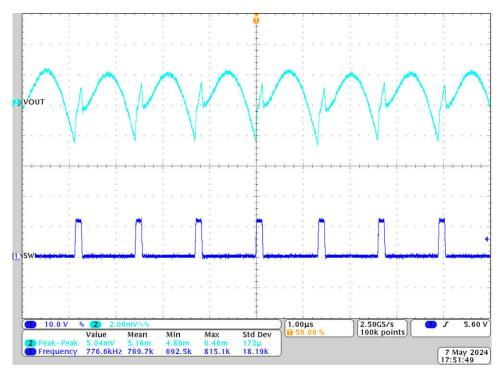
Figure 4-5. Output Ripple With 25A Load
