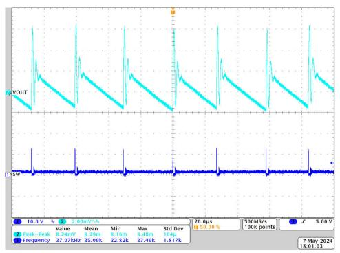
Figure 4-4. Output Ripple With 0A Load
