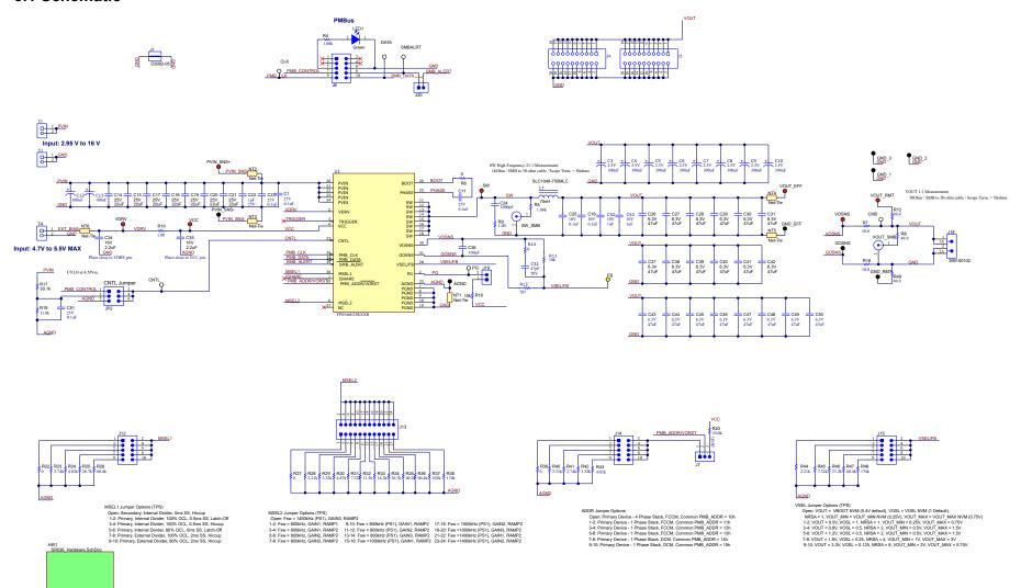
Figure 5-1. TPS546E25EVM-1PH Schematic
