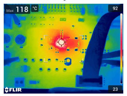
$V_{IN}$  = 12V,  $V_{OUT}$  = 1.2V,  $I_{OUT}$  = 50A
