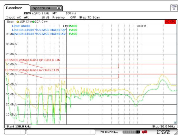
**Figure 3-35. VIN = 230 V<sub>RMS</sub>, VOUT = 20 V, Load = 3.25 A (Output Not Grounded to LISN Ground)**
