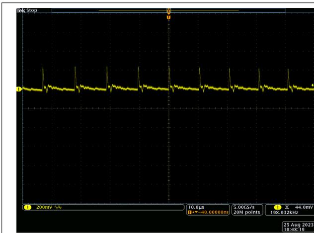
Figure 3-27. Typical Ripple Voltage of  $V_{OUT} = 9\text{ V}$
