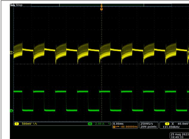
Figure 3-30. Load Transient Response at  $V_{OUT} = 20$  V
