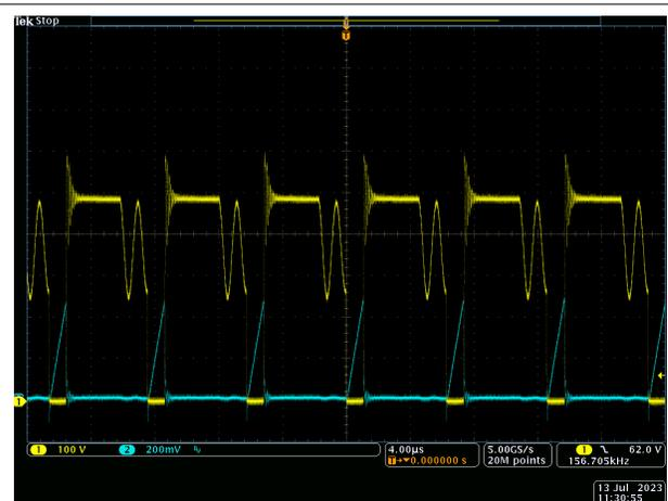
Figure 3-12. Vin = 265Vac, Vout = 20 V
