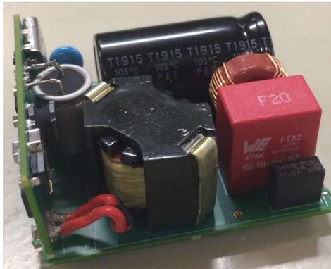
**Figure 2-1. High-Density Configuration**
