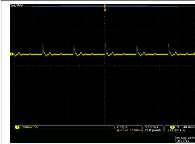
Figure 3-25. Typical Ripple Voltage of  $V_{OUT} = 20\text{ V}$
