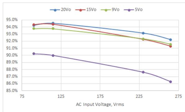
Figure 3-5. Efficiency of 50%-load vs. Input Voltage
