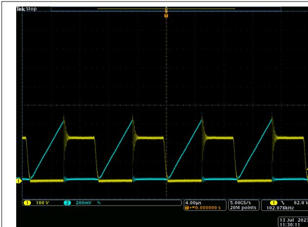
Figure 3-9. Vin = 90Vac, Vout = 20 V
