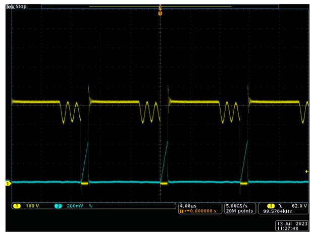
Figure 3-20. Vin = 265Vac, Vout = 9 V
