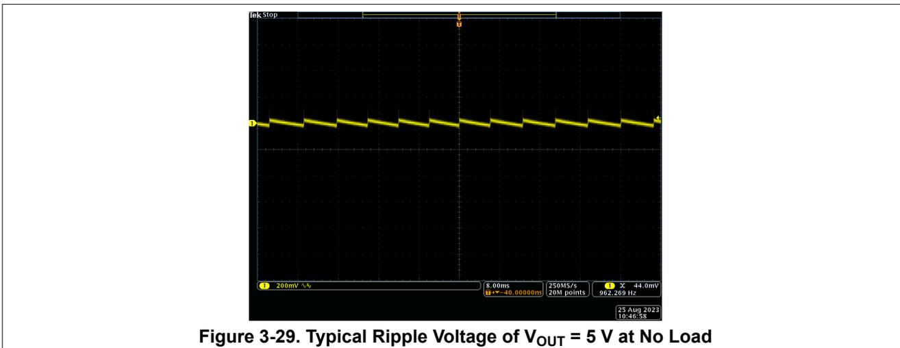
Figure 3-29. Typical Ripple Voltage of  $V_{OUT} = 5\text{ V}$  at No Load
