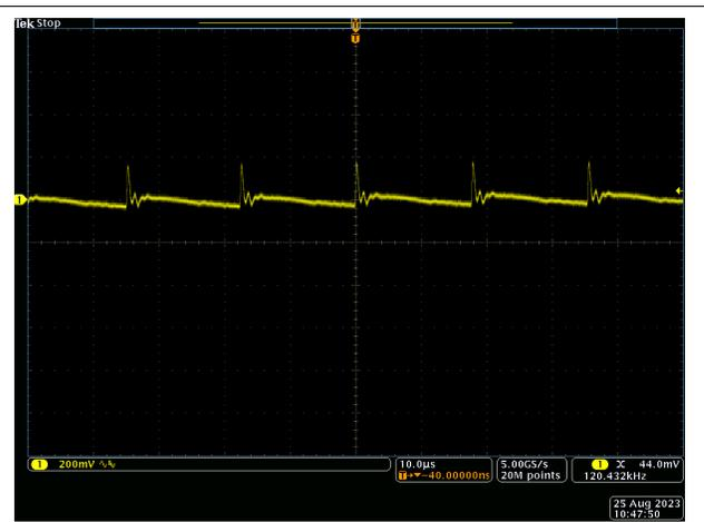
Figure 3-28. Typical Ripple Voltage of  $V_{OUT} = 5\text{ V}$
