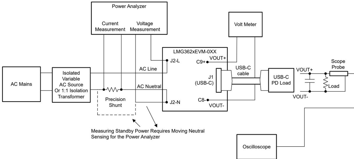
**Figure 3-1. LMG3624EVM-081 Test Setup Diagram**
