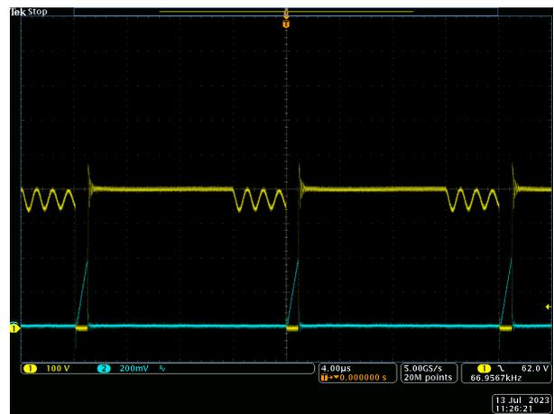
Figure 3-24. Vin = 265Vac, Vout = 5 V
