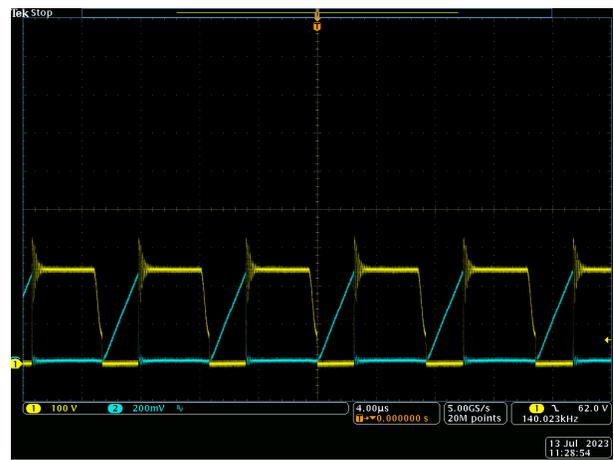
Figure 3-14. Vin = 115Vac, Vout = 15 V
