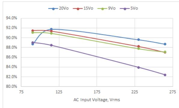
Figure 3-3. Efficiency of 10%-Load vs. Input Voltage
