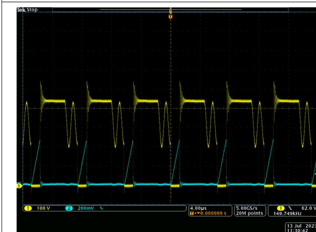
Figure 3-11. Vin = 230Vac, Vout = 20 V
