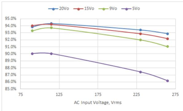
Figure 3-2. 4pt-Average Efficiency vs. Input Voltage
