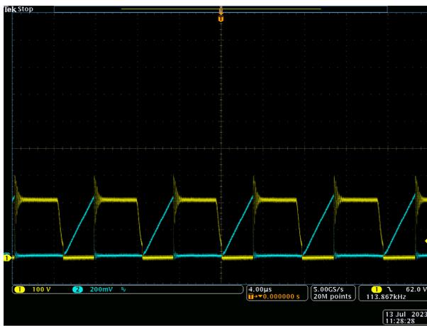
Figure 3-13. Vin = 90Vac, Vout = 15 V
