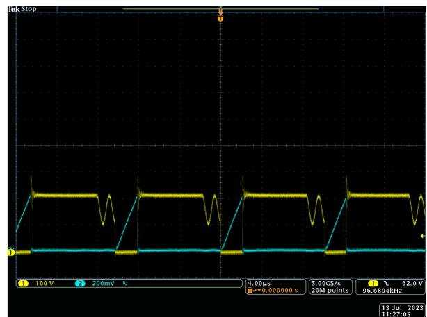
Figure 3-18. Vin = 115Vac, Vout = 9 V
