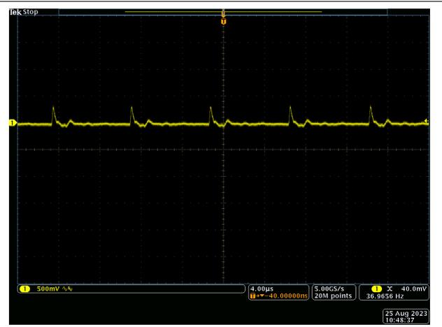
Figure 3-26. Typical Ripple Voltage of  $V_{OUT} = 15\text{ V}$
