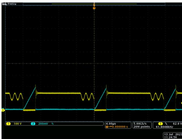
Figure 3-21. Vin = 90Vac, Vout = 5 V
