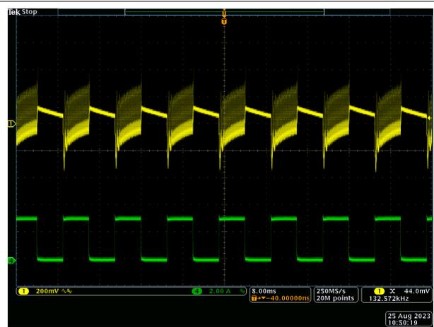
Figure 3-31. Transient Response at  $V_{OUT} = 15$  V
