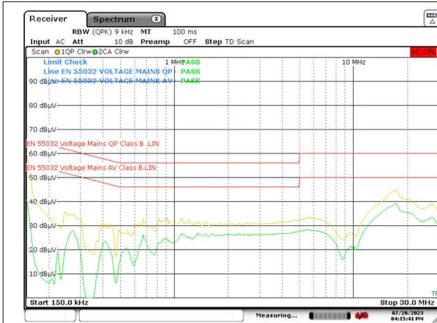
**Figure 3-34. VIN = 115 V<sub>RMS</sub>, VOUT = 20 V, Load = 3.25 A (Output Not Grounded to LISN Ground)**
