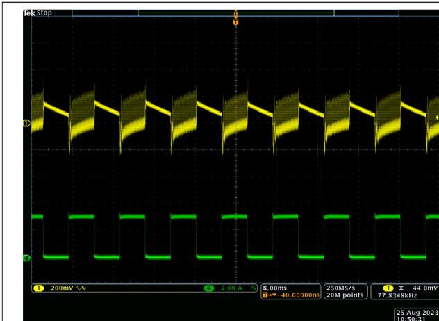
Figure 3-32. Transient Response at  $V_{OUT} = 9$  V
