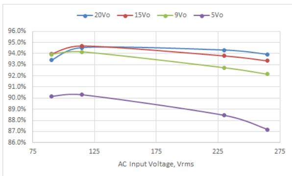
Figure 3-4. Full-load Efficiency vs. Input Voltage
