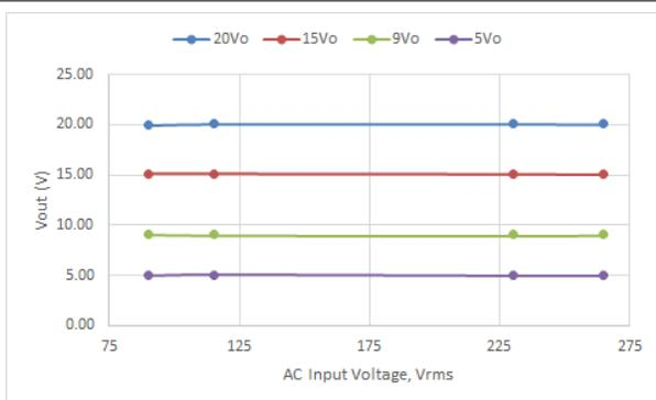
Figure 3-6.  $V_{OUT}$  at Full-Load vs Input Voltage
