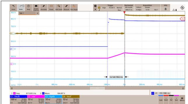
**Figure 3-8. Start-up Waveforms at 265Vac and No Load**
