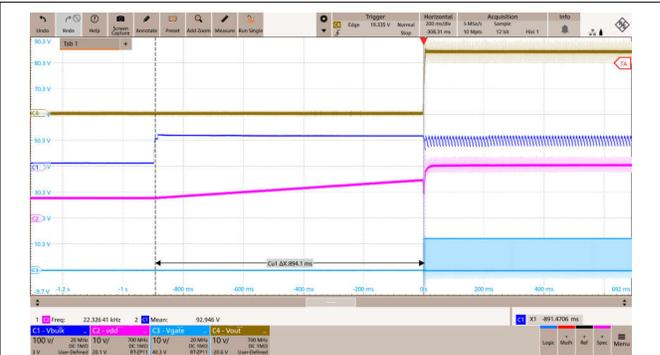
**Figure 3-3. Start-up Waveforms at 85Vac and Full Load**
