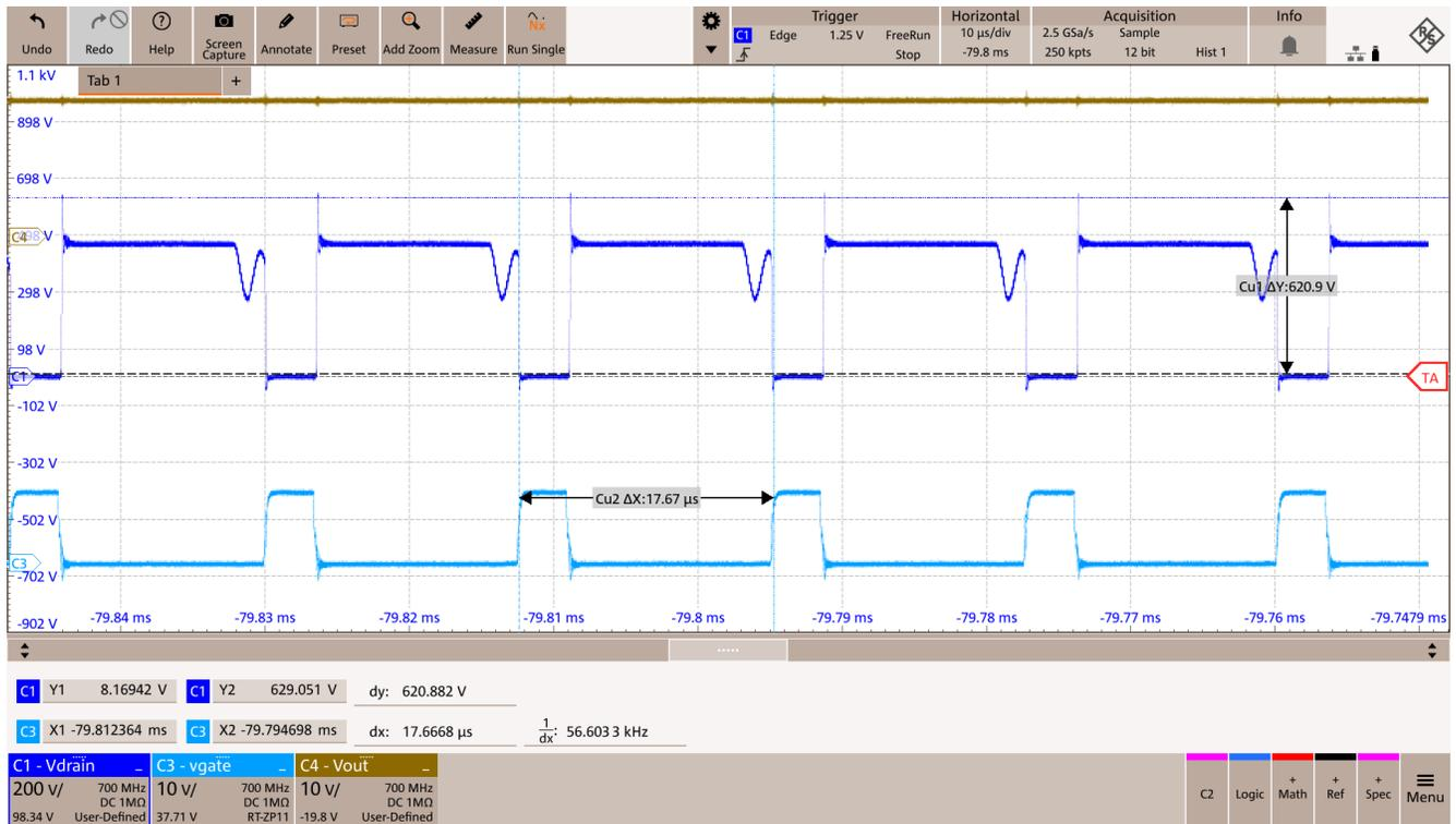
Figure 3-17. Steady State Waveform at 85Vac
