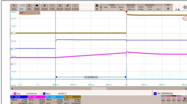
**Figure 3-2. Start-up Waveforms at 85Vac and No Load**
