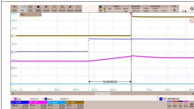
**Figure 3-4. Start-up Waveforms at 115Vac and No Load**
