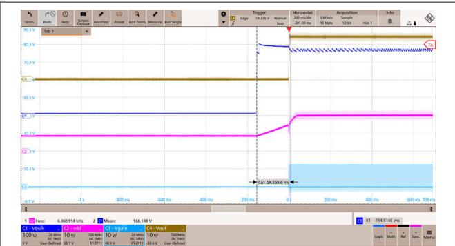
**Figure 3-9. Start-up Waveforms at 265Vac and Full Load**
