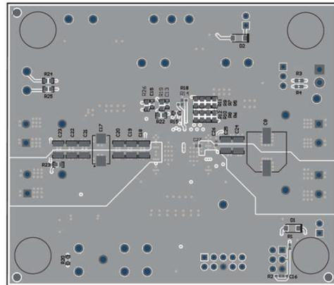
Figure 5-3. TPSM8S6C24SEVM-1PH Bottom Side Component View (Bottom View)
