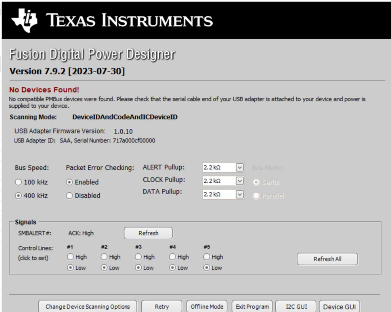
Figure 3-1. Select Device Scanning Mode
