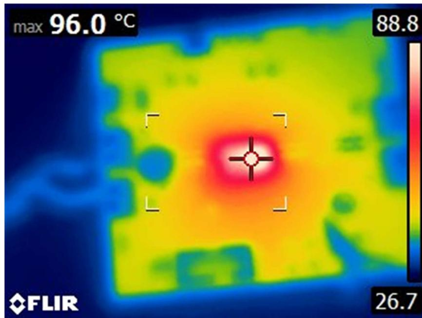
$V_{IN} = 12\text{ V}$ ,  $V_{OUT} = 1.2\text{ V}$ ,  $I_{OUT} = 35\text{ A}$ , Airflow = 200 LFM, 10-min soak
