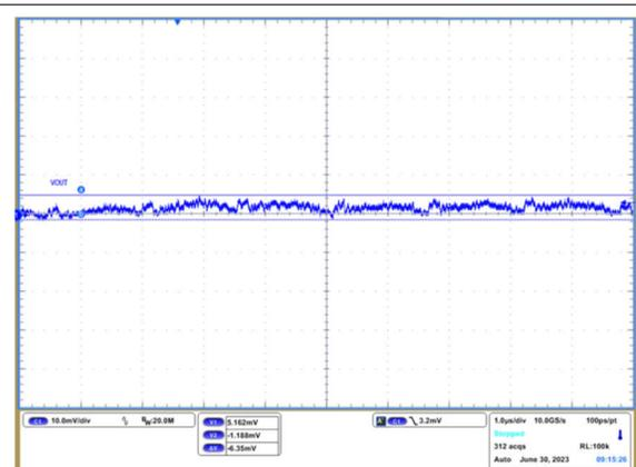
Figure 4-7. VOUT Output Ripple, 35-A Load
