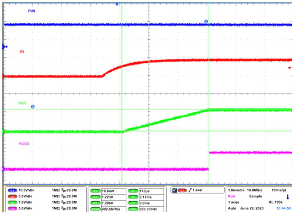
Figure 4-8. VOUT Start-Up From Enable, 35-A Load
