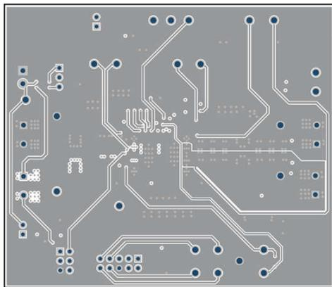
Figure 5-6. TPSM8S6C24SEVM-1PH Internal Layer 2 (Top View)
