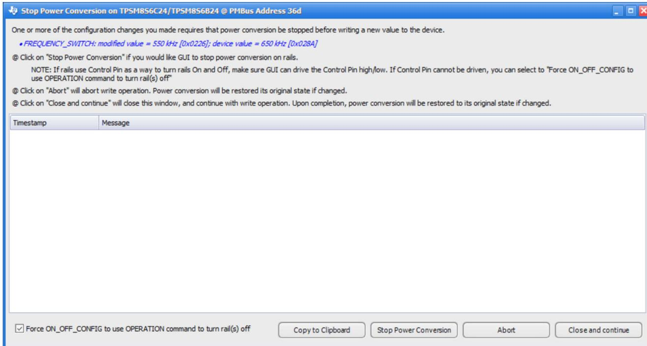
**Figure 3-4. Pop-Up When Trying to Change FREQUENCY\_SWITCH With Conversion Enabled**
