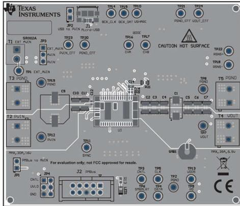
Figure 5-2. TPSM8S6C24SEVM-1PH Top Side Component View (Top View)
