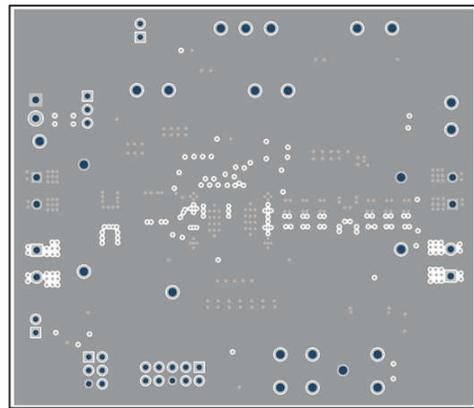
Figure 5-7. TPSM8S6C24SEVM-1PH Internal Layer 3 (Top View)
