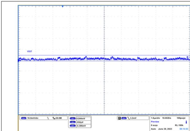
Figure 4-6. VOUT Output Ripple, No Load
