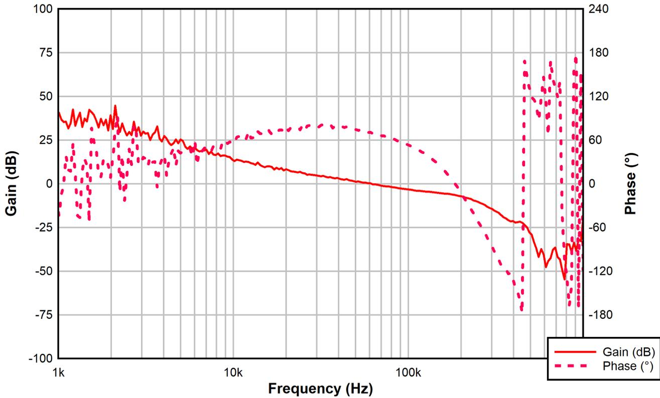
Figure 4-5. VOUT Bode Plot, 12Vin, 1.2-V, 35-A Load
