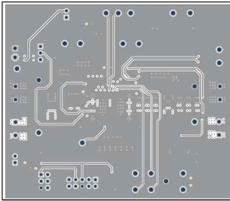
**Figure 5-8. TPMS8S6C24SEVM-1PH Internal Layer 4 (Top View)**
