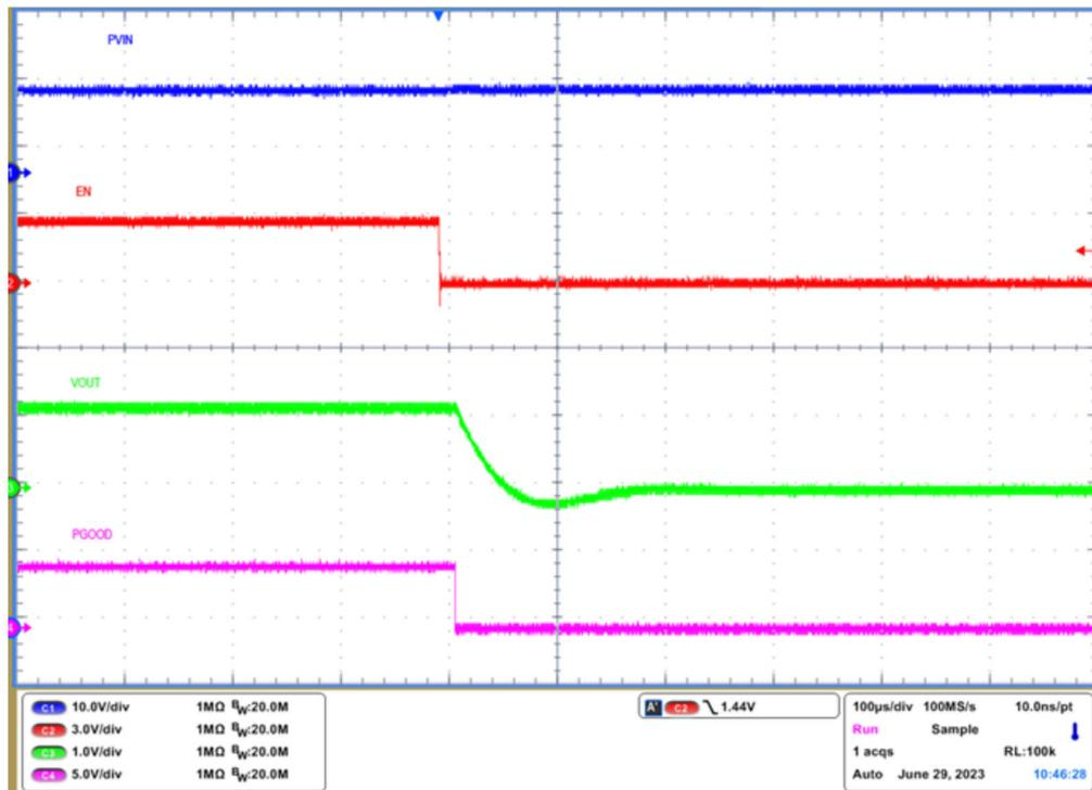
Figure 4-9. VOUT Shutdown From Enable, 35-A Load
