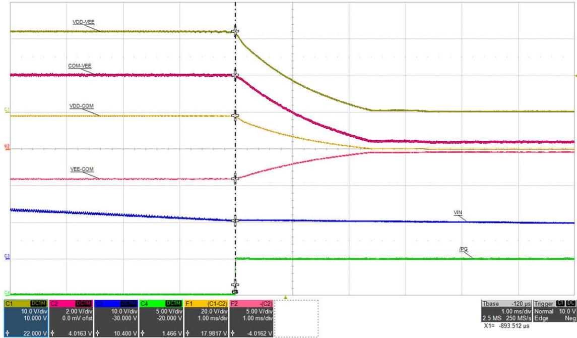
Figure 5-24. Shutdown by VIN Removal:  $V_{IN\text{OFF}}=10.4\text{ V}$ ,  $I_{VDD-VEE}=68\text{ mA}$  (top: VDD-VEE, 10 V/div, mid-1: COM-VEE, 2 V/div, mid-2: VDD-COM, 20 V/div, mid-3: VEE-COM, 5 V/div, mid-4: VIN, 10 V/div, bot: /PG, 5 V/div), time=1 ms/div
