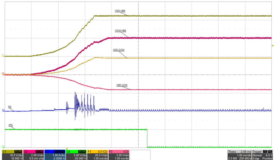
Figure 5-9. Inrush Current 1: VIN=15 V, I<sub>VDD-VEE</sub>=68 mA, (top: VDD-VEE, 10 V/div, mid-1: COM-VEE, 2 V/div, mid-2: VDD-COM, 20 V/div, mid-3: VEE-COM, 5 V/div, mid-4: IIN, 1 A/div, bot: /PG, 5 V/div), time = 1 ms/div
