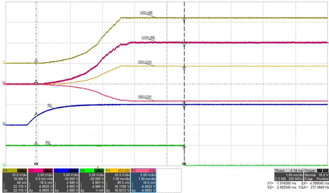
Figure 5-7. Start-up 3: VIN=15 V, I<sub>VDD-VEE</sub>=68 mA, (top: VDD-VEE, 10 V/div, mid-1: COM-VEE, 2 V/div, mid-2: VDD-COM, 20 V/div, mid-3: VEE-COM, 5 V/div, mid-4: EN, 5 V/div, bot: /PG, 5 V/div), time = 1 ms/div, EN to /PG delay = 4.6 ms
