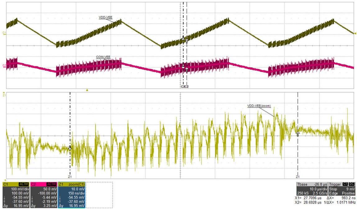
Figure 5-16. AC Ripple 5: VIN=15 V, IVDD=68 mA, FBURST=1 MHz, (top: VDD-VEE, 100 mV/div, bot: COM-VEE, 50 mV/div, Zoom: VDD-VEE, 10 mV/div), time =10  $\mu$ s/div, time\_zoom=150 ns/div
