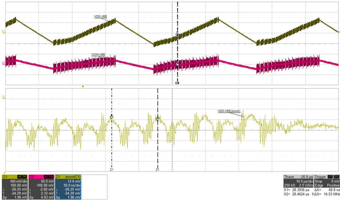
Figure 5-15. AC Ripple 4: VIN=15 V, IVDD=68 mA, FSW(PRI)=14.53 MHz, (top: VDD-VEE, 100 mV/div, bot: COM-VEE, 50 mV/div, Zoom: VDD-VEE, 13.6 mV/div), time =10 μs/div, time\_zoom=50 ns/div
