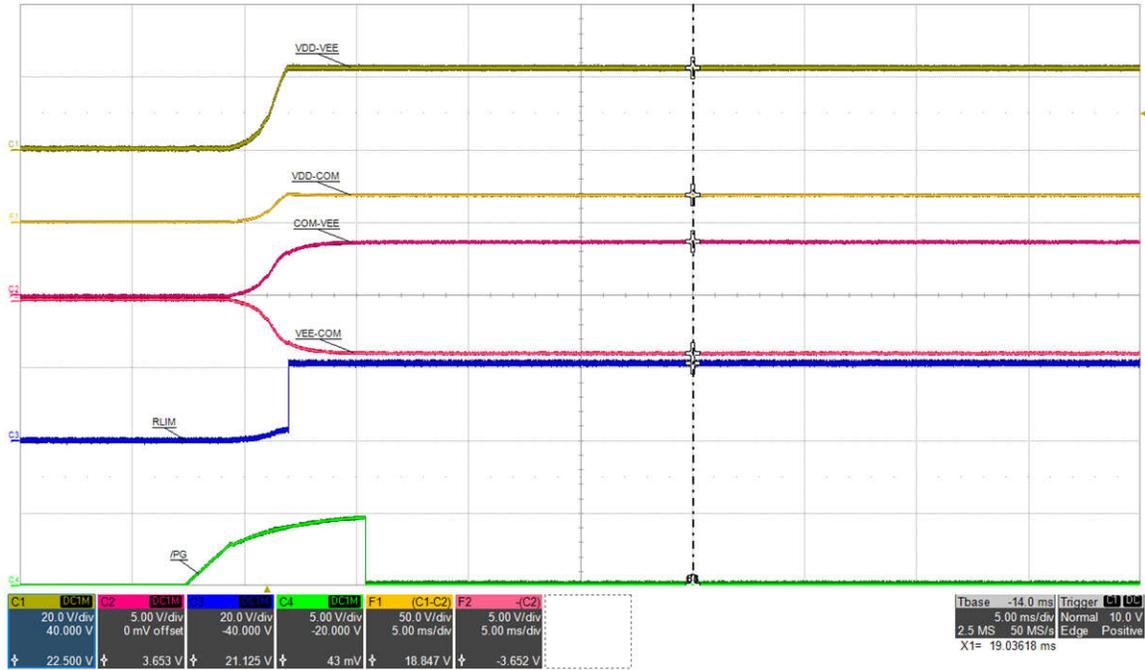
Figure 5-23. Normal Start (close to COM-VEE UVLO): VIN=15 V, PVDD=573 mW, PVEE=404 mW, (top: VDD-VEE, 20 V/div, mid-1: VDD-COM, 50 V/div, mid-2: COM-VEE, 5 V/div, mid-3: VEE-COM, 5 V/div, mid-4: RLIM, 20 V/div, bot: /PG, 5 V/div), time = 5 ms/div
