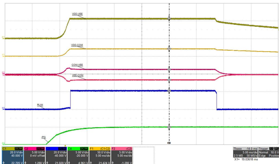
Figure 5-21. Output UVLO: Vin=15 V, PVDD=0 mW, PVEE=50 mW, (top: VDD-VEE, 20 V/div, mid-1: VDD-COM, 50 V/div, mid-2: COM-VEE, 5 V/div, mid-3: VEE-COM, 5 V/div, mid-4: RLIM, 20 V/div, bot: /PG, 5 V/div), time = 5 ms/div
