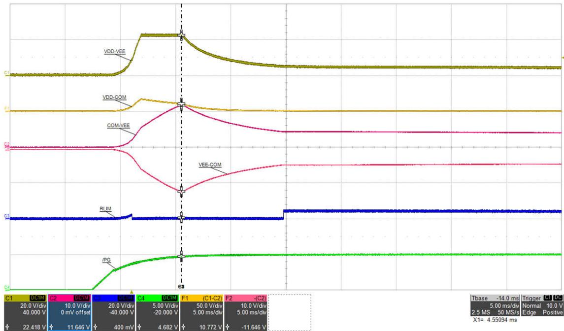
Figure 5-22. COM-VEE OVP: VIN=15 V, PVDD=188 mW, PVEE=0 mW, (top: VDD-VEE, 20 V/div, mid-1: VDD-COM, 50 V/div, mid-2: COM-VEE, 10 V/div, mid-3: VEE-COM, 10 V/div, mid-4: RLIM, 20 V/div, bot: /PG, 5 V/div), time = 5 ms/div
