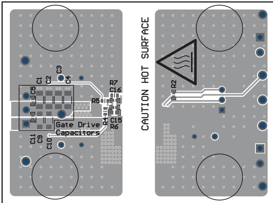
Figure 6-7. UCC14341EVM-069, PCB Bottom Layer, Assembly (mirrored view)
