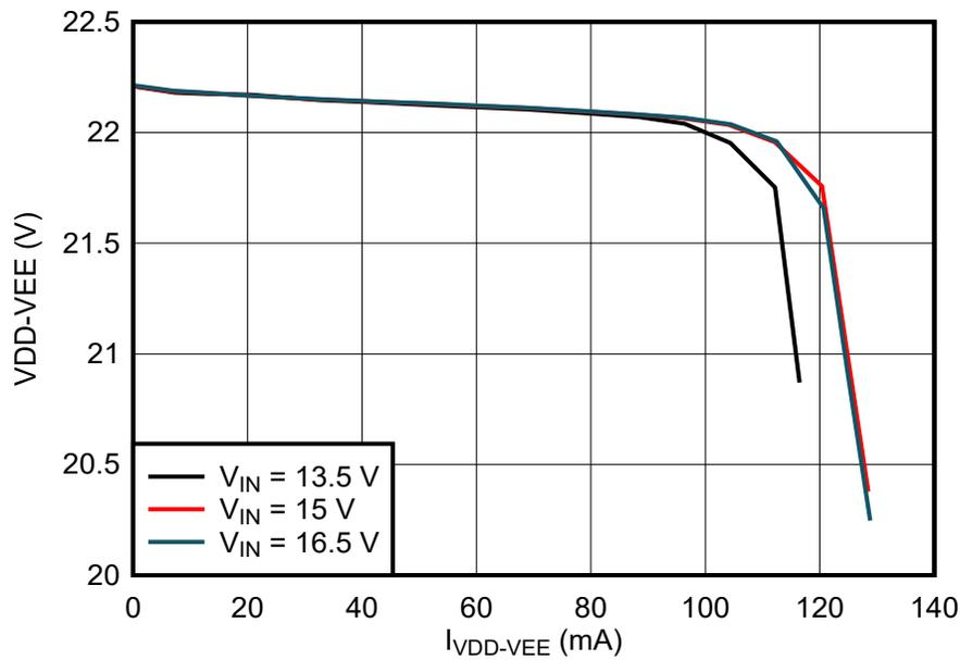
Figure 5-3. Regulation vs Current, VDD-VEE Loading Only
