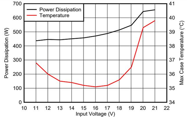
**Figure 5-30. Power Dissipation and Case Temperature vs Input Voltage,  $T_A=23^\circ\text{C}$ ,  $0\text{ W}$**
