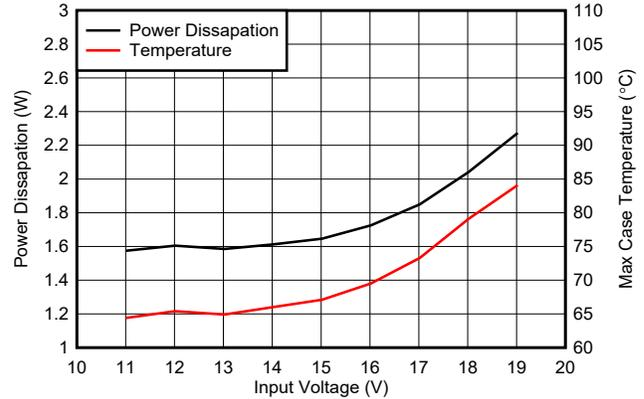
**Figure 5-28. Power Dissipation and Case Temperature vs Input Voltage,  $T_A=23^\circ\text{C}$ ,  $1.51\text{ W}$**
