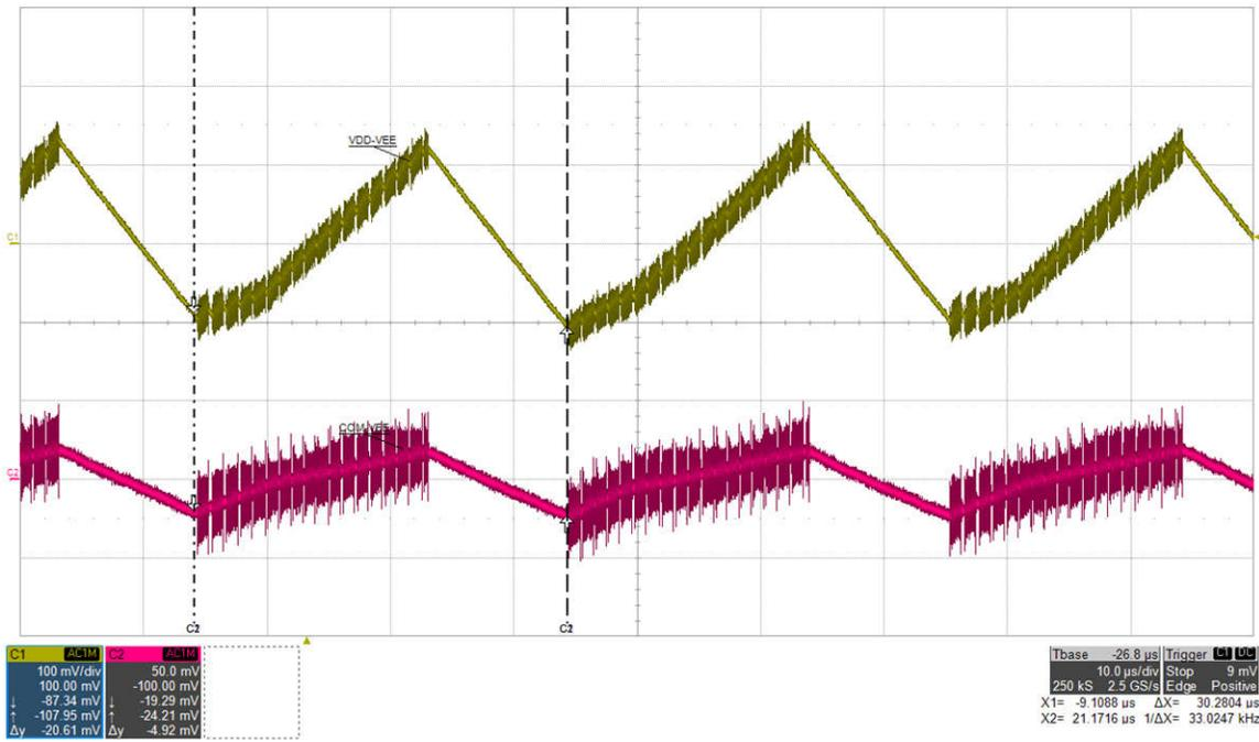
Figure 5-14. AC Ripple 3: VIN=15 V, IVDD=68 mA, IVEE=0 mA, FMOD=33 kHz, (top: VDD-VEE, 100 mV/div, bot: COM-VEE, 50 mV/div), time =10 μs/div
