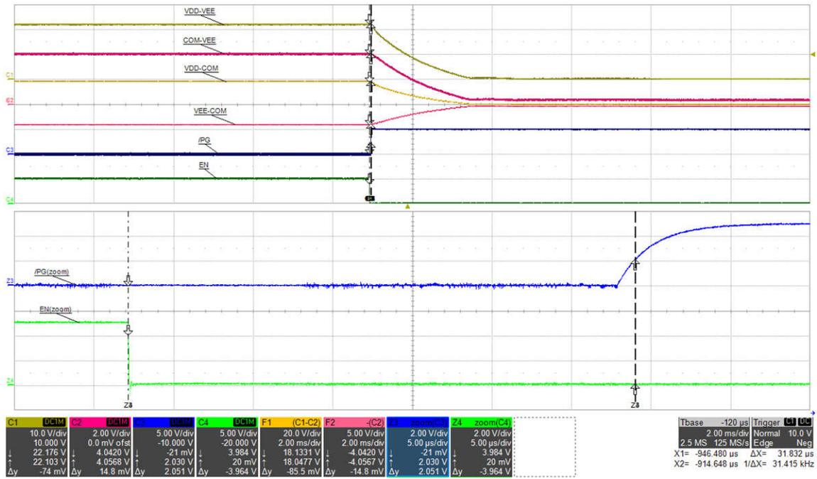
Figure 5-26. Shutdown by EN Low (zoom): VIN=15 V, I<sub>VDD-VEE</sub>=68 mA (top: VDD-VEE, 10 V/div, mid-1: COM-VEE, 2 V/div, mid-2: VDD-COM, 20 V/div, mid-3: VEE-COM, 5 V/div, mid-4: /PG, 5 V/div, bot: EN, 5 V/div, top\_zoom: /PG, 2 V/div, bot\_zoom: EN, 2 V/div), time=2 ms/div, time\_zoom=5 μs/div
