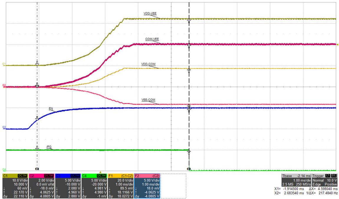
Figure 5-17. ENA to /PG Delay, 4.6 ms, VIN=15 V, IVDD-VEE=68 mA, (top: VDD-VEE, 10 V/div, mid-1: COM-VEE, 2 V/div, mid-2: VDD-COM, 20 V/div, mid-3: VEE-COM, 5 V/div, mid-4: EN, 5 V/div, bot: /PG, 5 V/div), time = 1 ms/div
