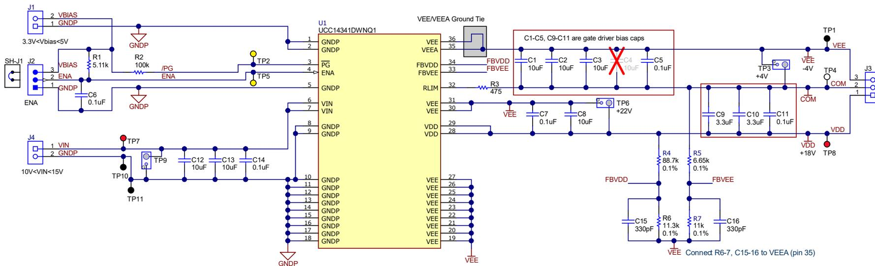
Figure 3-1. UCC14341EVM-069 Schematic Diagram
