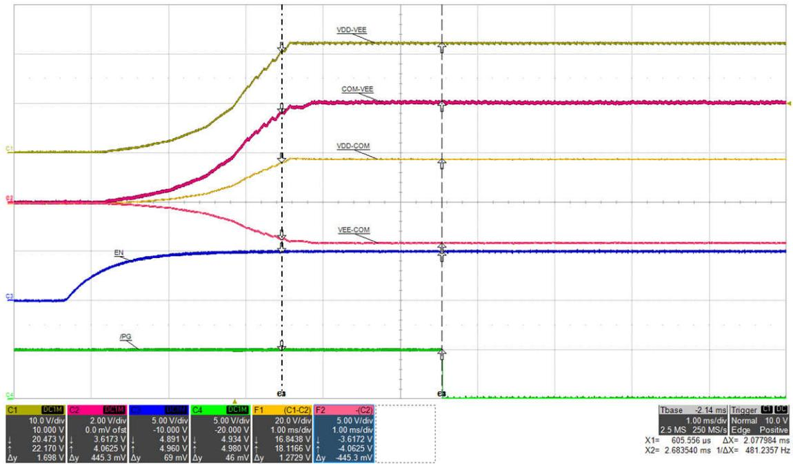
Figure 5-8. Start-up 4: VIN=15 V, I<sub>VDD-VEE</sub>=68 mA, (top: VDD-VEE, 10 V/div, mid-1: COM-VEE, 2 V/div, mid-2: VDD-COM, 20 V/div, mid-3: VEE-COM, 5 V/div, mid-4: EN, 5 V/div, bot: /PG, 5 V/div), time = 1 ms/div, Reg to /PG delay = 2.07 ms
