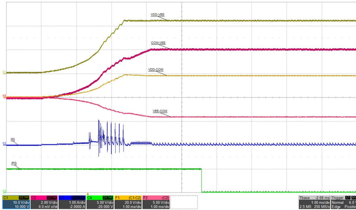
Figure 5-10. Inrush Current 2: VIN=15 V, I<sub>VDD-VEE</sub>=0 mA, (top: VDD-VEE, 10 V/div, mid-1: COM-VEE, 2 V/div, mid-2: VDD-COM, 20 V/div, mid-3: VEE-COM, 5 V/div, mid-4: IIN, 1 A/div, bot: /PG, 5 V/div), time =1 ms/div
