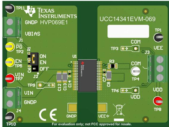
Figure 6-1. UCC14341EVM-069, Fully Assembled 3D Top View
