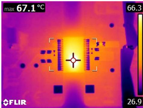
$V_{IN} = 15\text{ V}$       $V_{DD} = 22.2\text{ V}$       $I_{VDD} = 68.3\text{ mA}$
