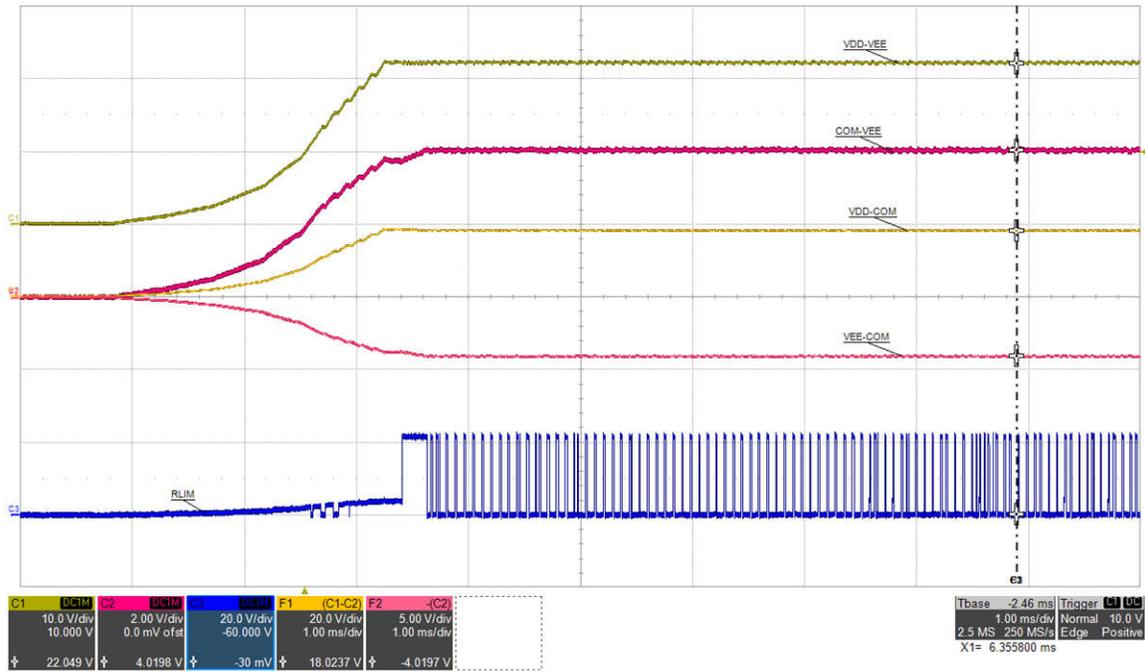
Figure 5-19. RLIM 2:  $V_{IN}=15\text{ V}$ ,  $I_{VDD-VEE}=68\text{ mA}$ , (top: VDD-VEE, 10 V/div, mid-1: COM-VEE, 2 V/div, mid-2: VDD-COM, 20 V/div, mid-3: VEE-COM, 5 V/div, bot: RLIM, 20 V/div), time = 1 ms/div
