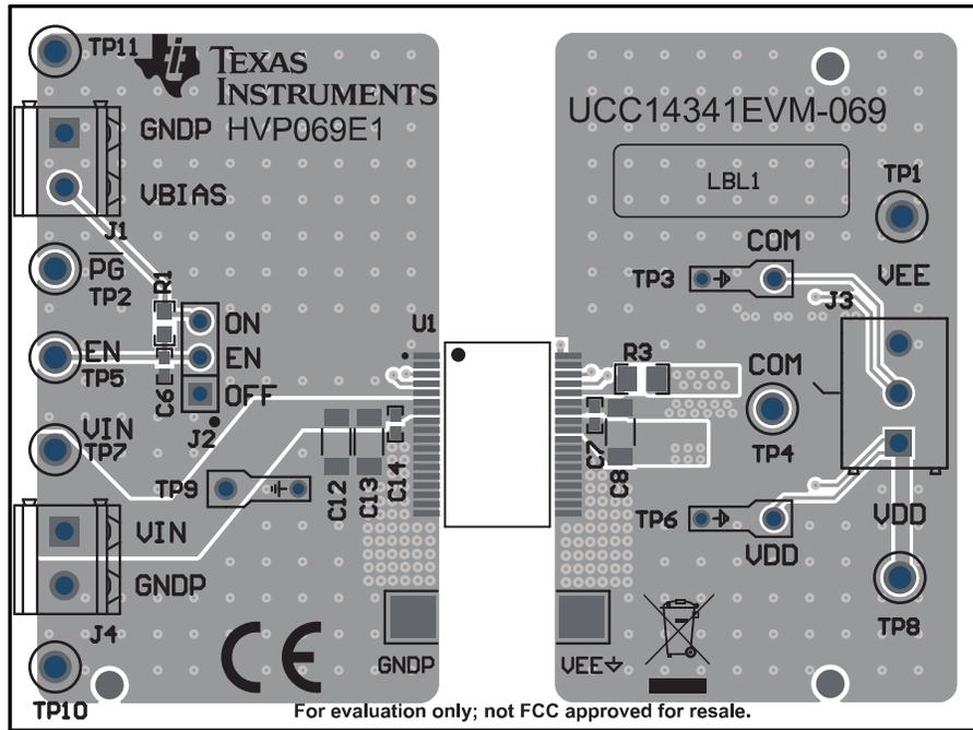
Figure 6-4. UCC14341EVM-069, PCB Top Layer, Assembly
