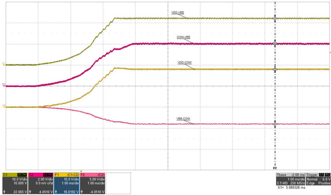
Figure 5-6. Start-up 2: VIN=15 V, I<sub>VDD-VEE</sub>=68 mA, (top: VDD-VEE, 10 V/div, mid-1: COM-VEE, 2 V/div, mid-2: VDD-COM, 10 V/div, bot: VEE-COM, 5 V/div), time = 1 ms/div
