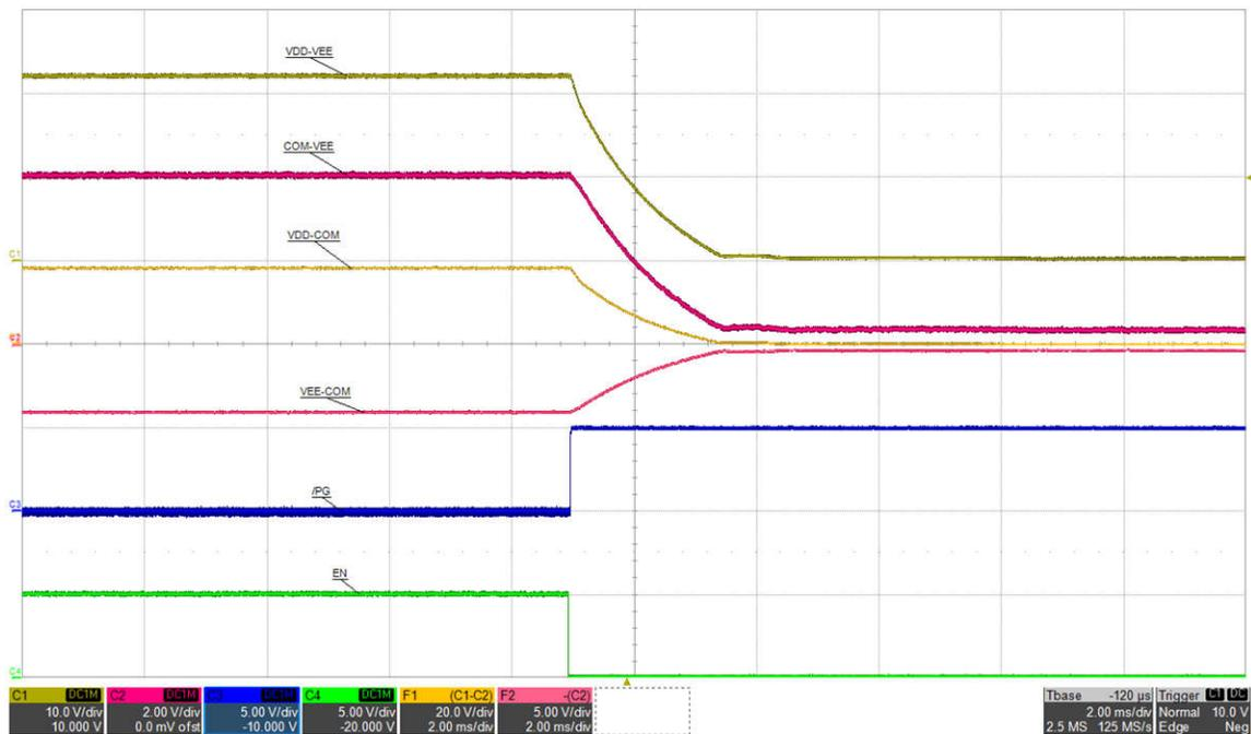
Figure 5-25. Shutdown by EN Low:  $V_{IN}=15\text{ V}$ ,  $I_{VDD-VEE}=68\text{ mA}$  (top: VDD-VEE, 10 V/div, mid-1: COM-VEE, 2 V/div, mid-2: VDD-COM, 20 V/div, mid-3: VEE-COM, 5 V/div, mid-4: /PG, 5 V/div, bot: EN, 5 V/div), time=2 ms/div
