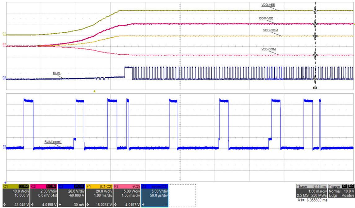
Figure 5-20. RLIM 3: VIN=15 V, I<sub>VDD-VEE</sub>=68 mA, (top: VDD-VEE, 10 V/div, mid-1: COM-VEE, 2 V/div, mid-2: VDD-COM, 20 V/div, mid-3: VEE-COM, 5 V/div, bot: RLIM, 20 V/div, Zoom: RLIM, 5 V/div), time = 1 ms/div, time\_zoom = 50 μs/div
