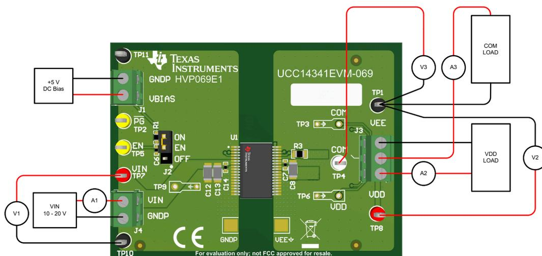
Figure 4-1. Typical Efficiency Measurement Setup
