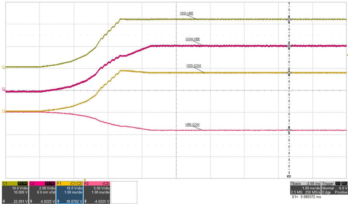
Figure 5-5. Start-up 1:  $V_{IN}=15$  V,  $I_{VDD-VEE}=0$  mA, (top: VDD-VEE, 10 V/div, mid-1: COM-VEE, 2 V/div, mid-2: VDD-COM, 10 V/div, bot: VEE-COM, 5 V/div), time = 1 ms/div
