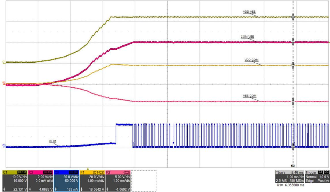
Figure 5-18. RLIM 1:  $V_{IN}=15\text{ V}$ ,  $I_{VDD-VEE}=0\text{ mA}$ , (top: VDD-VEE, 10 V/div, mid-1: COM-VEE, 2 V/div, mid-2: VDD-COM, 20 V/div, mid-3: VEE-COM, 5 V/div, bot: RLIM, 20 V/div), time = 1 ms/div
