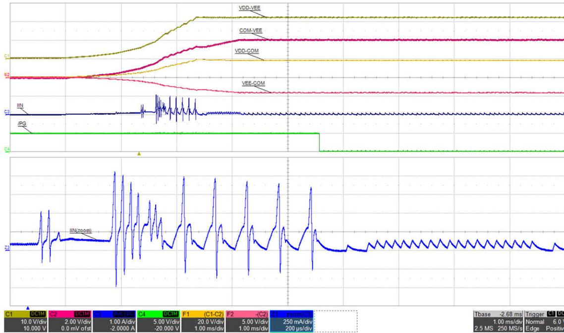
Figure 5-11. Inrush Current 3: VIN=15 V, I<sub>VDD-VEE</sub>=0 mA, (top: VDD-VEE, 10 V/div, mid-1: COM-VEE, 2 V/div, mid-2: VDD-COM, 20 V/div, mid-3: VEE-COM, 5 V/div, mid-4: IIN, 1 A/div, bot: /PG, 5 V/div, zoom: 250 mA/div), time =1 ms/div, time\_zoom=200 µs/div
