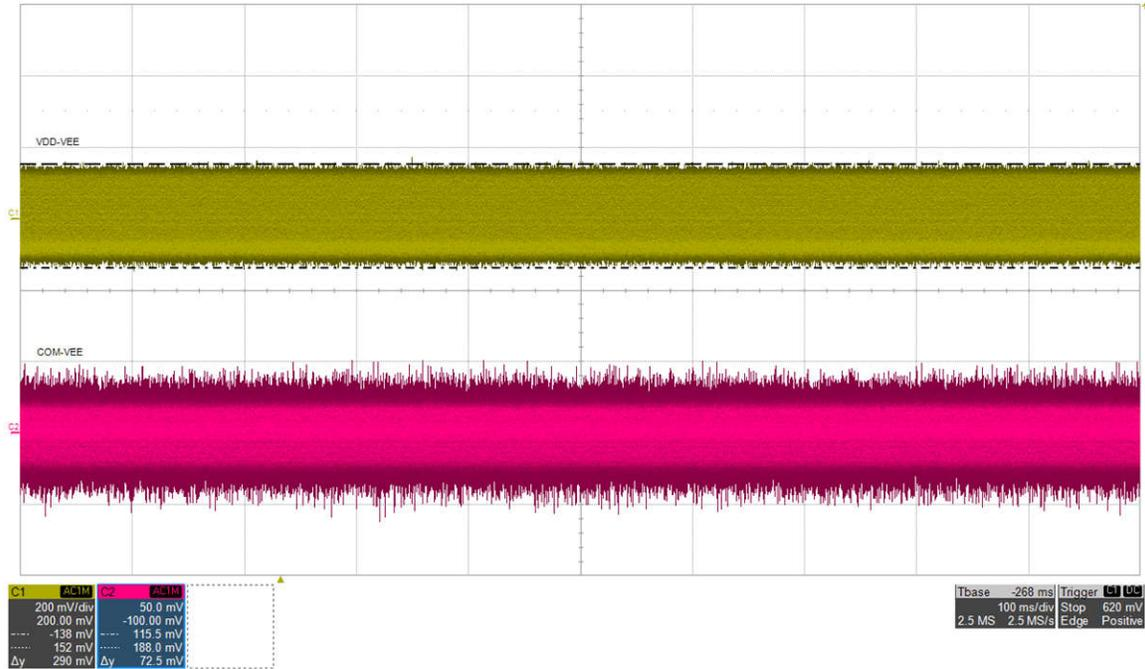
Figure 5-12. AC Ripple 1:  $V_{DDAC}=290$  mV,  $V_{EEAC}=90$  mV,  $I_{VDD}=68$  mA,  $I_{VEE}=0$  mA (top: VDD-VEE, 200 mV/div, bot: COM-VEE, 50 mV/div), time = 100 ms/div
