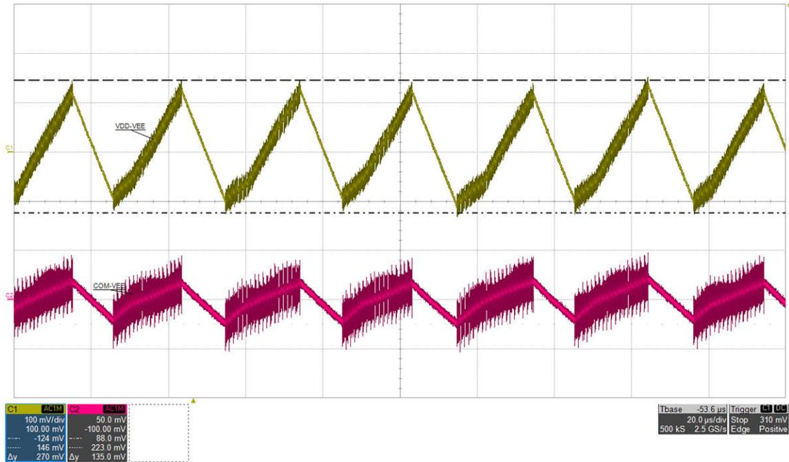
Figure 5-13. AC Ripple 2:  $V_{IN}=15$  V,  $I_{VDD}=68$  mA,  $I_{VEE}=0$  mA, (top: VDD-VEE, 100 mV/div, bot: COM-VEE, 50 mV/div), time = 20 μs/div
