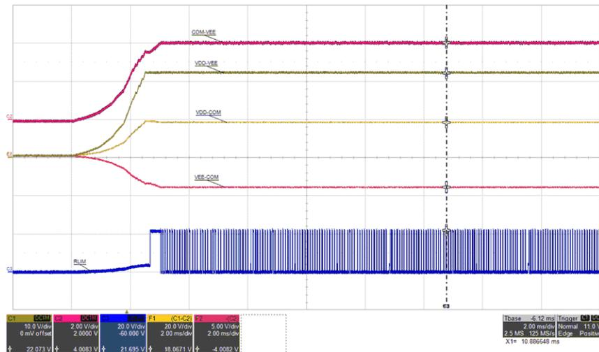
Figure 5-19. RLIM:  $V_{IN}=12$  V,  $I_{VDD-VEE}=0$  mA, (top: COM-VEE, 2 V/div, mid-1: VDD-VEE, 10 V/div, mid-2: VDD-COM, 20 V/div, mid-3: VEE-COM, 5 V/div, bot: RLIM, 20 V/div), time = 2 ms/div
