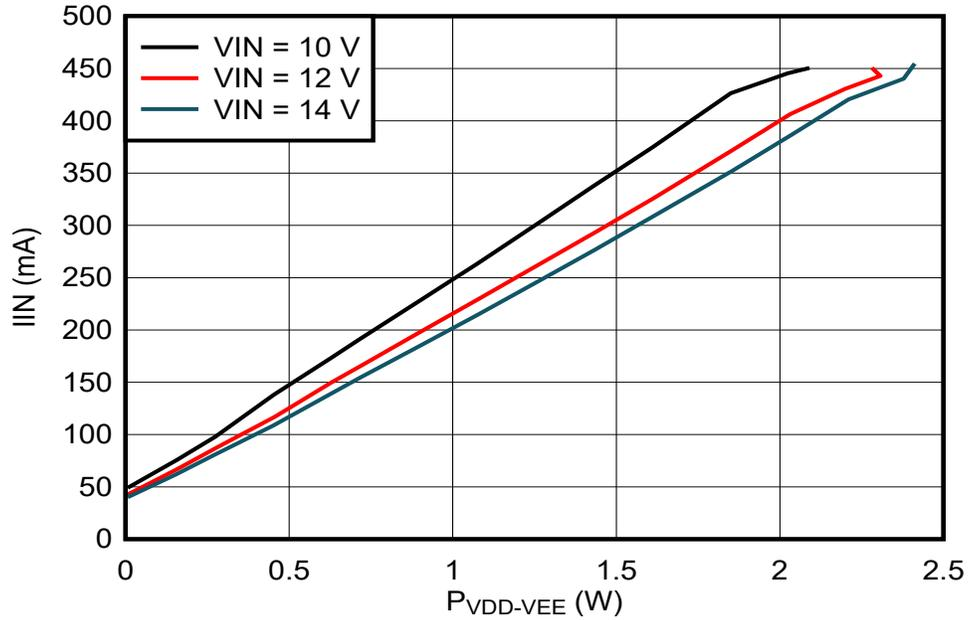
Figure 5-4. Input Current vs Power, VDD-VEE Loading Only
