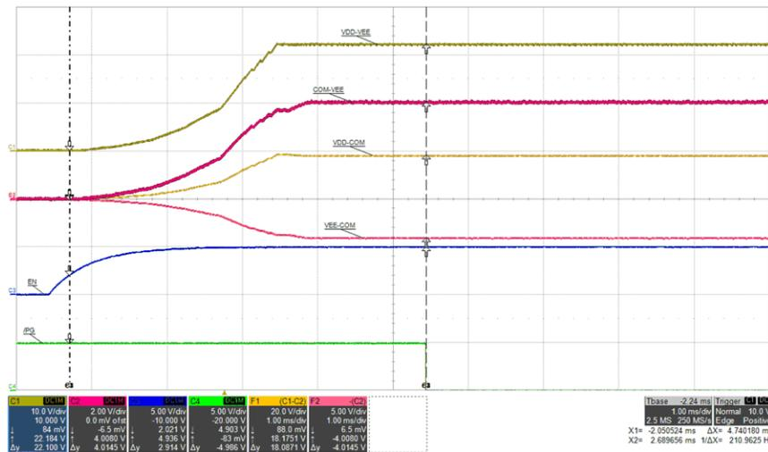
Figure 5-7. Start-up 3:  $V_{IN}=12\text{ V}$ ,  $I_{VDD-VEE}=68\text{ mA}$ , (top: VDD-VEE, 10 V/div, mid-1: COM-VEE, 2 V/div, mid-2: VDD-COM, 20 V/div, mid-3: VEE-COM, 5 V/div, mid-4: EN, 5 V/div, bot: /PG, 5 V/div), time = 1 ms/div
