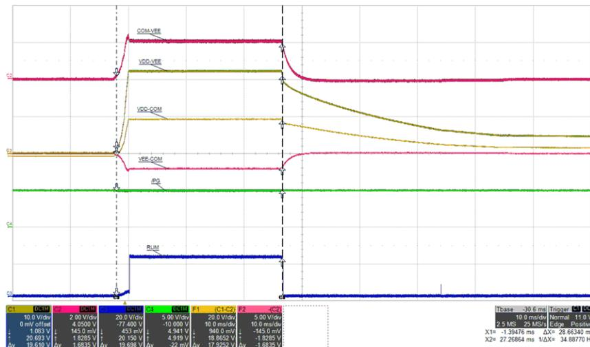
Figure 5-22. Output UVLO, PVDD=0 mW, PVEE=313 mW, (top: COM-VEE, 2 V/div, mid1: VDD-VEE, 10 V/div, mid2: VDD-COM, 20 V/div, mid3: VEE-COM, 5 V/div, bot: RLIM, 20 V/div), time = 10 ms/div
