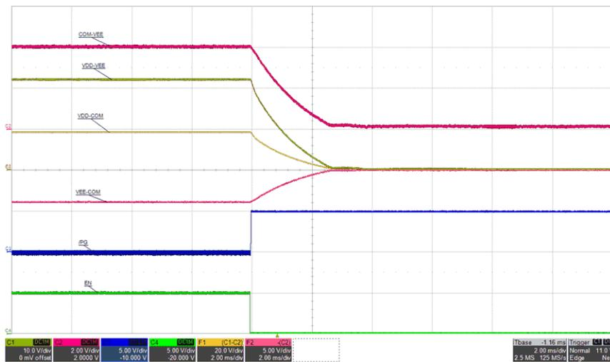
Figure 5-26. Shutdown by EN Low:  $V_{IN}=12\text{ V}$ ,  $I_{VDD-VEE}=68\text{ mA}$ , (top: COM-VEE, 2 V/div, mid-1: VDD-VEE, 10 V/div, mid-2: VDD-COM, 20 V/div, mid-3: VEE-COM, 5 V/div, mid-4: /PG, 5 V/div, bot: ENA, 5 V/div), time = 2 ms/div
