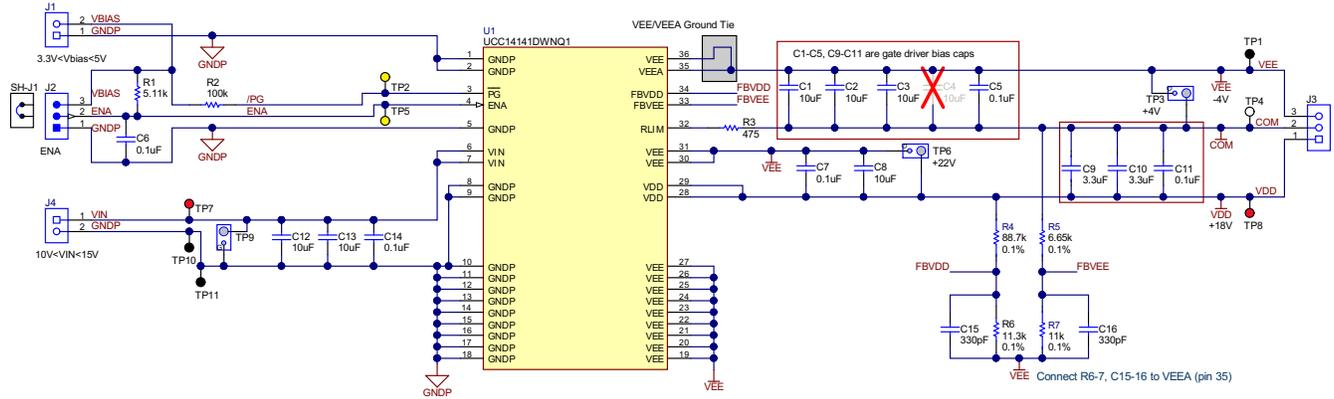
Figure 3-1. UCC14141EVM-068 Schematic Diagram
