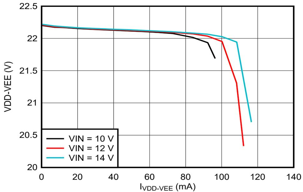
Figure 5-3. Regulation vs Current, VDD-VEE Loading Only
