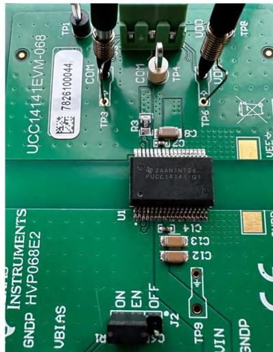
**Figure 4-2. UCC14141EVM-068, PCB Scope Probe Test Points**
