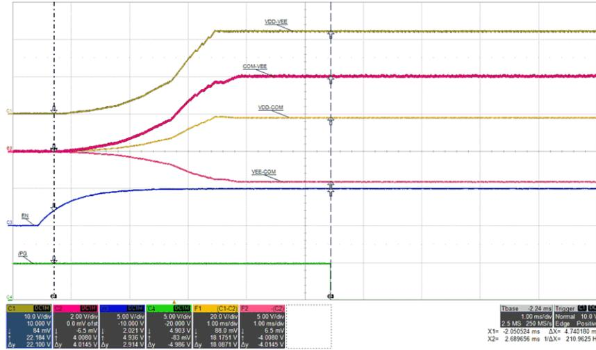
Figure 5-18. ENA to /PG Delay, 4.7 ms,  $I_{VDD-VEE}=68$  mA, (top: VDD-VEE, 10 V/div, mid1: COM-VEE, 2 V/div, mid2: VDD-COM, 20 V/div, mid3: VEE-COM, 5 V/div, mid4: EN, 5 V/div, bot: /PG, 5 V/div), time = 1 ms/div
