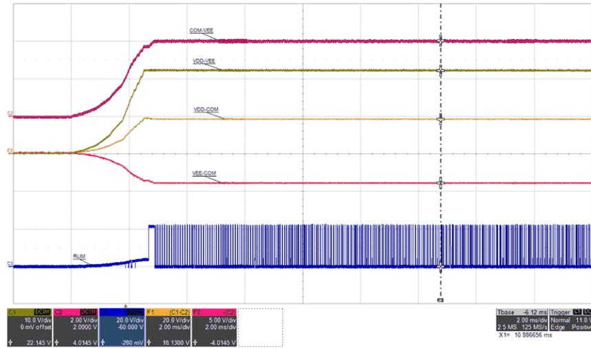
Figure 5-20. RLIM:  $V_{IN}=12\text{ V}$ ,  $I_{VDD-VEE}=68\text{ mA}$ , (top: COM-VEE, 2 V/div, mid-1: VDD-VEE, 10 V/div, mid-2: VDD-COM, 20 V/div, mid-3: VEE-COM, 5 V/div, bot: RLIM, 20 V/div), time = 2 ms/div
