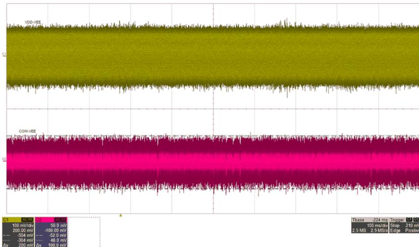
Figure 5-13.  $V_{DDAC}=240\text{ mV}$ ,  $V_{EEAC}=100\text{ mV}$ ,  $I_{VDD}=68\text{ mA}$ ,  $I_{VEE}=30\text{ mA}$  (top: VDD-VEE, 100 mV/div, bot: COM-VEE, 50 mV/div), time = 100 ms/div
