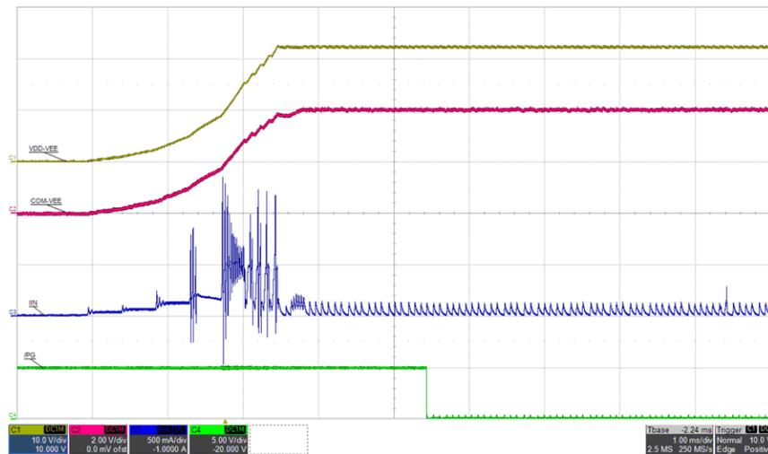
**Figure 5-11. Inrush Current:  $V_{IN}=12\text{ V}$ ,  $I_{VDD-VEE}=0\text{ mA}$ , (top: VDD-VEE, 10 V/div, mid-1: COM-VEE, 2 V/div, mid-2: IIN, 0.5 A/div, bot: /PG, 5 V/div), time = 1 ms/div**
