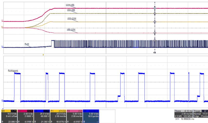
Figure 5-21. RLIM:  $V_{IN}=12\text{ V}$ ,  $I_{VDD-VEE}=68\text{ mA}$ , (top: COM-VEE, 2 V/div, mid-1: VDD-VEE, 10 V/div, mid-2: VDD-COM, 20 V/div, mid-3: VEE-COM, 5 V/div, bot: RLIM, 20 V/div, Zoom: RLIM, 5 V/div), time = 10 ms/div, time\_zoom = 50  $\mu$ s/div
