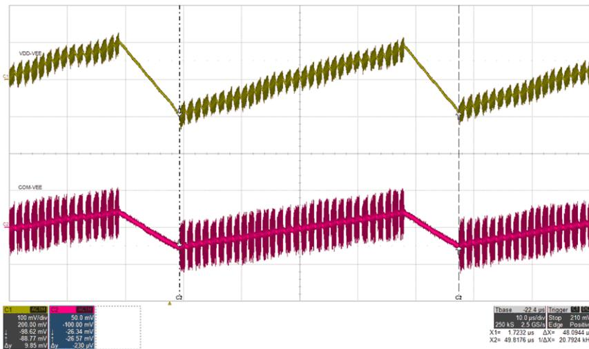
Figure 5-15. AC Ripple: VIN=12 V, IVDD=68 mA, IVEE=30 mA, FMOD=20.8 kHz (top: VDD-VEE, 100 mV/div, bot: COM-VEE, 50 mV/div), time = 10 μs/div
