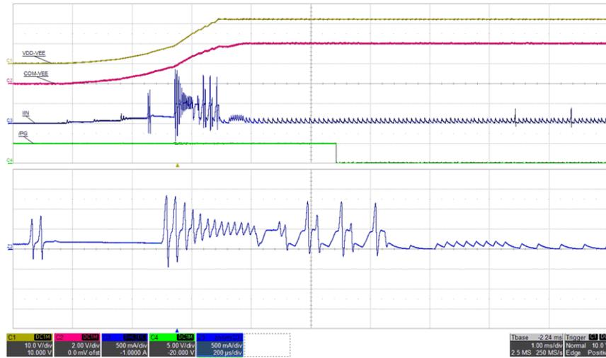
**Figure 5-10. Inrush Current:  $V_{IN}=12\text{ V}$ ,  $I_{VDD-VEE}=68\text{ mA}$ , (top: VDD-VEE, 10 V/div, mid-1: COM-VEE, 2 V/div, mid-2: IIN, 0.5 A/div, bot: /PG, 5 V/div), time = 1 ms/div, time\_zoom=200  $\mu\text{s}$ /div**
