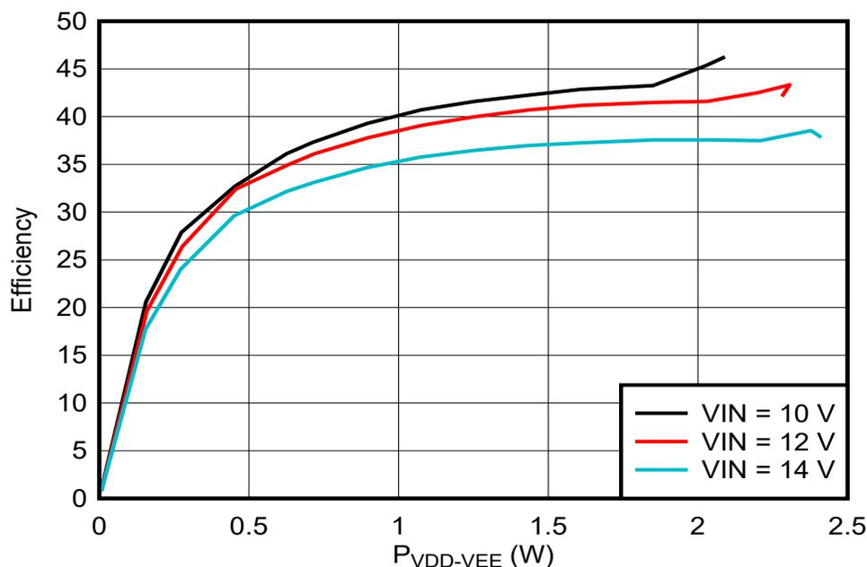
Figure 5-1. Measured Efficiency, VDD-VEE Loading Only
