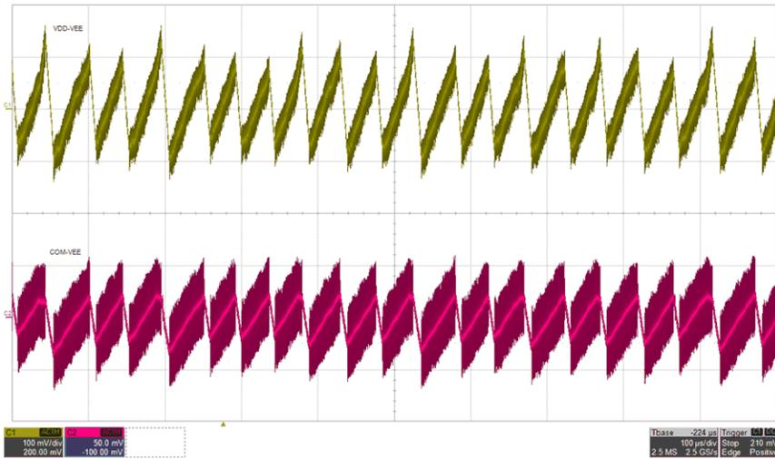
Figure 5-14. AC Ripple: VIN=12 V, IVDD=68 mA, IVEE=30 mA (top: VDD-VEE, 100 mV/div, bot: COM-VEE, 50 mV/div), time = 100 μs/div
