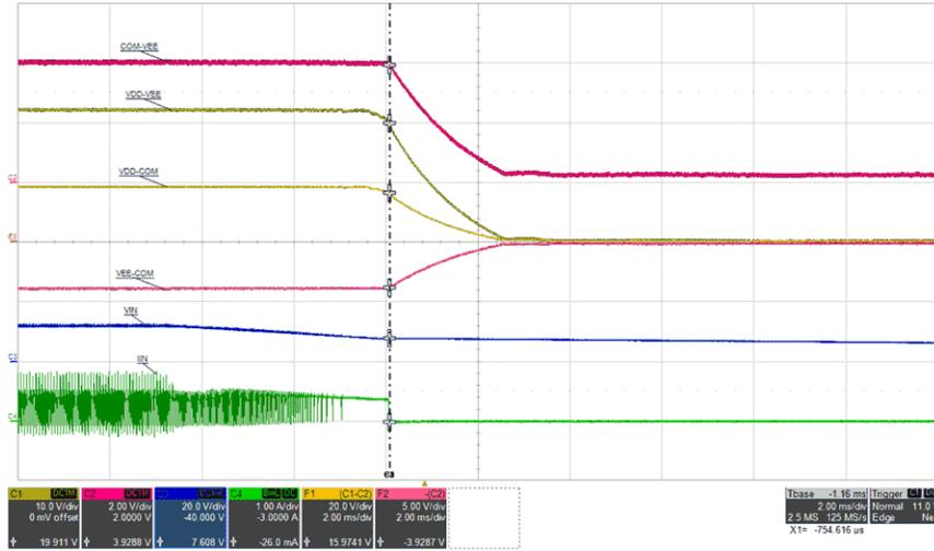
Figure 5-25. Shutdown by VIN Removal:  $V_{IN\text{OFF}}=7.6\text{ V}$ ,  $I_{VDD-VEE}=68\text{ mA}$  (top: COM-VEE, 2 V/div, mid-1: VDD-VEE, 10 V/div, mid-2: VDD-COM, 20 V/div, mid-3: VEE-COM, 5 V/div, mid-4: VIN, 20 V/div, bot: IIN, 1 A/div), time = 2 ms/div
