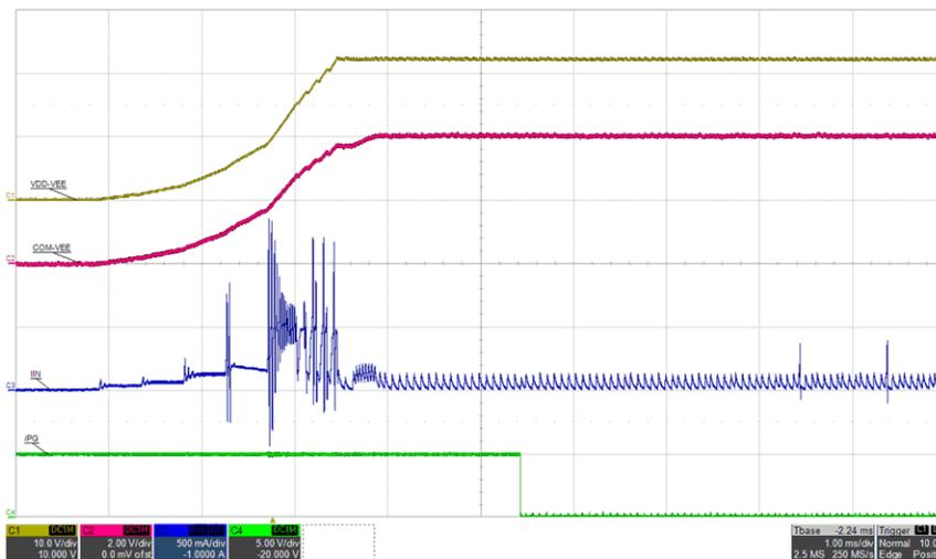
Figure 5-9. Inrush Current: VIN=12 V, I<sub>VDD-VEE</sub>=68 mA, (top: VDD-VEE, 10 V/div, mid-1: COM-VEE, 2 V/div, mid-2: IIN, 0.5 A/div, bot: /PG, 5 V/div), time = 1 ms/div
