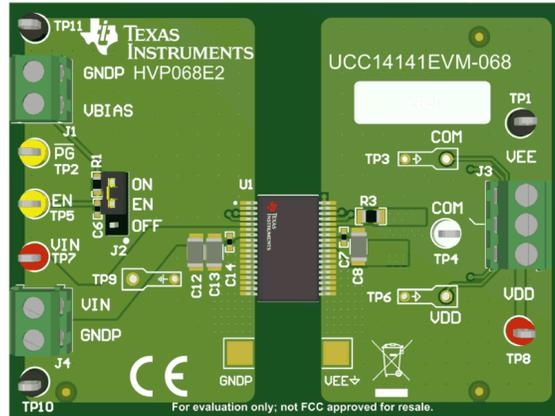
Figure 6-1. UCC14141EVM-068, Fully Assembled 3D Top View
