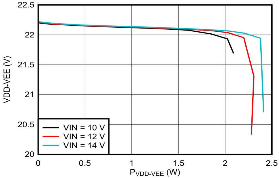
Figure 5-2. Regulation vs Power, VDD-VEE Loading Only
