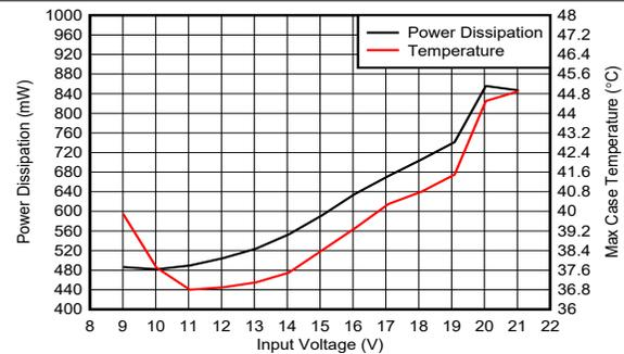
Figure 5-30. Power Dissipation and Case Temperature vs Input Voltage,  $T_A=23^\circ\text{C}$ ,  $0\text{ W}$
