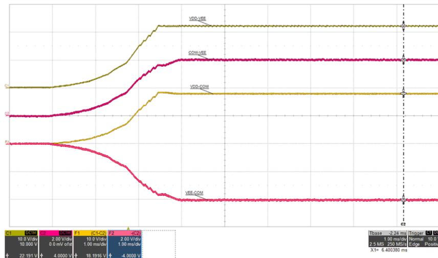
Figure 5-5. Start-up 1:  $V_{IN}=12$  V,  $I_{VDD-VEE}=0$  mA, (top: VDD-VEE, 10 V/div, mid-1: COM-VEE, 2 V/div, mid-2: VDD-COM, 10 V/div, bot: VEE-COM, 2 V/div), time = 1 ms/div
