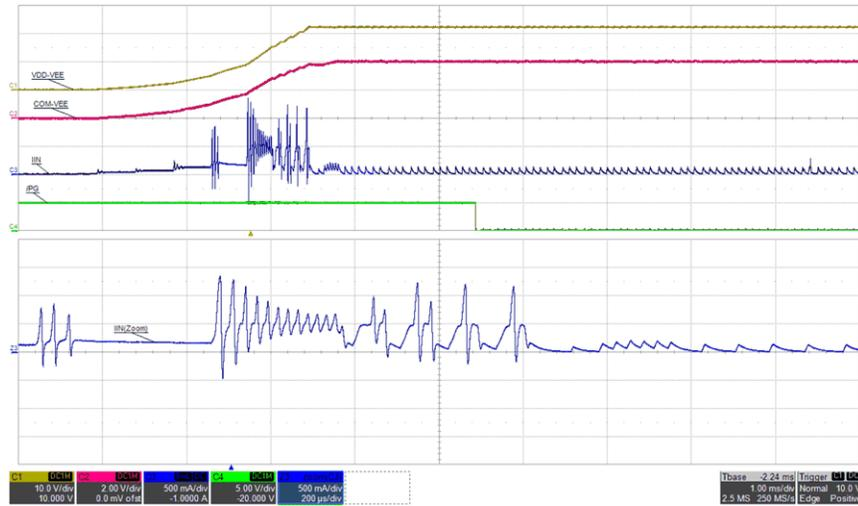
Figure 5-12. Inrush Current:  $V_{IN}=12\text{ V}$ ,  $I_{VDD-VEE}=68\text{ mA}$ , (top: VDD-VEE, 10 V/div, mid-1: COM-VEE, 2 V/div, mid-2: IIN, 0.5 A/div, bot: /PG, 5 V/div), time = 1 ms/div, time\_zoom=200  $\mu\text{s}$ /div
