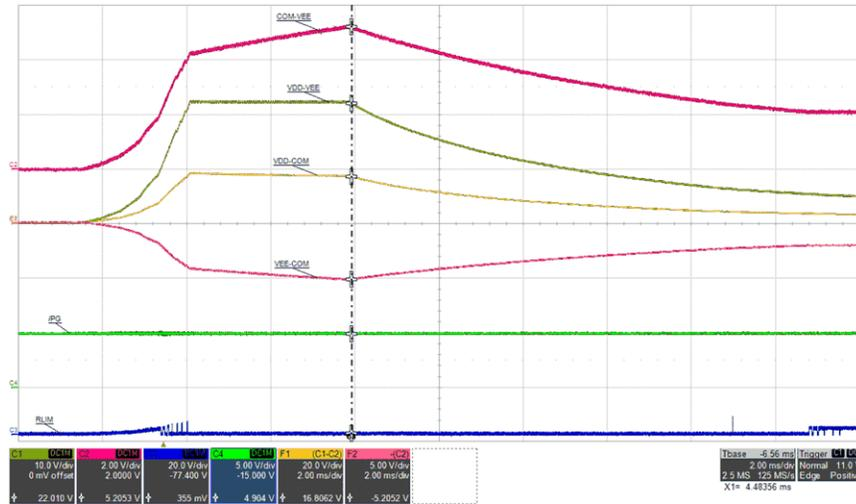
Figure 5-23. VEE OVP, VIN=12 V, PVDD=324 mW, PVEE=0 mW, (top: COM-VEE, 2 V/div, mid1: VDD-VEE, 10 V/div, mid2: VDD-COM, 20 V/div, mid3: VEE-COM, 5 V/div, mid4: /PG, 5 V/div, bot: RLIM, 20 V/div), time = 2 ms/div
