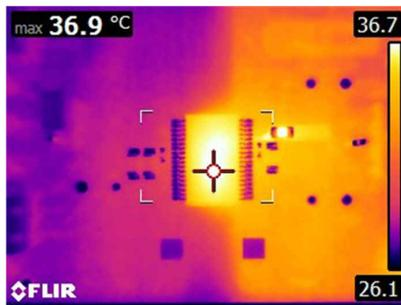
$V_{IN} = 12\text{ V}$      $V_{DD} = 22.21\text{ V}$      $I_{VDD} = 0\text{ mA}$
