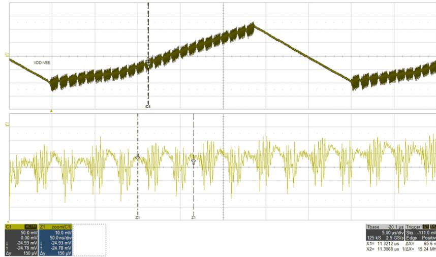
Figure 5-16. AC Ripple: VIN=12 V, IVDD=68 mA, FSW(PRI)=15.24 kHz (VDD-VEE, 50 mV/div, Zoom: VDD-VEE, 10 mV/div), time = 5 µs/div, time\_zoom=50 ns/div
