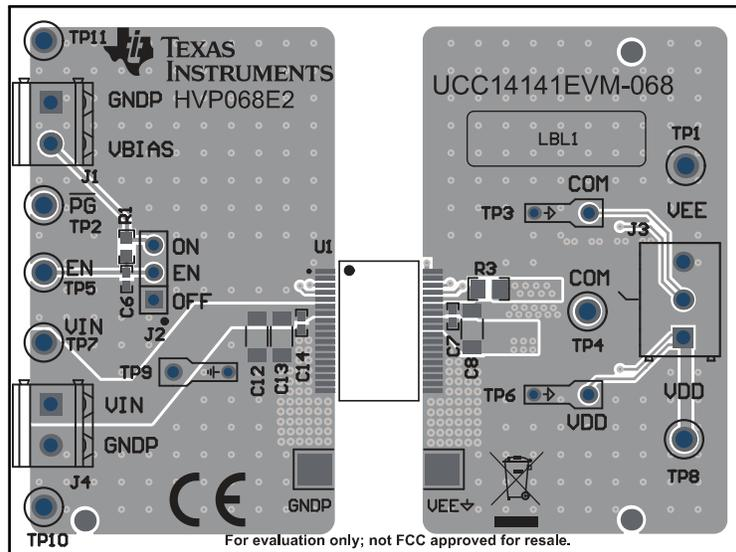
Figure 6-4. UCC14141EVM-068, PCB Top Layer, Assembly
