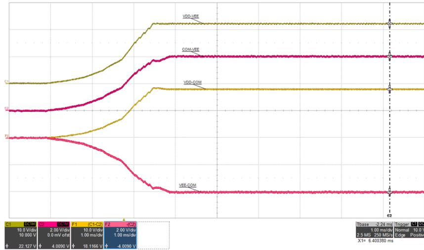
Figure 5-6. Start-up 2:  $V_{IN}=12\text{ V}$ ,  $I_{VDD-VEE}=68\text{ mA}$ , (top: VDD-VEE, 10 V/div, mid-1: COM-VEE, 2 V/div, mid-2: VDD-COM, 10 V/div, bot: VEE-COM, 2 V/div), time = 1 ms/div
