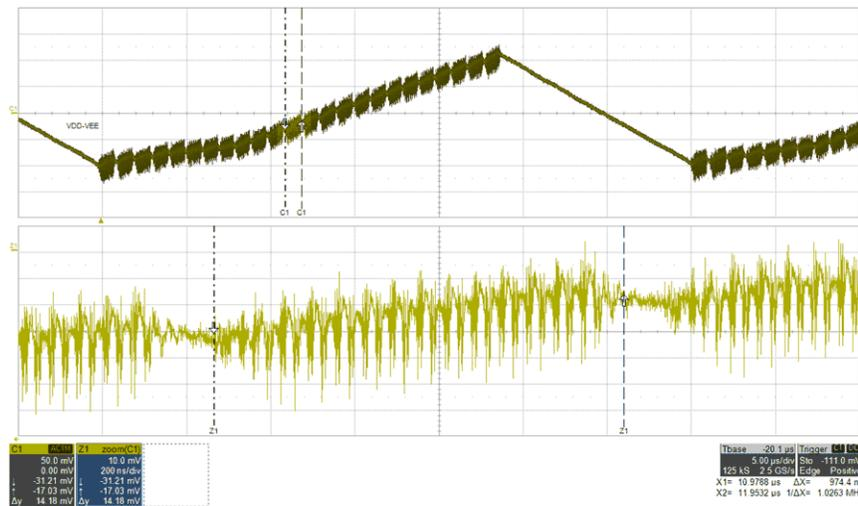
Figure 5-17. AC Ripple: VIN=12 V, IVDD=68 mA, FBURST=1 MHz (VDD-VEE, 50 mV/div, Zoom: VDD-VEE, 10 mV/div), time = 5 µs/div, time\_zoom=200 ns/div
