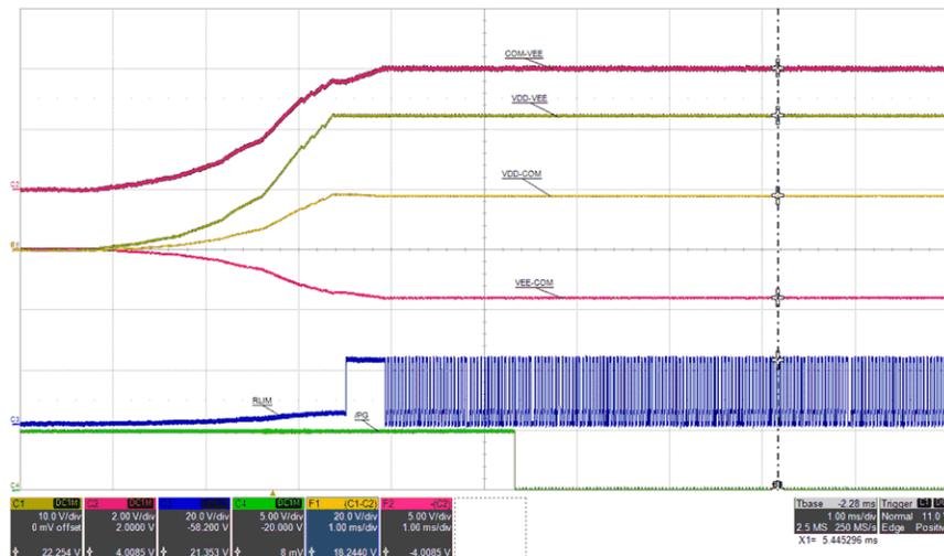
Figure 5-24. Normal Start, VIN=12 V, PVDD=324 mW, PVEE=106 mW, (top: COM-VEE, 2 V/div, mid1: VDD-VEE, 10 V/div, mid2: VDD-COM, 20 V/div, mid3: VEE-COM, 5 V/div, mid4: RLIM, 20 V/div, bot: /PG, 5 V/div), time = 1 ms/div
