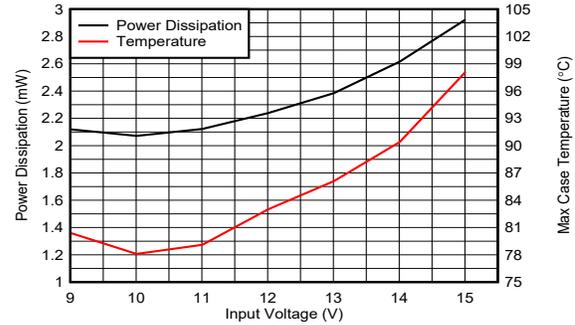
Figure 5-28. Power Dissipation and Case Temperature vs Input Voltage,  $T_A=23^\circ\text{C}$ ,  $1.52\text{ W}$
