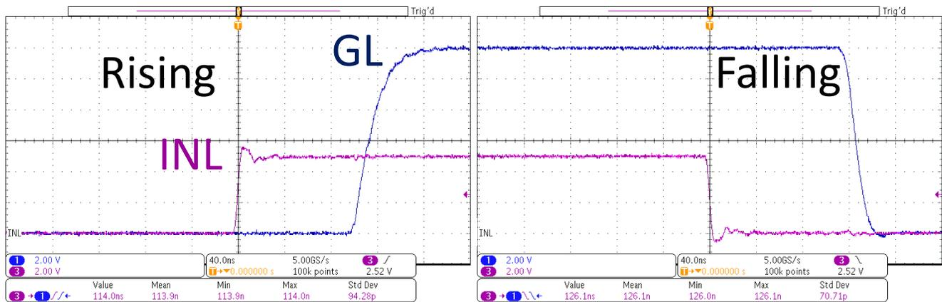
Figure 7-2. INL and GL Propagation Delay Waveforms (green is GL, dark blue is GL)
