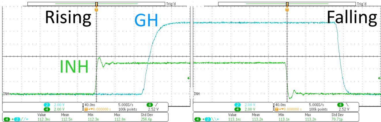
Figure 7-1. INH and GH Propagation Delay Waveforms (green is INH, blue is GH)
