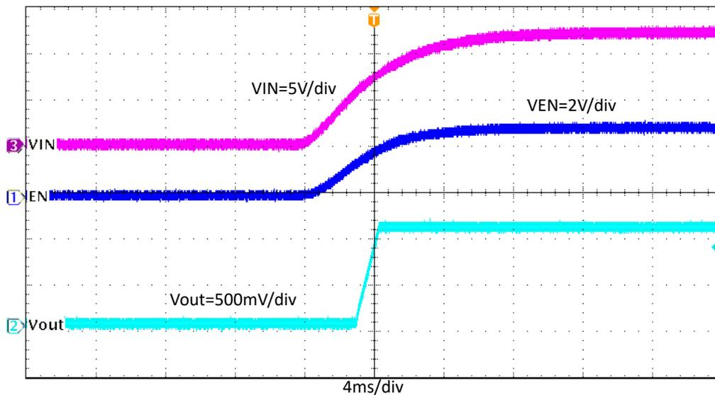
**Figure 4-10. TPS563203EVM Start-Up Relative to  $V_{IN}$**
