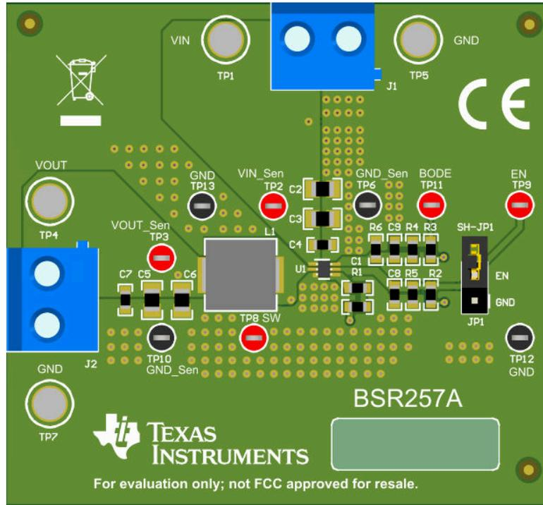
**Figure 4-1. TPS563203EVM Connectors and Jumpers Placement**
