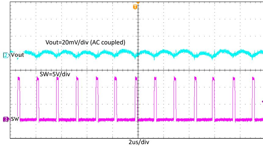
**Figure 4-14. TPS563203EVM Output Voltage Ripple,  $I_{OUT} = 3\text{ A}$**
