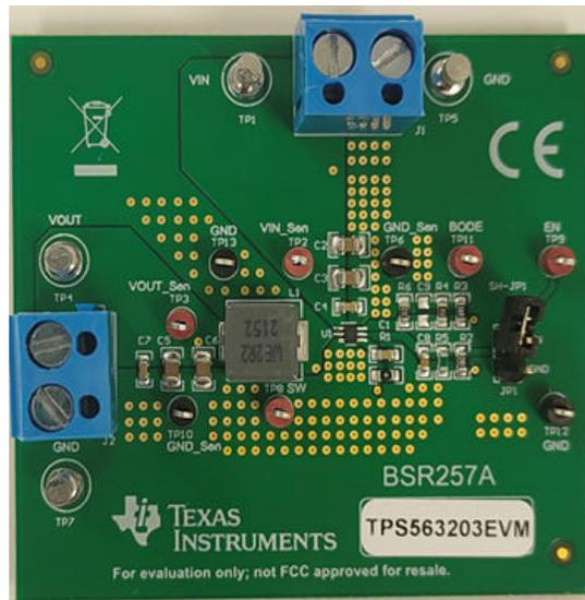
Figure 5-4. TPS563203EVM Board (Top View)
