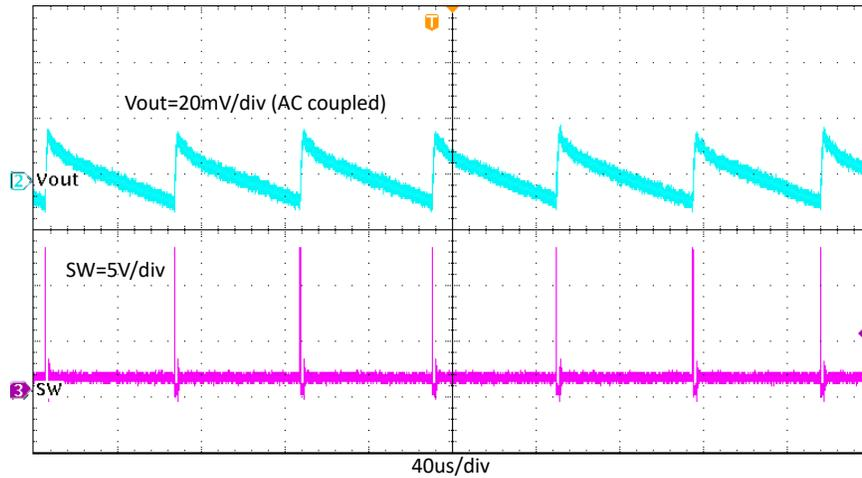
**Figure 4-15. TPS563203EVM Output Voltage Ripple,  $I_{OUT} = 0.01\text{ A}$**
