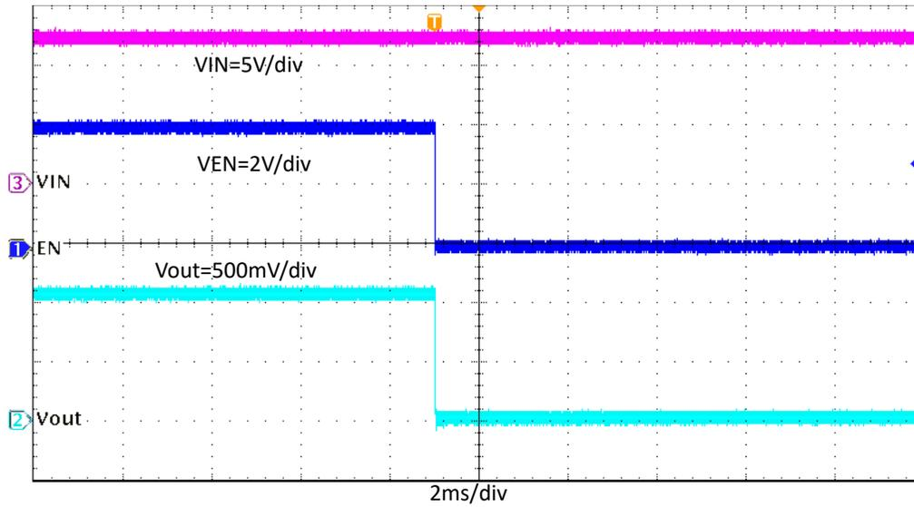
Figure 4-13. TPS563206EVM Shutdown Relative to EN
