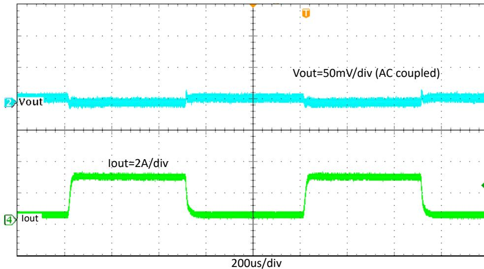
Figure 4-9. TPS563206EVM Load Transient Response, 10% to 90% (0.3 A to 2.7 A) Load Step
