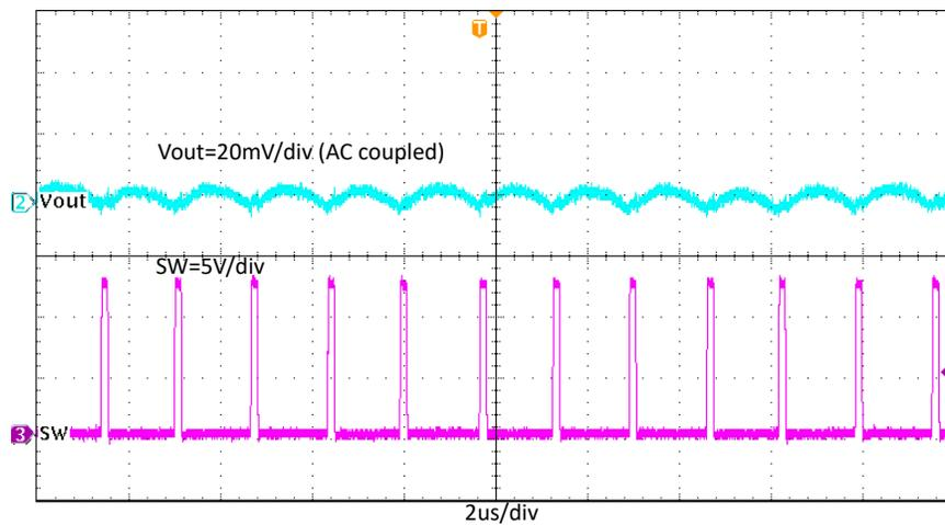
**Figure 4-16. TPS563206EVM Output Voltage Ripple,  $I_{OUT} = 0.01\text{ A}$**
