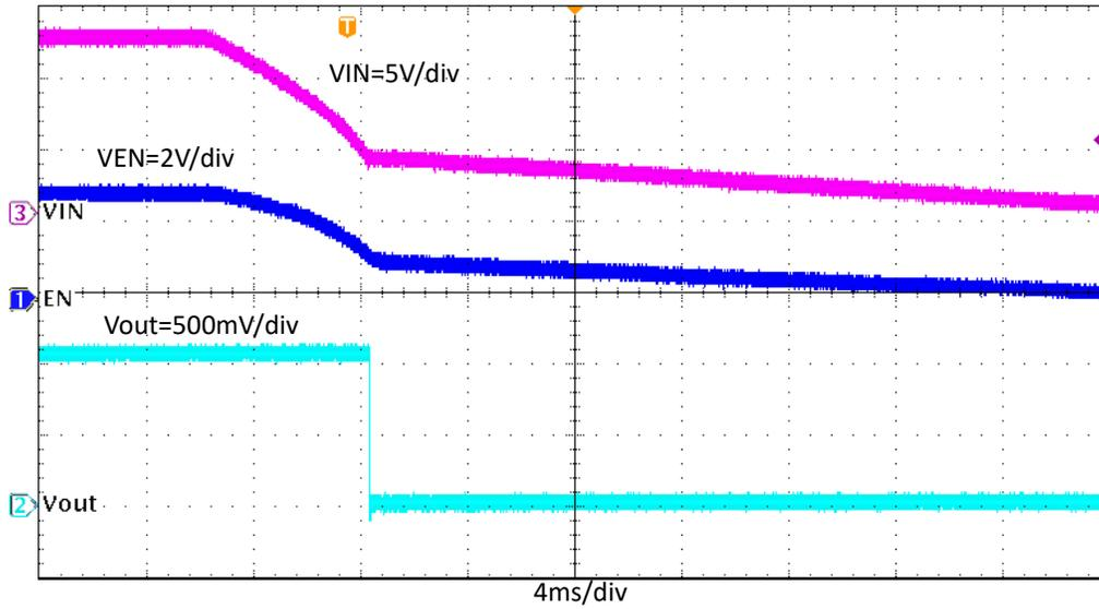
Figure 4-12. TPS563203EVM Shutdown Relative to  $V_{IN}$
