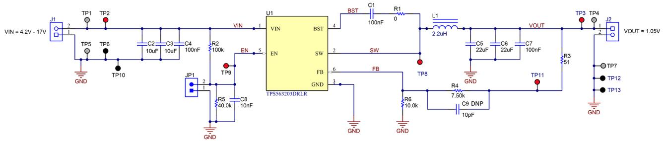
**Figure 6-1. TPS563203EVM Schematic Diagram**
