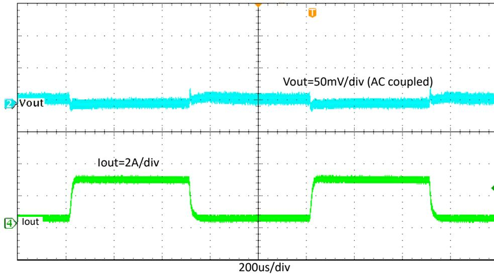
Figure 4-8. TPS563203EVM Load Transient Response, 10% to 90% (0.3 A to 2.7 A) Load Step
