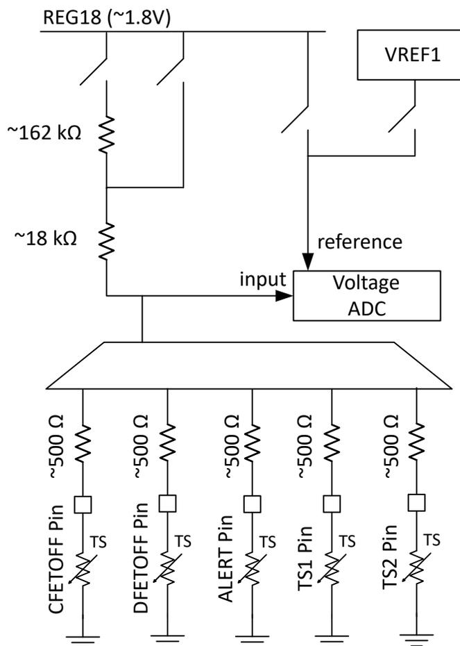
**Figure 4-3. External Thermistor Biasing**
