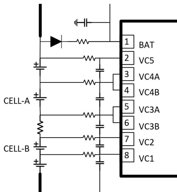
**Figure 4-1. Using Cell Input Pins for Interconnect Measurement**
