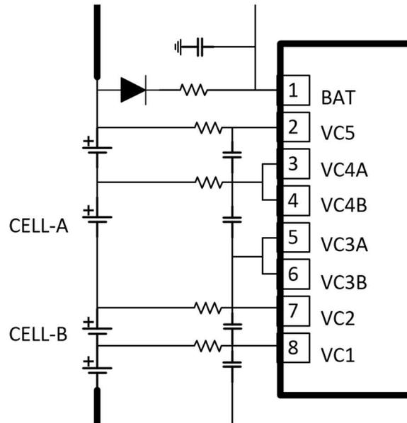
Figure 4-2. Terminating an Unused Cell Input Pin
