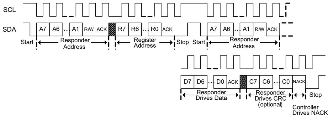
**Figure 9-3. I<sup>2</sup>C Read Without Repeated Start**
