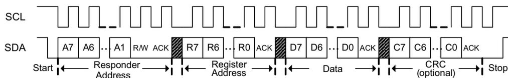
**Figure 9-1. I<sup>2</sup>C Write**
