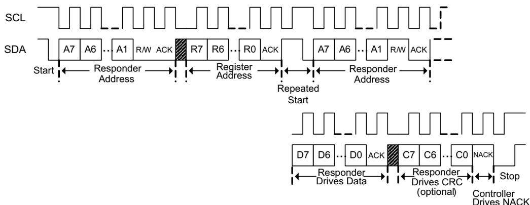
**Figure 9-2. I<sup>2</sup>C Read with Repeated Start**
