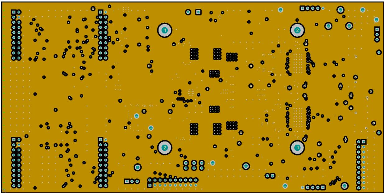
Figure 11. TPS92520EVM-074 Inner Layer (Ground Plane)
