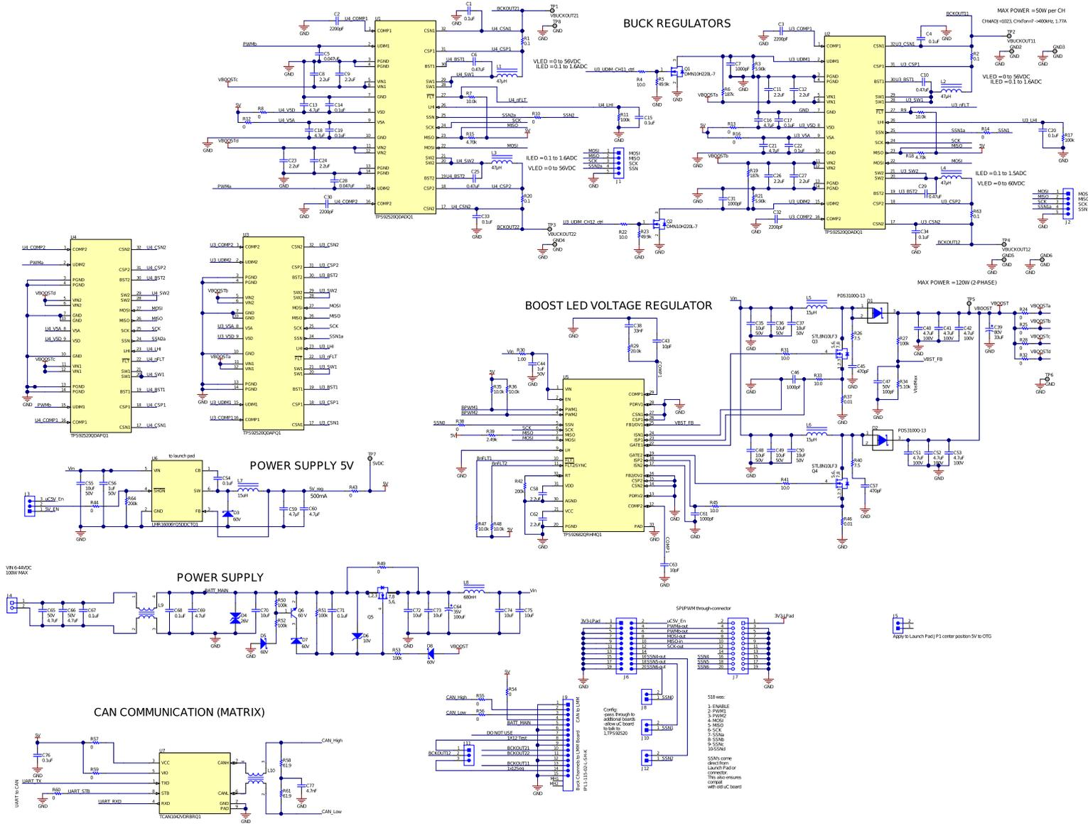
Figure 8. TPS92520EVM-074 Schematic
