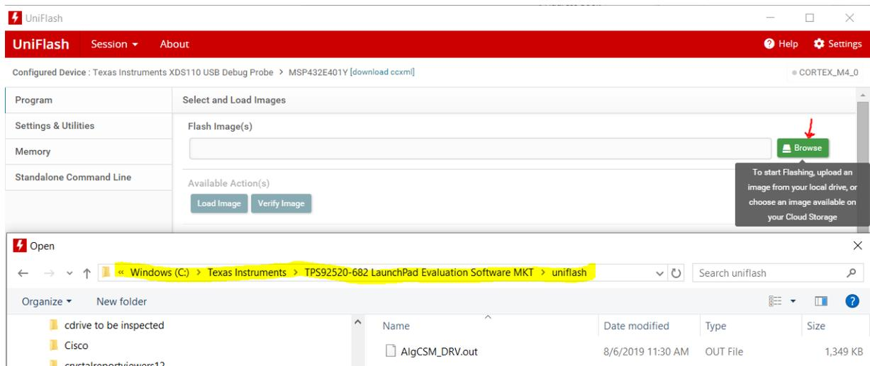
**Figure 29. UniFlash Programming, Step 4**
