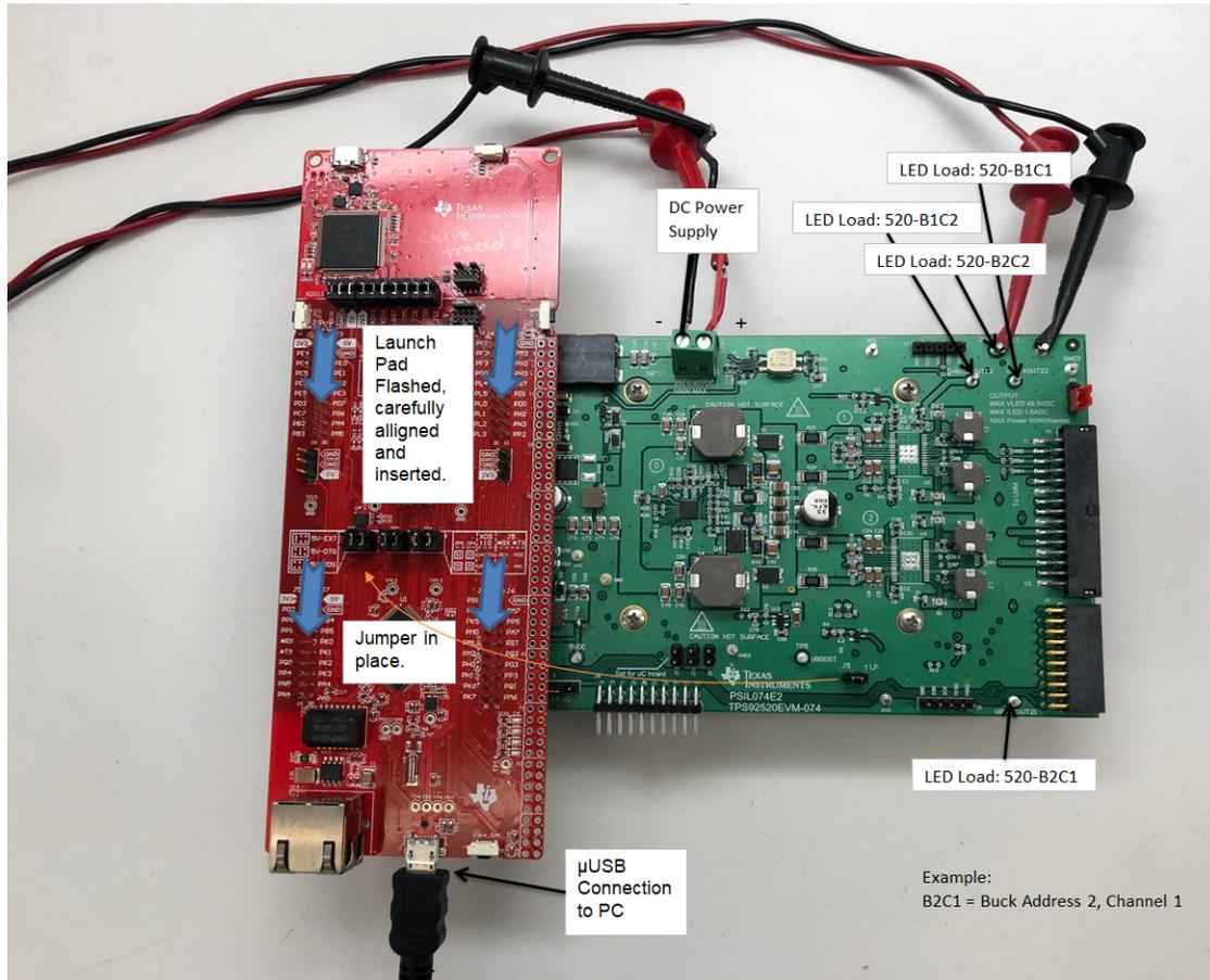
**Figure 33. LaunchPad Connection to the TPS92520EVM-074**
