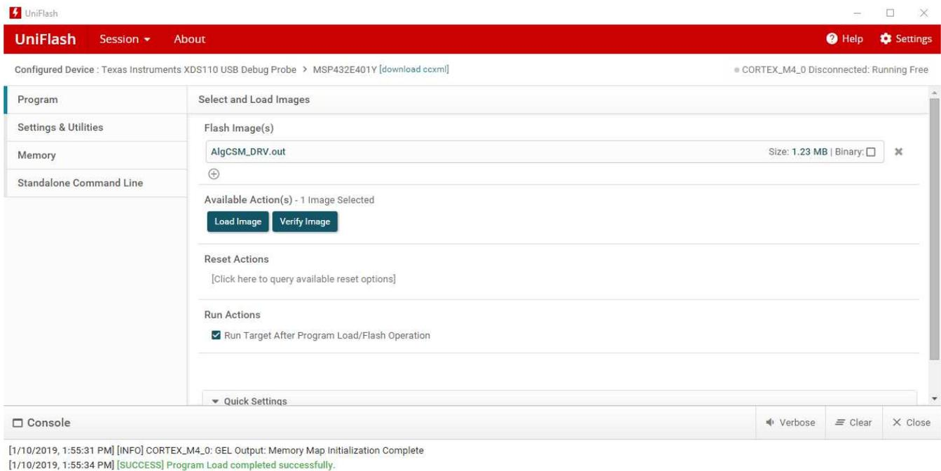
**Figure 30. UniFlash Programming, Step 5**
