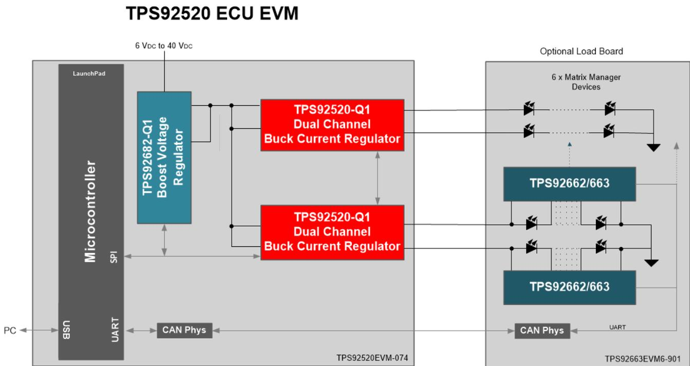
Figure 1. TPS92520EVM-074 Block Diagram
