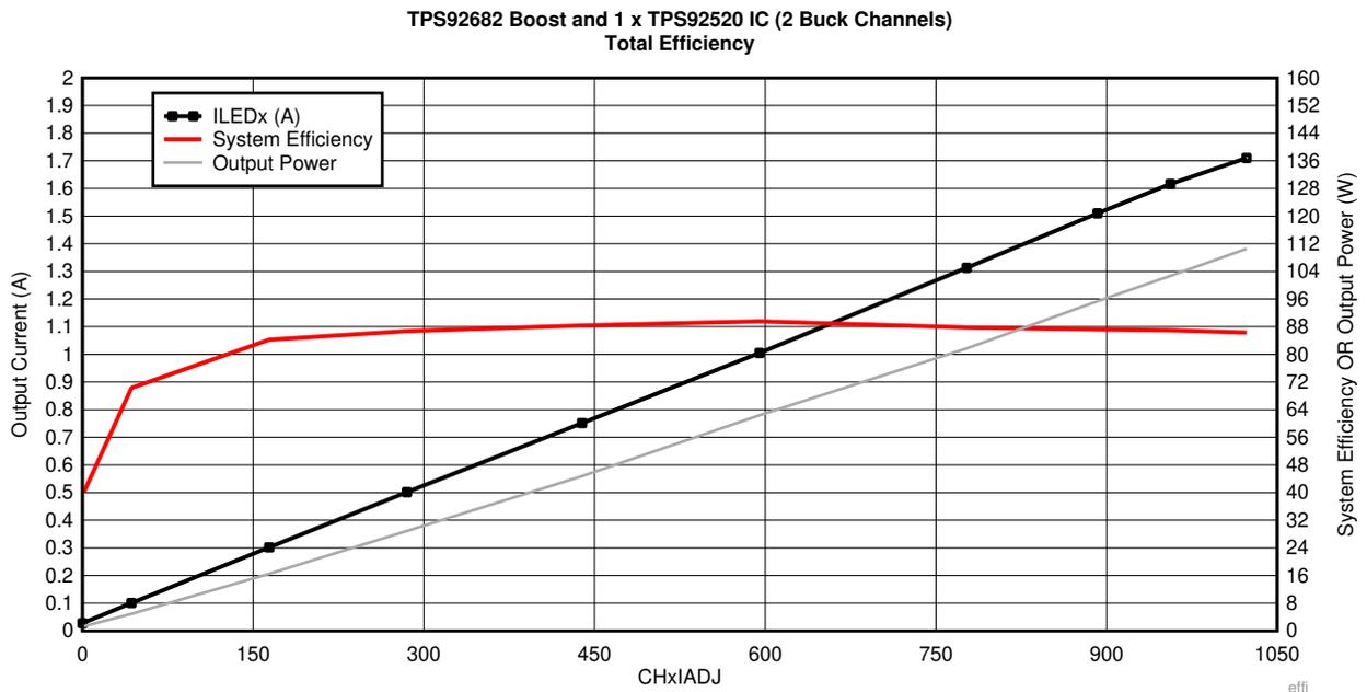
**Figure 5. ECU Metrics, V<sub>IN</sub> = 12 V, TPS92682 Boost Channel and 2 Channels from 1 x TPS92520 IC**
