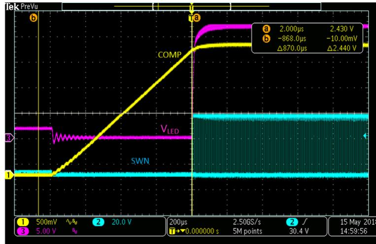
Figure 6. Start-up Waveforms
