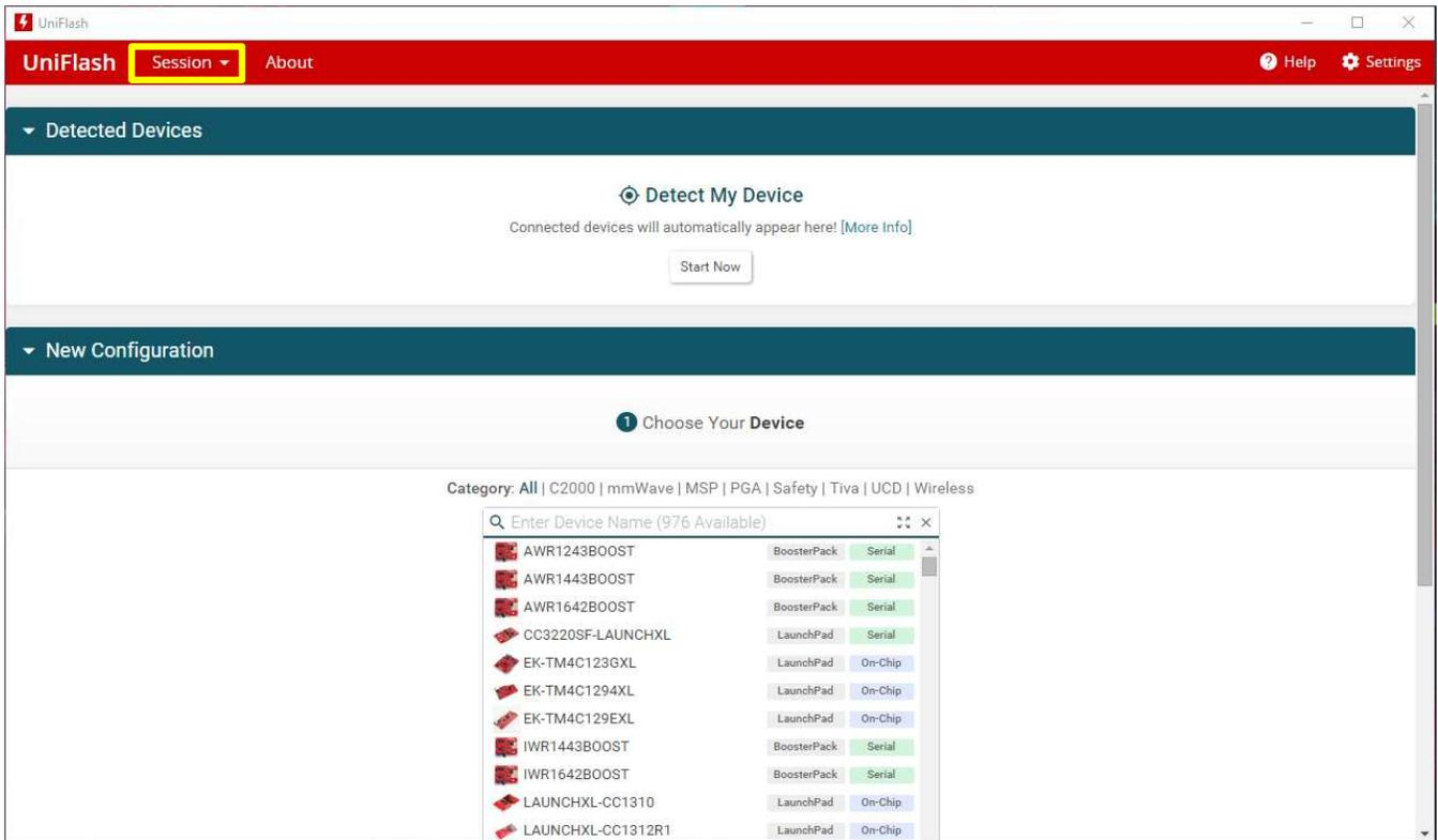
**Figure 27. UniFlash Programming, Step 1**
