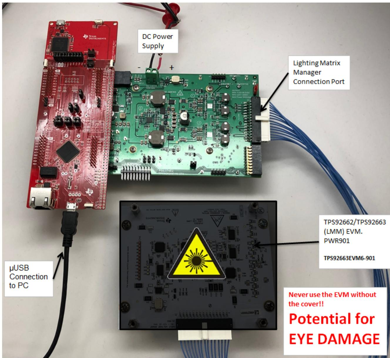
**Figure 34. LaunchPad Connection to the TPS92520EVM-074 and PWR901 Matrix Manager EVM**
