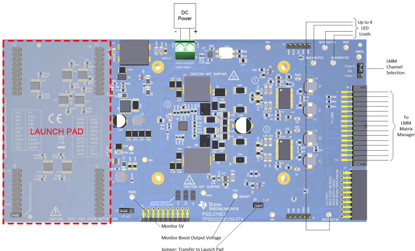
**Figure 2. Component Connections**
