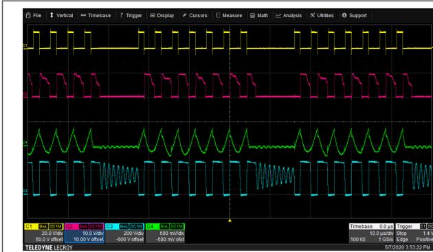
**Figure 8-11. Typical Waveform in ABM Operation**
