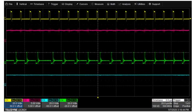
**Figure 8-30. Boost Operation at 5 V<sub>OUT</sub> and Full Load (Yellow = PWML, Red = BIN, Green = BSW, Blue = VDD)**
