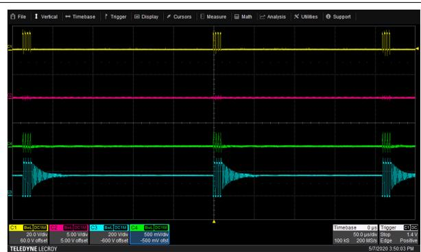
**Figure 8-14. Typical Waveform in SBP2 Operation**
