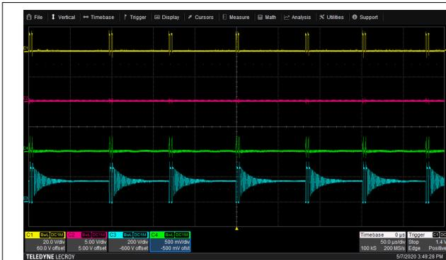
**Figure 8-13. Typical Waveform in SBP1 Operation**
