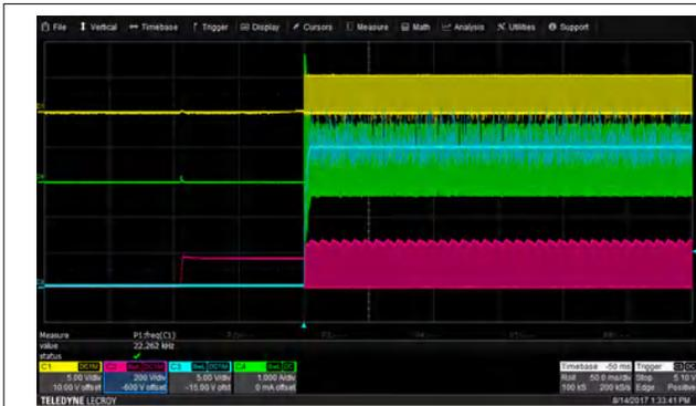
**Figure 8-15. 115 V<sub>AC</sub> and Full Load Startup**
