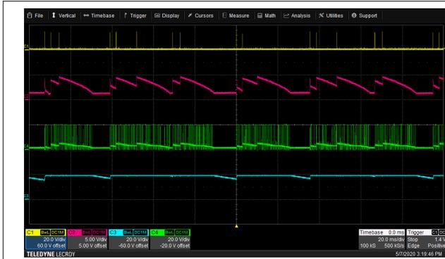
**Figure 8-29. Boost Operation at 5 V<sub>OUT</sub> and No Load (Yellow = PWML, Red = BIN, Green = BSW, Blue = VDD)**
