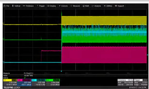
**Figure 8-16. 230 V<sub>AC</sub> and Full Load Startup**
