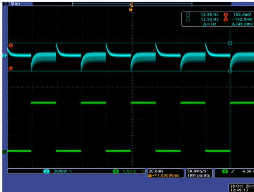
Figure 19. 300 mA to 15 A Transient (Ch2 =  $V_{OUT}$  AC Coupled; Ch4 =  $I_{OUT}$ )
