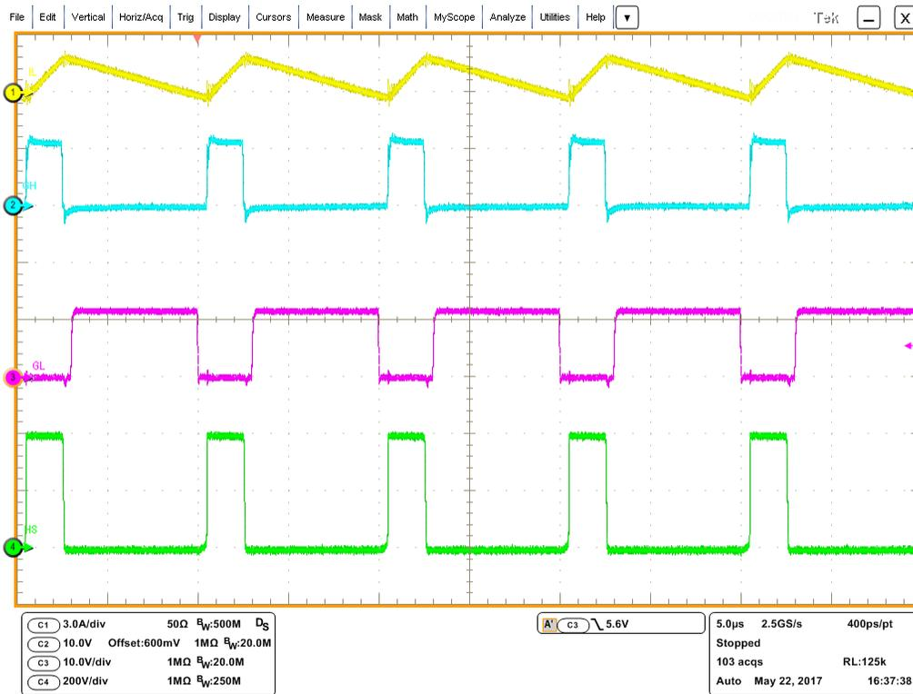
Figure 9. Buck Converter IL, GH, GL, and HS
