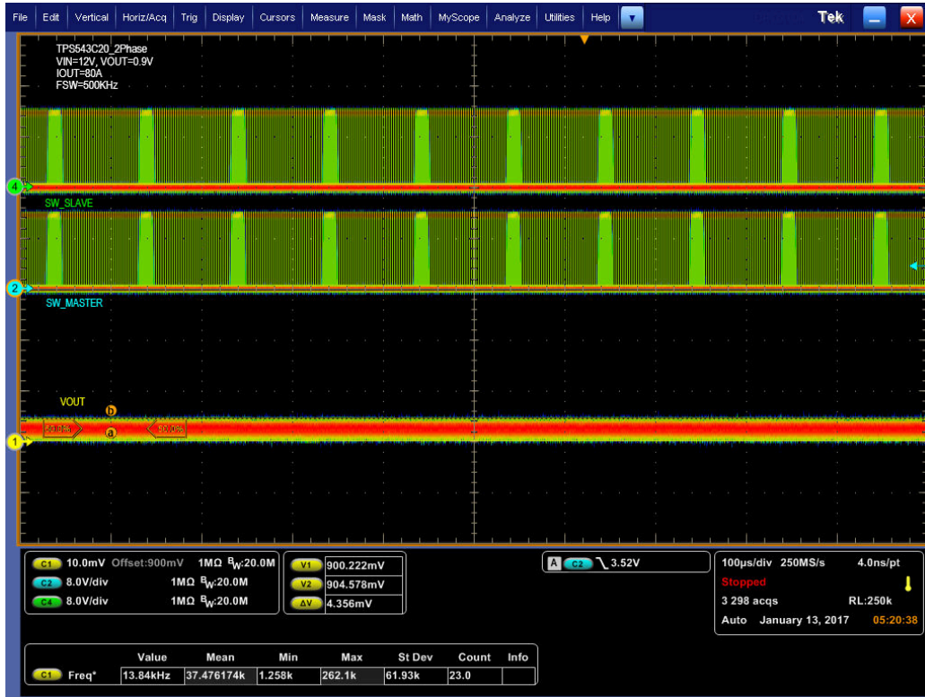
Figure 9-7. Output Ripple and SW Node of 0.9-V Output at 12 V IN , 80-A Output
