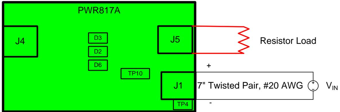
Figure 2. Typical TPS254900Q1EVM-817 Test Setup
