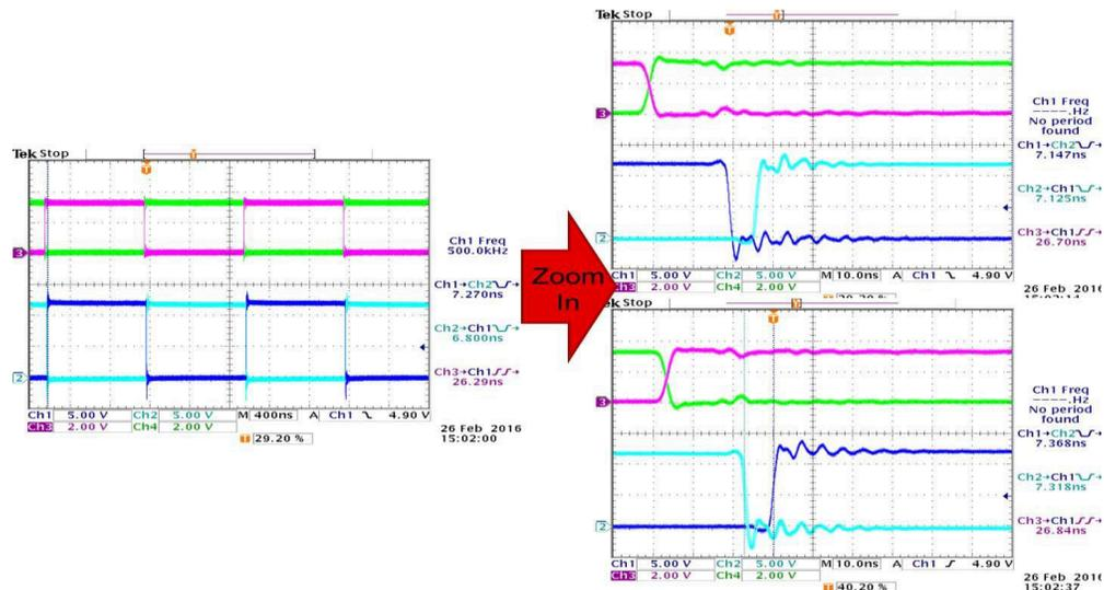
Figure 7-2. Test Waveforms if DT is Left Open (Channel 3 and 4 are PWM Inputs, and Channel 1 and 2 are Driver Outputs)
