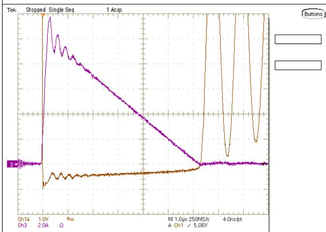
Figure 16. Diode Current and Voltage on [UCC28740EVM-525](#) at 265-V<sub>AC</sub> Input
