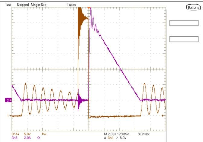
Figure 11. 100%-Load Diode Current and Voltage on [UCC28740EVM-525](#) at 265-V<sub>AC</sub> Input
