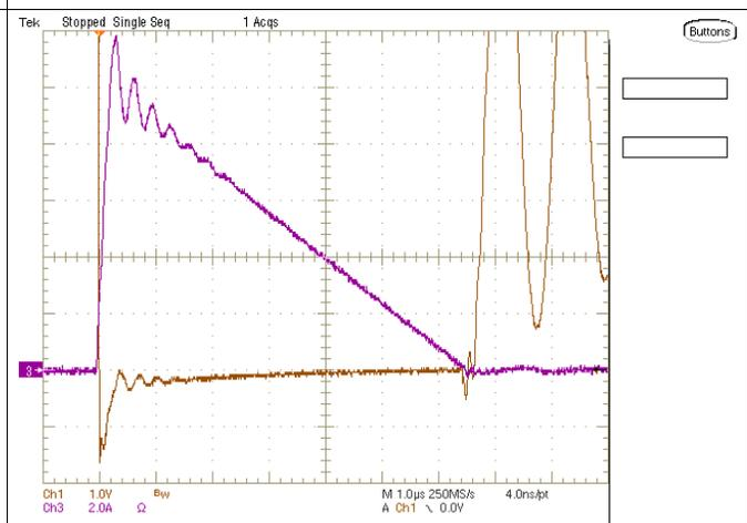
Figure 17. SR Current and Voltage on [UCC28740EVM-525](#) at 265-V<sub>AC</sub> Input
