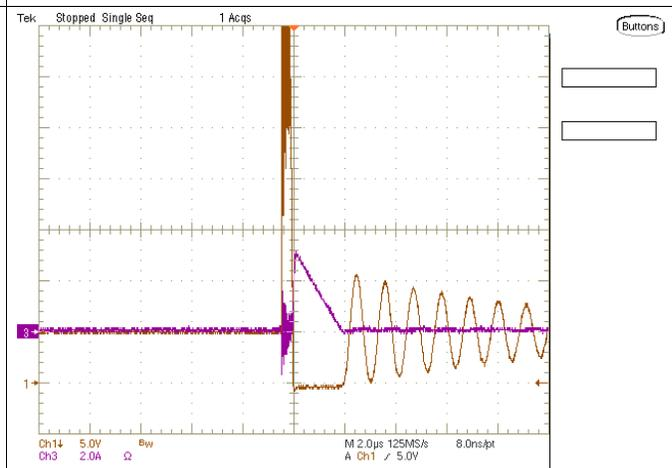
Figure 13. 1%-Load Diode Current and Voltage on [UCC28740EVM-525](#) at 265-V<sub>AC</sub> Input
