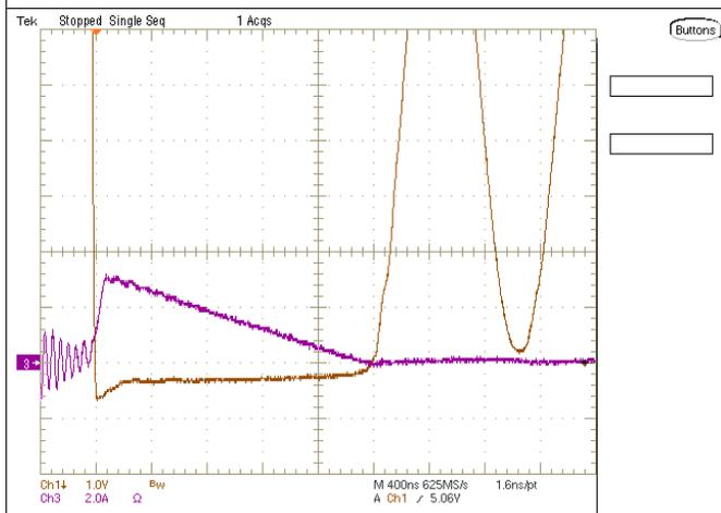
Figure 20. Diode Current and Voltage on [UCC28740EVM-525](#) at 265-V<sub>AC</sub> Input
