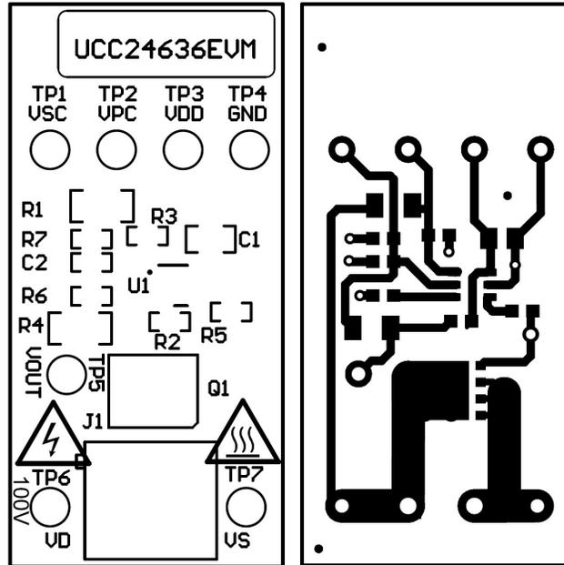
Figure 27. UCC24636EVM Assembly and Copper Drawings (Top View)
