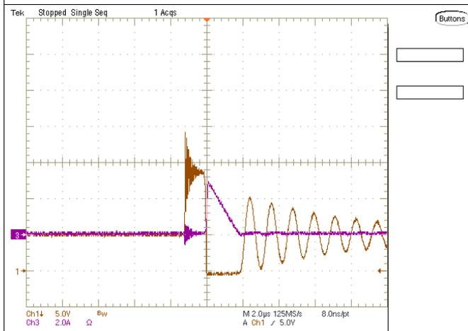
Figure 12. 1%-Load Diode Current and Voltage on [UCC28740EVM-525](#) at 85-V<sub>AC</sub> Input
