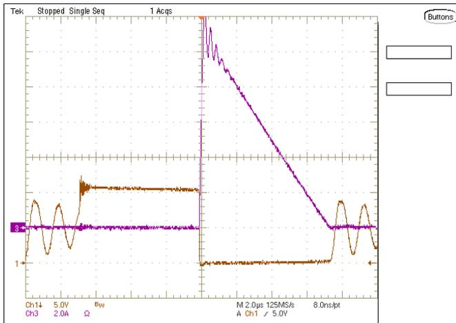
Figure 10. 100%-Load Diode Current and Voltage on [UCC28740EVM-525](#) at 85-V<sub>AC</sub> Input
