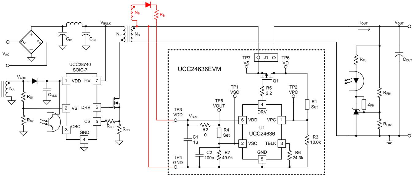
Figure 25. UCC24636EVM Used in the *High-Side* Rectifier Configuration
