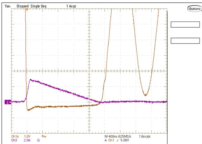
Figure 18. Diode Current and Voltage on [UCC28740EVM-525](#) at 85-V<sub>AC</sub> Input
