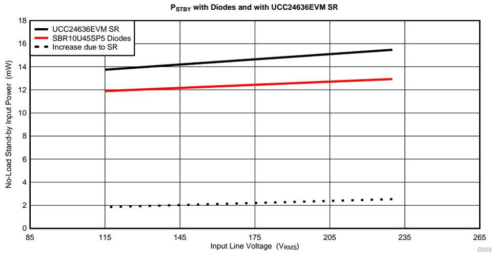
Figure 24. Comparison of No-Load Input Power Consumption
