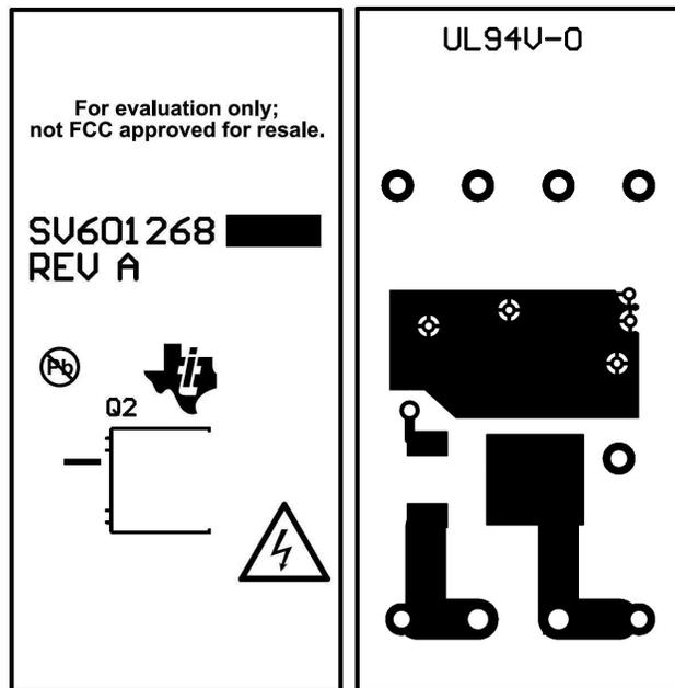
Figure 28. UCC24636EVM Assembly and Copper Drawings (Bottom View)
