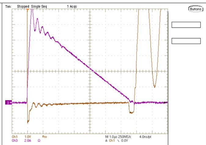
Figure 15. SR Current and Voltage on [UCC28740EVM-525](#) at 85-V<sub>AC</sub> Input
