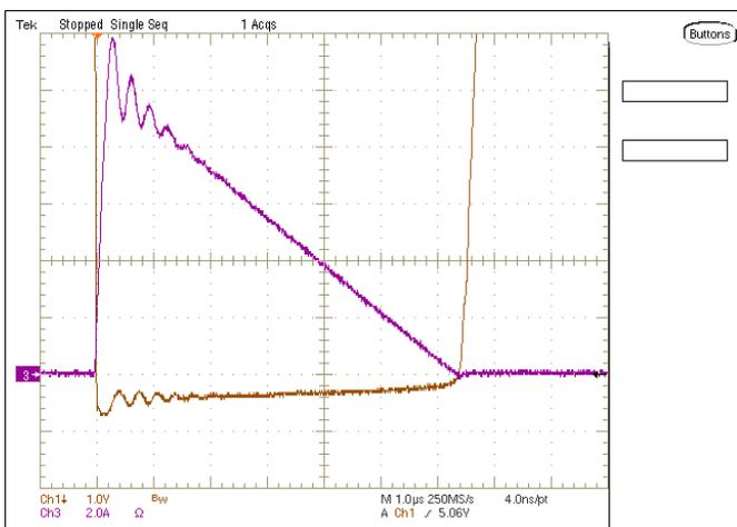
Figure 14. Diode Current and Voltage on [UCC28740EVM-525](#) at 85-V<sub>AC</sub> Input
