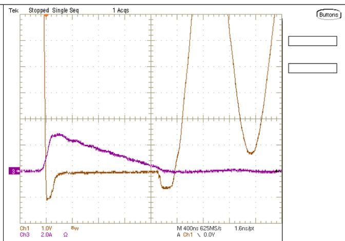
Figure 19. SR Current and Voltage on [UCC28740EVM-525](#) at 85-V<sub>AC</sub> Input
