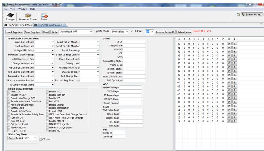
Figure 9. Main Window of the bq2589x Evaluation Software
