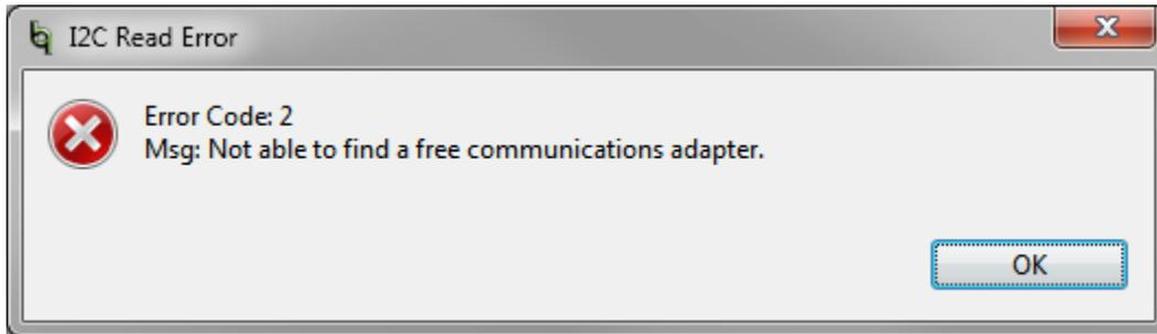
**Figure 5. Communications Adapter Error**
