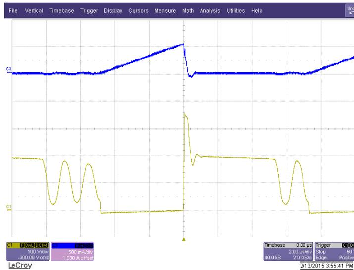
**Figure 13. Primary-Side Switching Waveforms 85 V<sub>AC</sub>**
