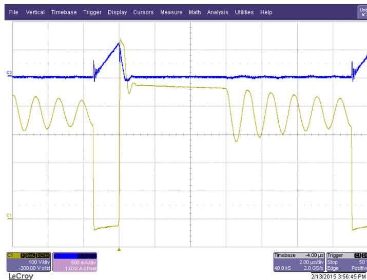
**Figure 14. Primary-Side Switching Waveforms 265 V<sub>AC</sub>**
