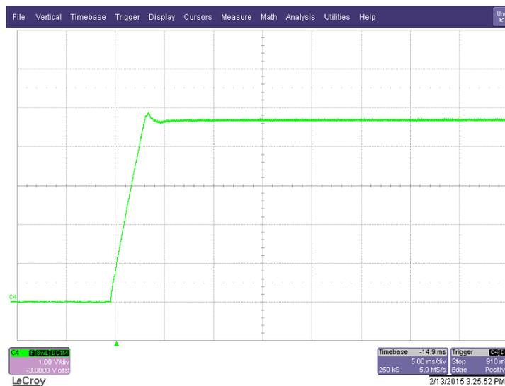
Figure 12. Output Voltage Start, 230 V<sub>AC</sub>, 1.5-A load, 1 V/div 50 ms/div
