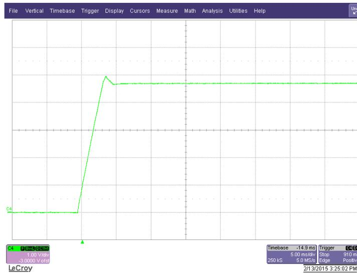
Figure 11. Output Voltage Start 115 V<sub>AC</sub>, 1.5-A load, 1 V/div 50 mS/div
