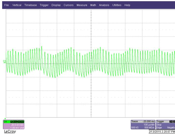
Figure 7. Ripple with 5 V, 1.5 A Out, 115 V<sub>AC</sub> in 20 mV/div 100  $\mu$ s/div
