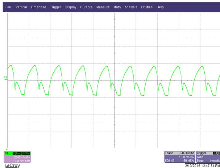
Figure 8. Ripple with 5 V, 1 A Out, 115 V<sub>AC</sub> in 20 mV/div 100  $\mu$ s/div
