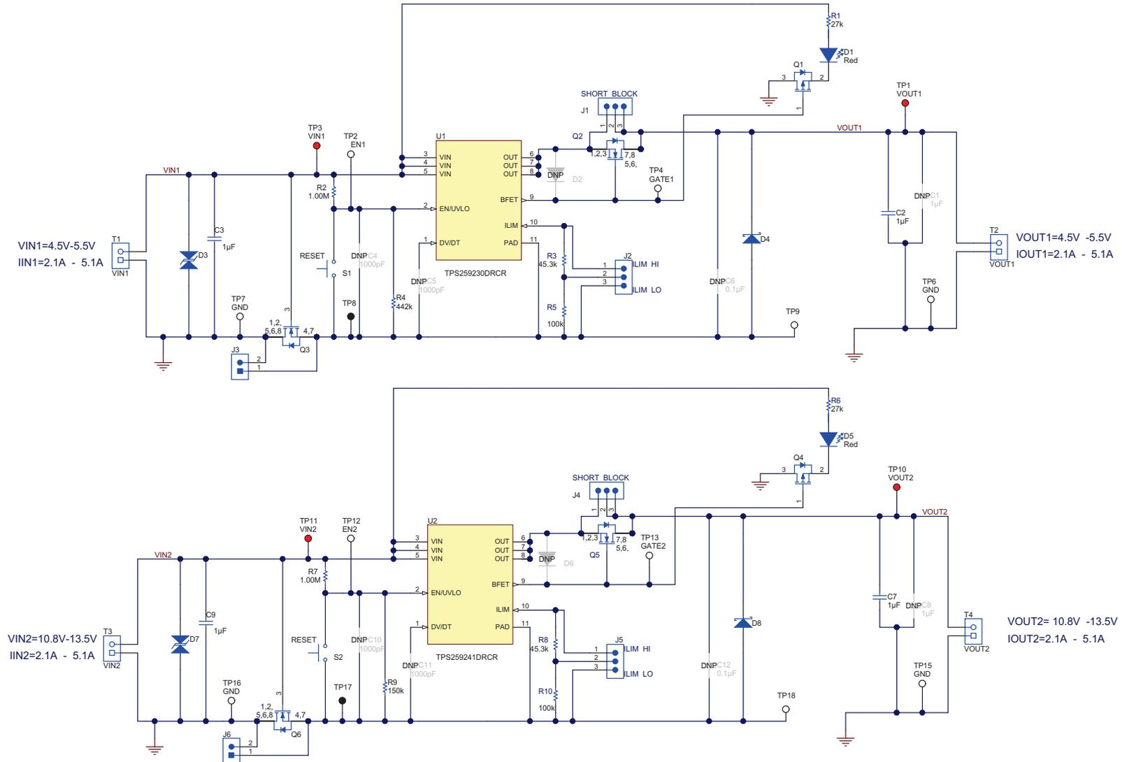
Figure 1. TPS259230-41EVM Schematic
