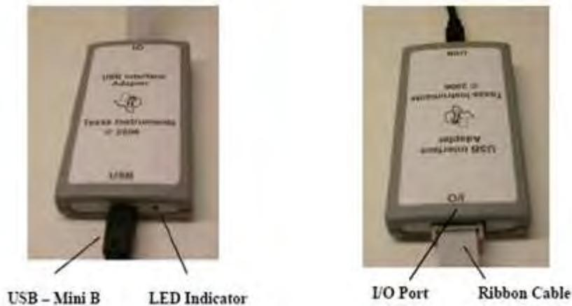
Figure 4. USB-to-GPIO Interface Adapter (HPA172)
