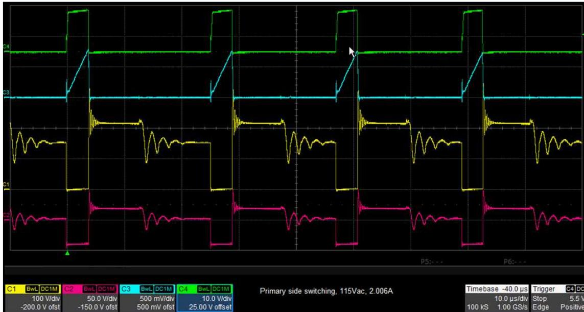
Figure 14. Primary-Side Switching Waveform
