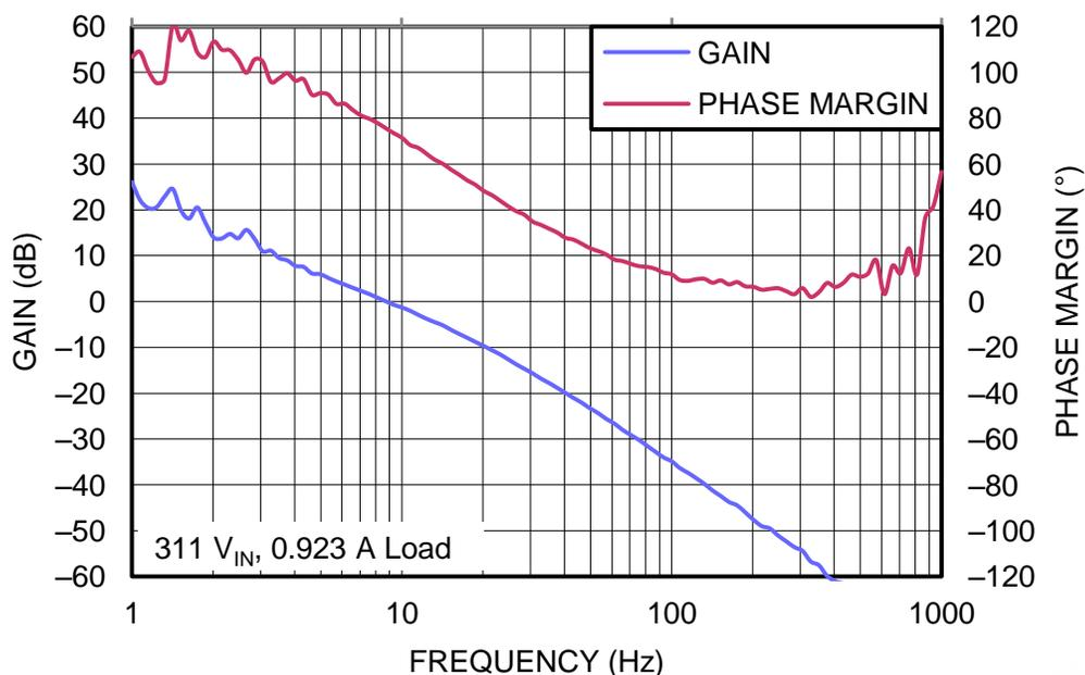
Figure 21. UCC28180EVM-573 Voltage Loop Response Gain and Phase, (162-V<sub>DC</sub>, full load, f<sub>CO</sub> = 8.6-Hz, phase margin = 63 degrees)
