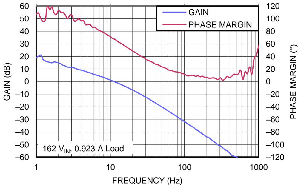
Figure 20. UCC28180EVM-573 Voltage Loop Response Gain and Phase, (311-V<sub>DC</sub>, full load, f<sub>CO</sub> = 10.7-Hz, phase margin = 68 degrees)
