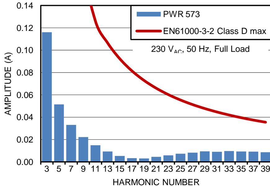
Figure 9. UCC28180EVM-573 Current Harmonics, (230-V<sub>AC</sub>, 50-Hz input, full load, without the fundamental)
