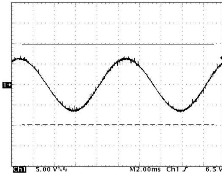
Figure 14. UCC28180EVM-573 Line Frequency Output Voltage Ripple (230 V<sub>AC</sub>, 50 Hz input, full load)
