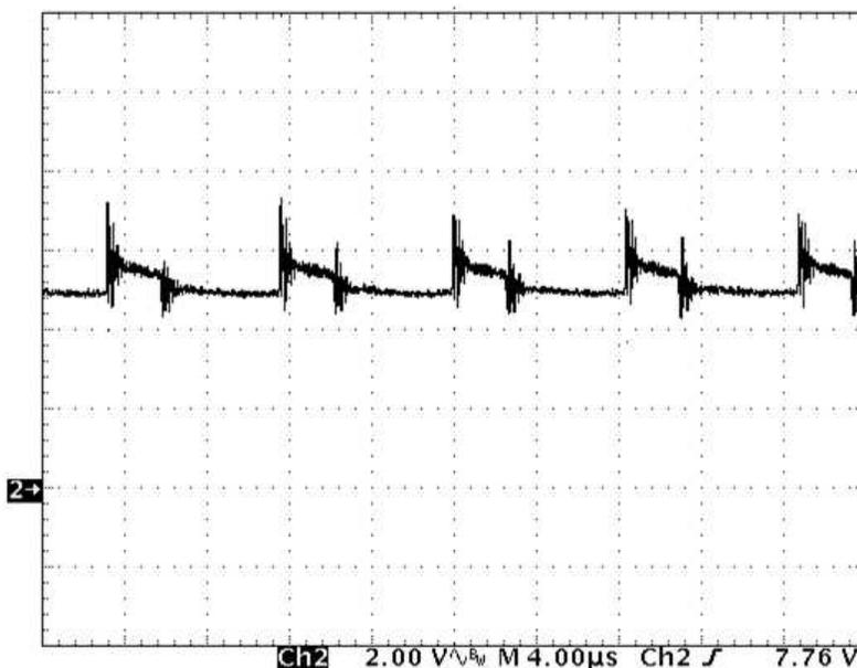
Figure 15. UCC28180EVM-573 Switching Frequency Output Voltage Ripple (115 V<sub>AC</sub>, 60 Hz input, full load)
