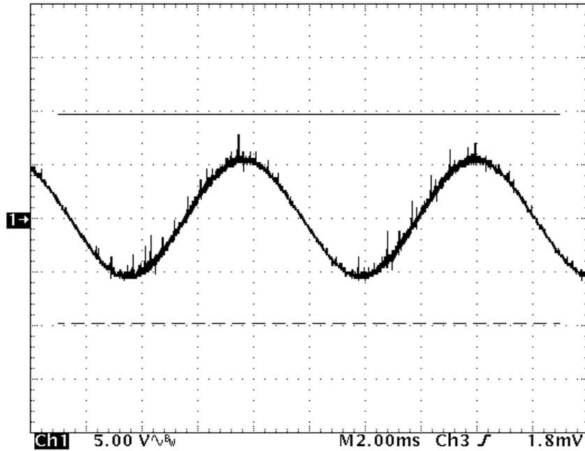
Figure 13. UCC28180EVM-573 Line Frequency Output Voltage Ripple (115 V<sub>AC</sub>, 60 Hz input, full load)
