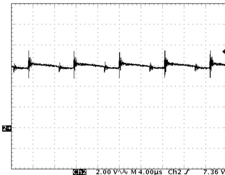
Figure 16. UCC28180EVM-573 Switching Frequency Output Voltage Ripple (230 V<sub>AC</sub>, 50 Hz input, full load)
