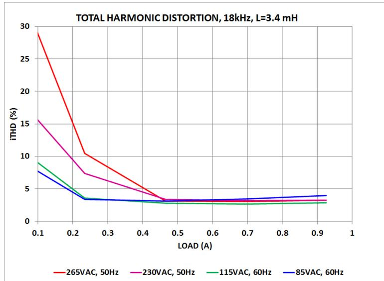
Figure 7. Total harmonic distortion (as a function of line voltage and load current) with L = 3.4 mH and f<sub>SW</sub> = 18 kHz
