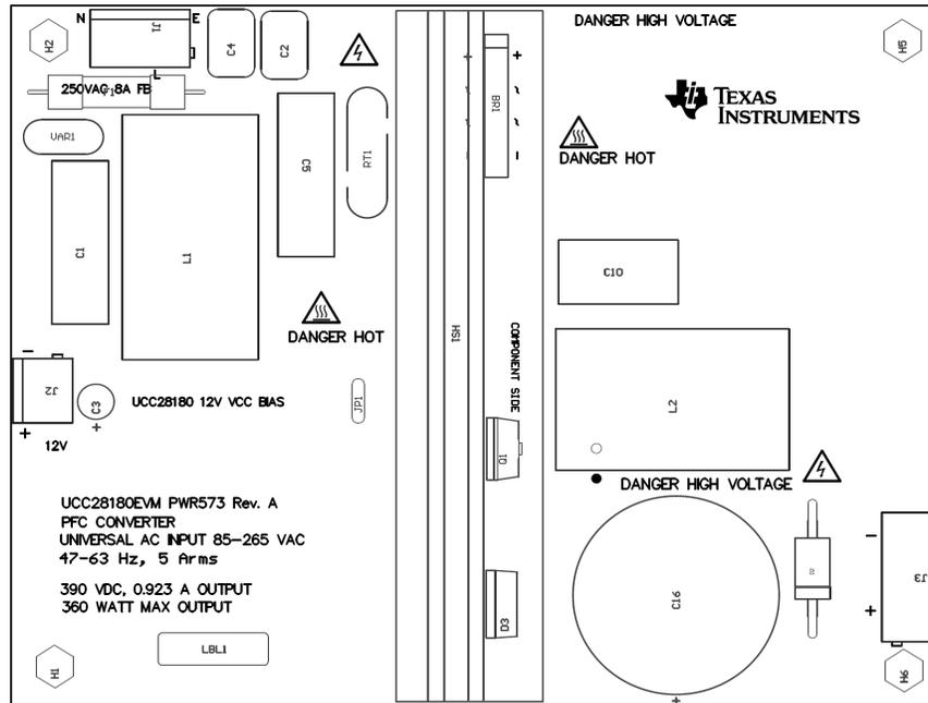
Figure 22. UCC28180EVM-573 Top Layer Assembly Drawing (top view)
