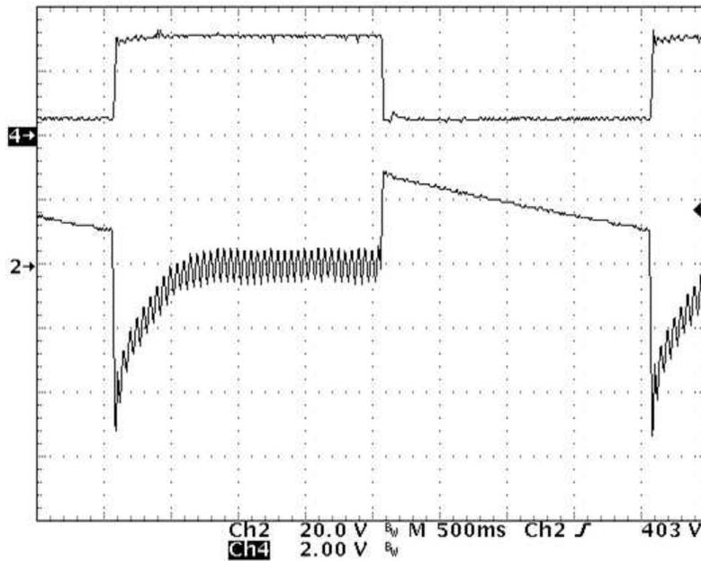
**Figure 19. Load Transient**
