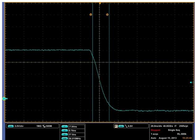
Figure 9. UCC27532DBV Input vs. Output PWM Fall Time
