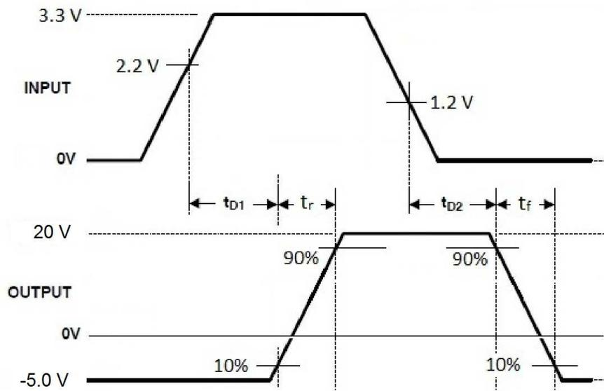
Figure 5. UCC27532EVM-538 Input vs. Output waveforms
