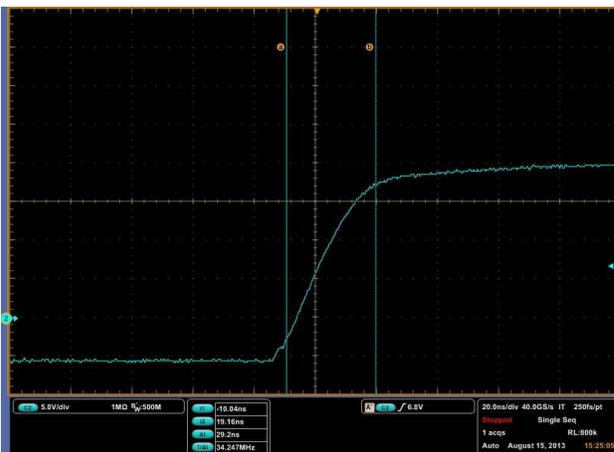
Figure 8. UCC27532DBV Input vs. Output PWM Rise Time
