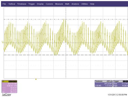
Figure 14 Ripple with 5V,700mA out 265Vac in 20mV/div 500µs/div
