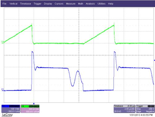
Figure 18 Primary side switching waveforms
