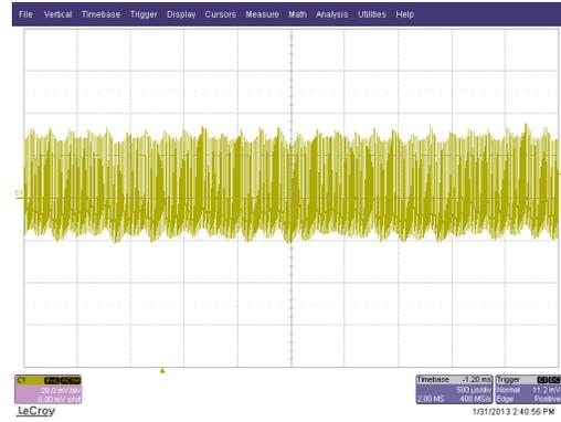
Figure 13 Ripple with 5V,1.2A out 265Vac in 20mV/div 500µs/div
