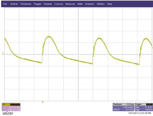
Figure 12 Ripple with 5V,1.2A out 265Vac in 20mV/div 5µs/div
