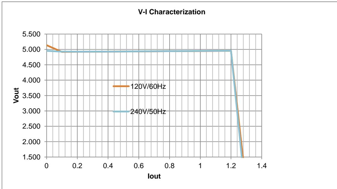
Figure6. Typical V-I Characteristic at 25°C
