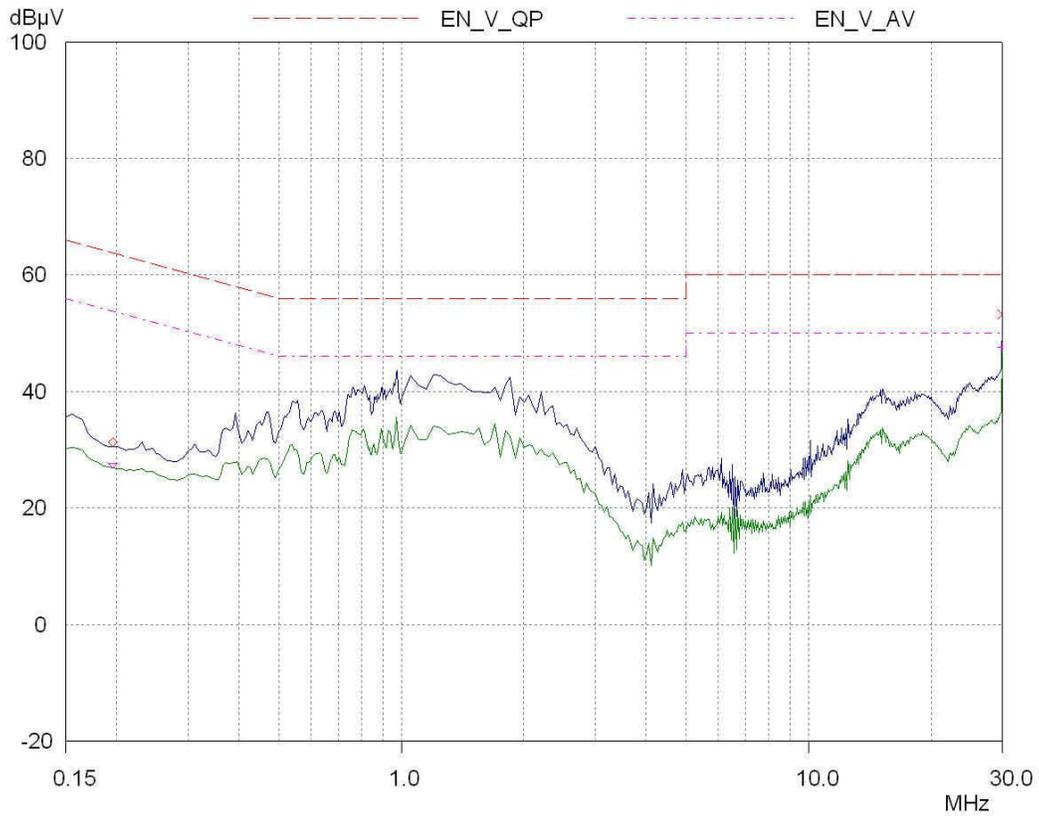
Figure20. EMI test results per EN55022, Class B. 115V<sub>AC</sub> input
