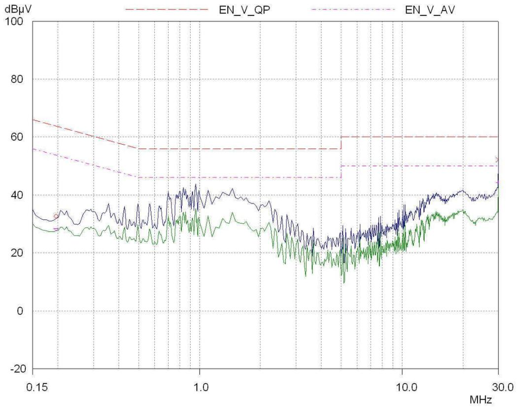
Figure21. EMI test results per EN55022, Class B. 230V<sub>AC</sub> input
