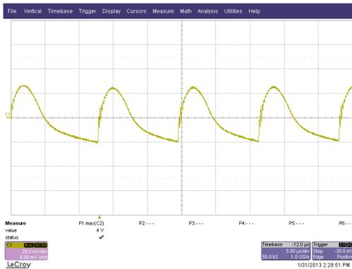
Figure 10 Ripple with 5V,1.2A out 85Vac in 20mV/div 5uS/div
