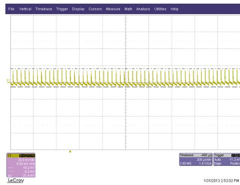
Figure 15 Ripple with 5V,100mA out 265Vac in 20mV/div 500µs/div
