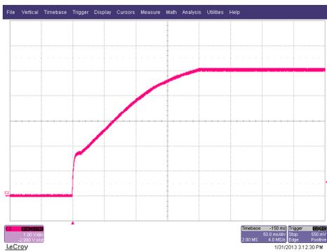
Figure 16 Output voltage start 115Vac,1.2A load 1V/div 50ms/div
