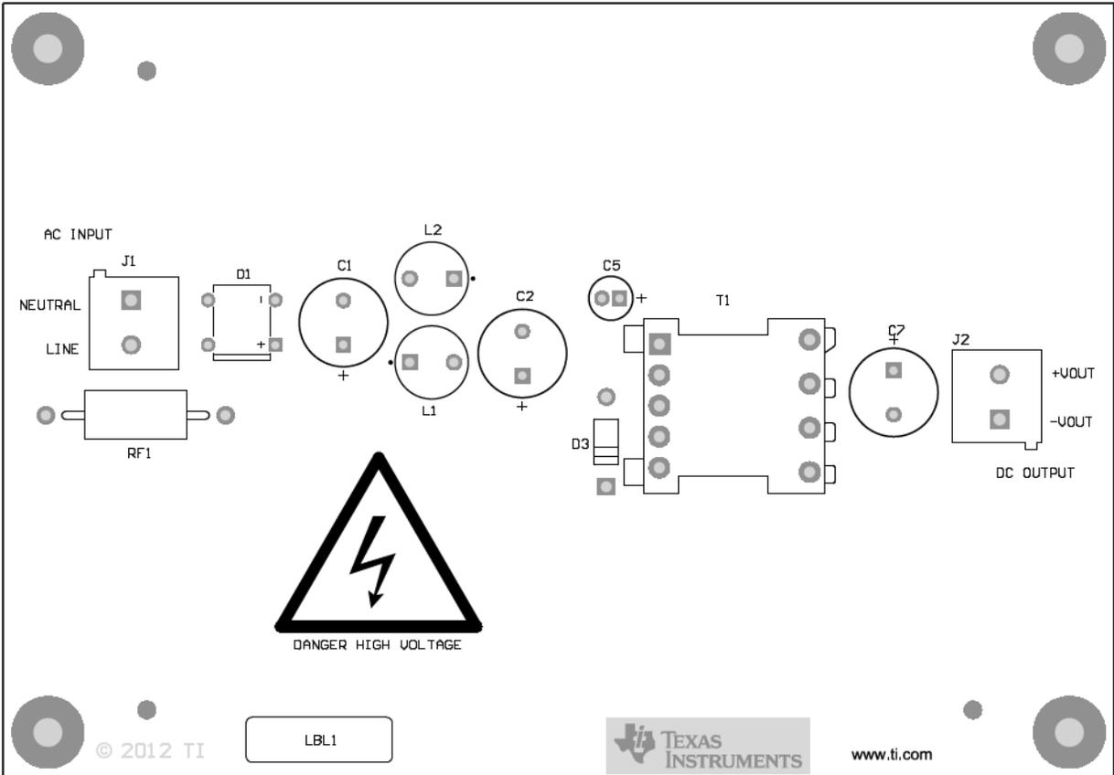
Figure23. Top layer component placement.
