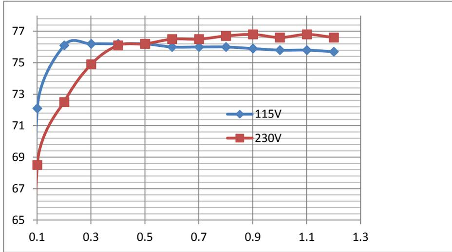
Figure8. Efficiency Vs Iout
