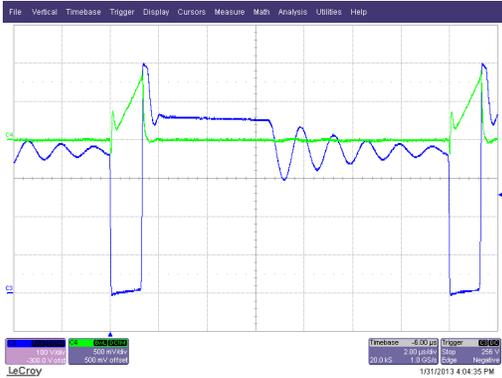
Figure 19 Primary side switching waveforms
