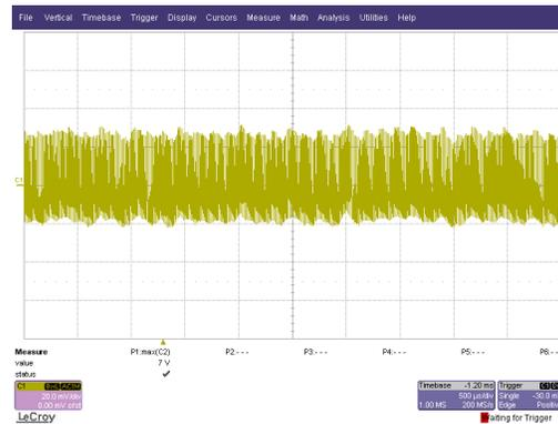
Figure 11 Ripple with 5V,1.2A out 85Vac in 20mV/div 500uS/div
