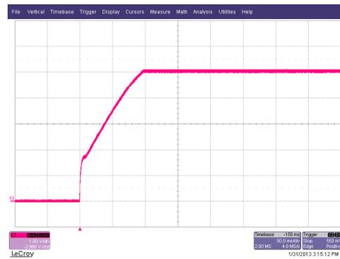
Figure 17 Output voltage start, 230Vac, 1.2A load 1V/div 50ms/div
