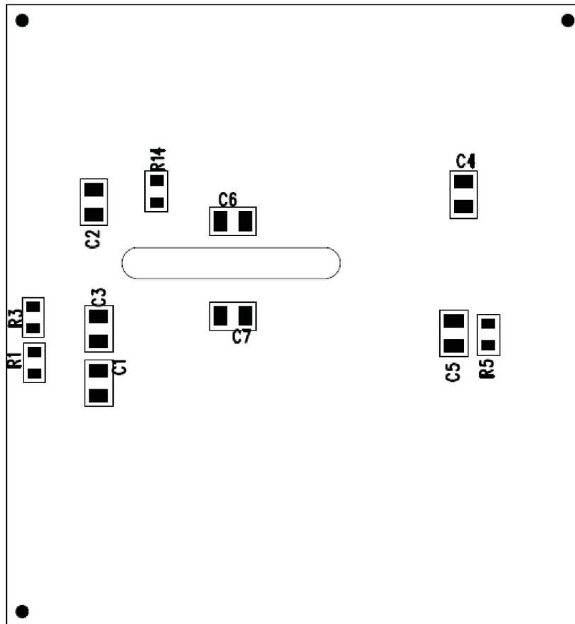
Figure 11. UCC27531EVM-184 Bottom Assembly Drawing (bottom view)
