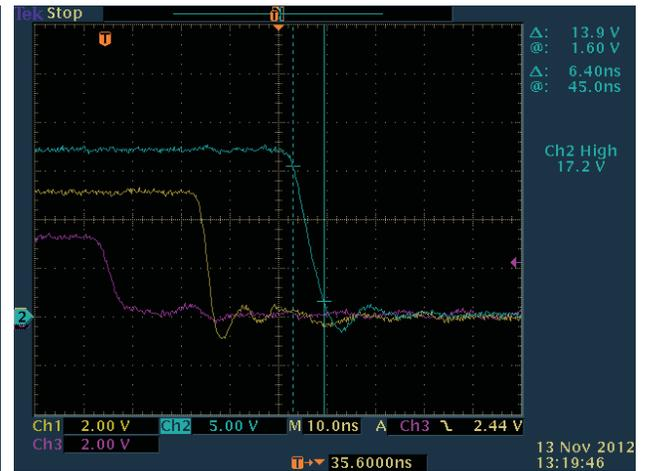
Figure 9. UCC27531DBV Input vs. Output PWM Fall Time
