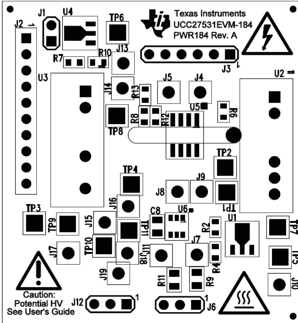
Figure 10. UCC27531EVM-184 Top Layer Assembly Drawing (top view)
