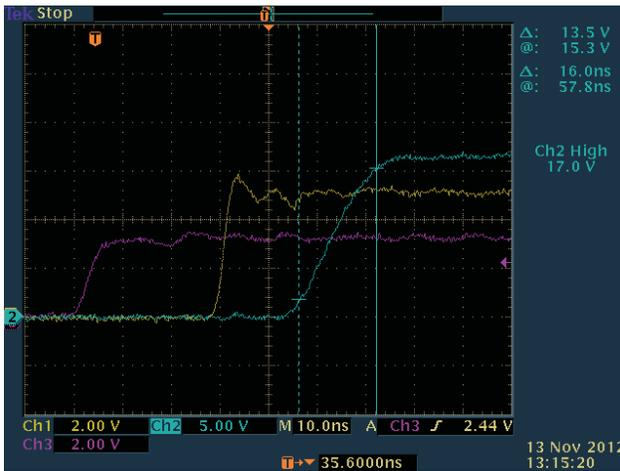
Figure 8. UCC27531DBV Input vs. Output PWM Rise Time
