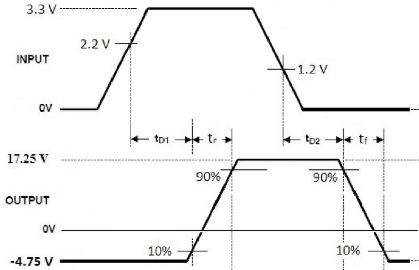
Figure 5. UCC27531EVM-184 Input vs. Output waveforms
