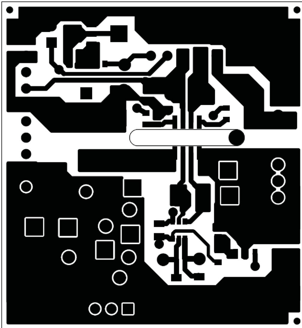
**Figure 12. UCC27531EVM-184 Top Copper (top view)**
