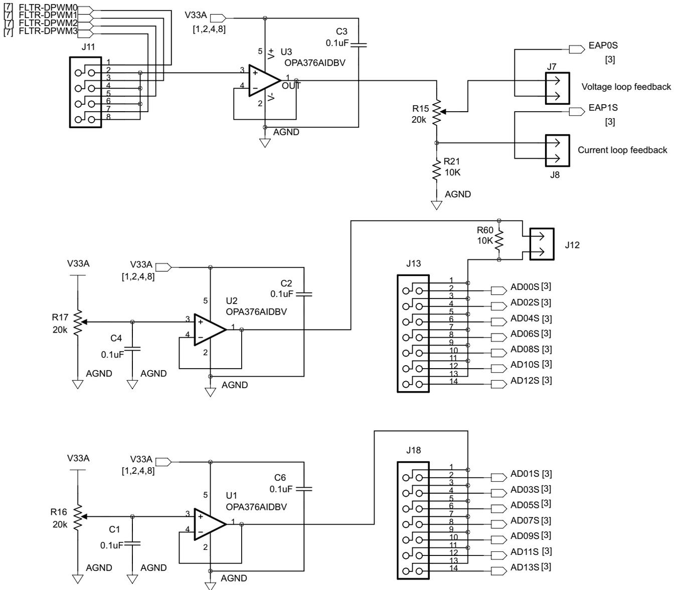
Figure 8. UCD3138OL64EVM-031 Schematics (EADC and ADC12) 8 of 9
