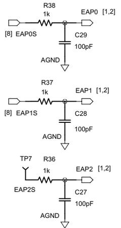
Filter or Address Resistor
