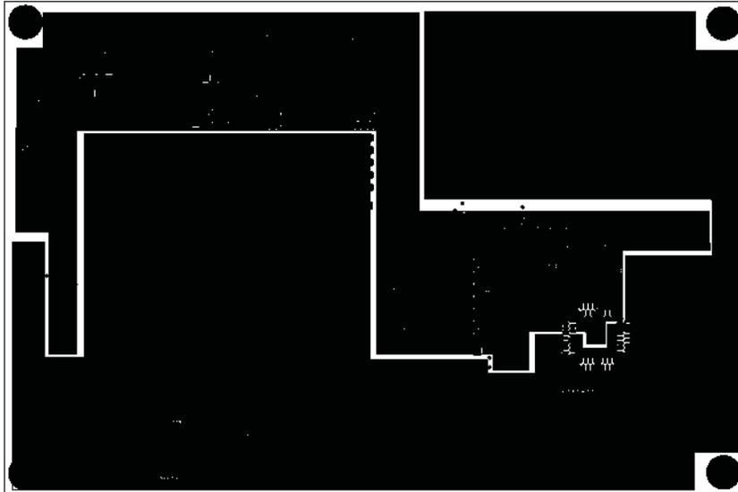
Figure 22. UCD3138OL64EVM-031 Internal Layer 2 (top view)
