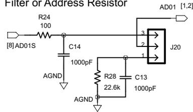
Figure 3. UCD3138OL64EVM-031 Schematics (Filters) 3 of 9
