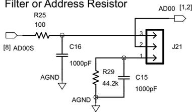
Filter or Address Resistor
