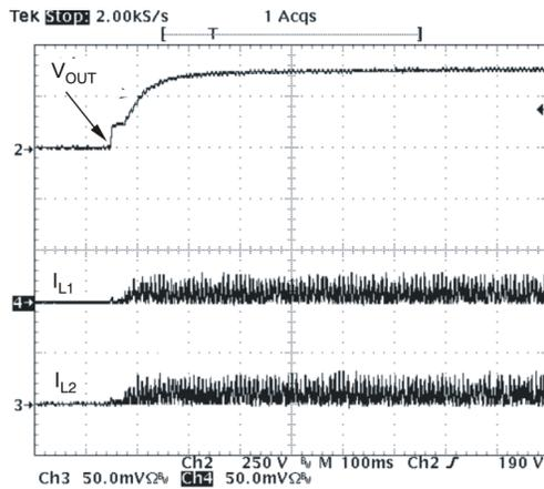
Figure 15. Start-Up at  $V_{IN} = 85 V_{RMS}$ ,  $P_{OUT} = 300 W$
