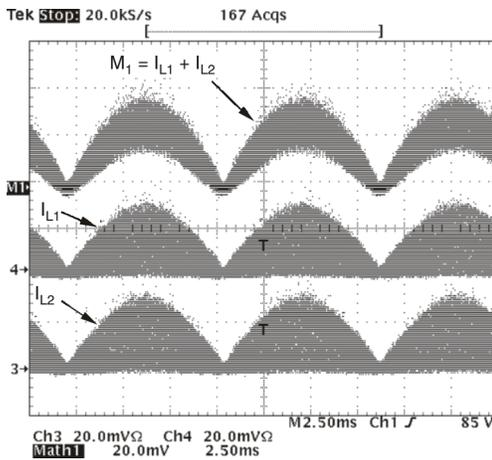
**Figure 13. Inductor and Input Ripple Current at V<sub>IN</sub> = 85 V<sub>RMS</sub>, P<sub>OUT</sub> = 300 W**
