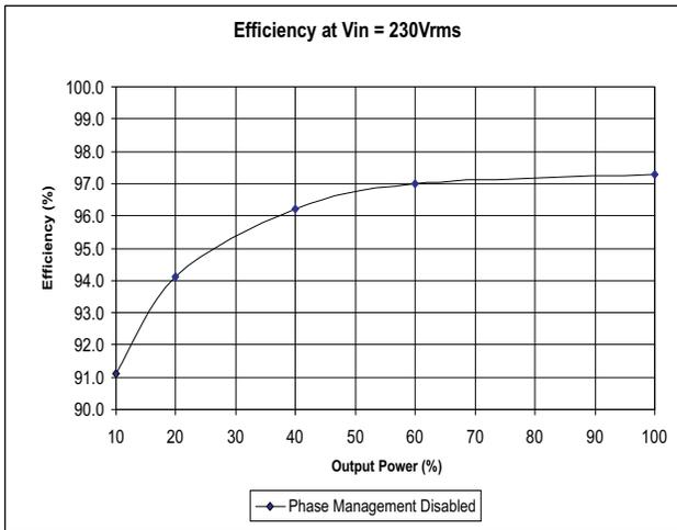
Figure 6. Efficiency at 230 V<sub>RMS</sub>, Without Phase Management
