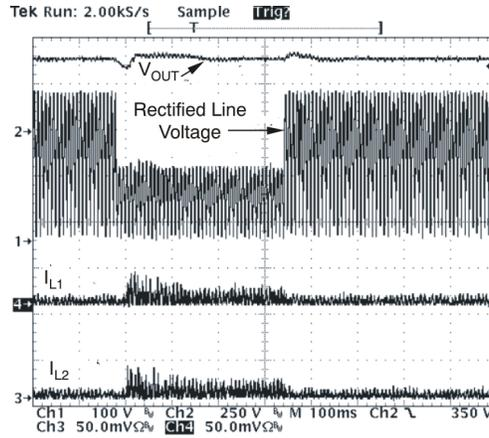
Figure 19. Line Transient, P<sub>OUT</sub> = 300W
