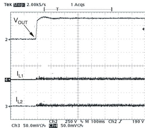
Figure 16. Start-Up at  $V_{IN} = 265 V_{RMS}$ ,  $P_{OUT} = 0 W$
