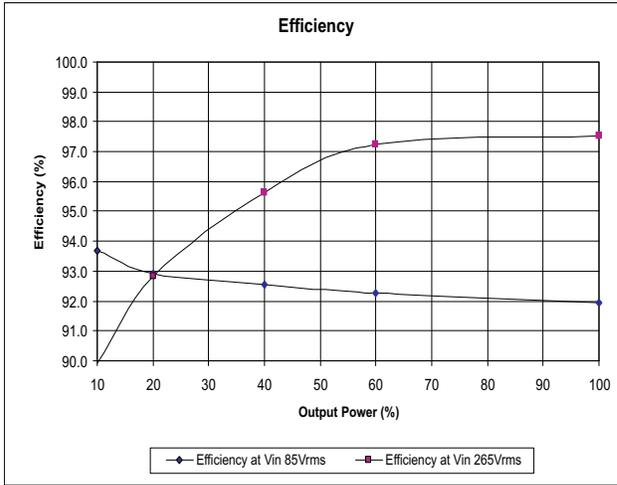
Figure 4. Efficiency at 85 V<sub>RMS</sub> and 265 V<sub>RMS</sub>
