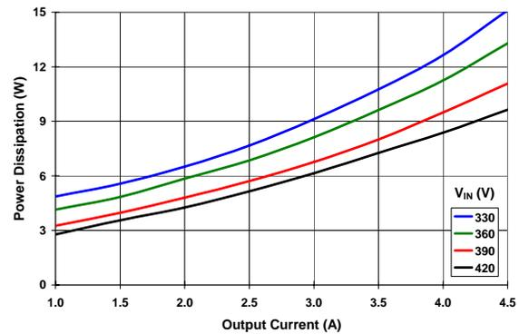
Figure 11 Power Dissipation with MBR1645 Schottky Rectifiers <sup>(1)</sup>
