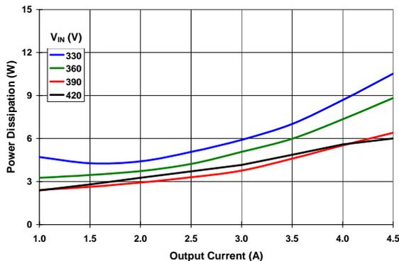
Figure 10 Power Dissipation with UCC24610 Rectifier Controllers and FETs <sup>(1)</sup>
