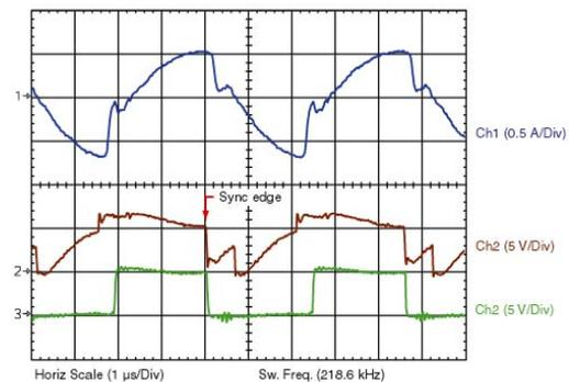
**Figure 19** Upper SR Gate and SYNC Signals at 420-VDC and 3-A Load <sup>(2)</sup>
