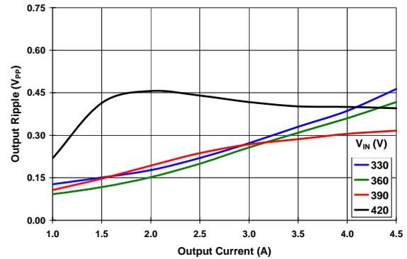
Figure 13 Output AC-Ripple with MBR1645 Schottky Rectifiers <sup>(2), (3)</sup>
