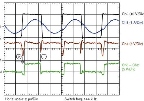
**Figure 25** Upper SR Gate and SYNC Signals at 393-VDC Input and 3-A Load <sup>(4)</sup> ( $f_{SW} \approx f_R$ )
