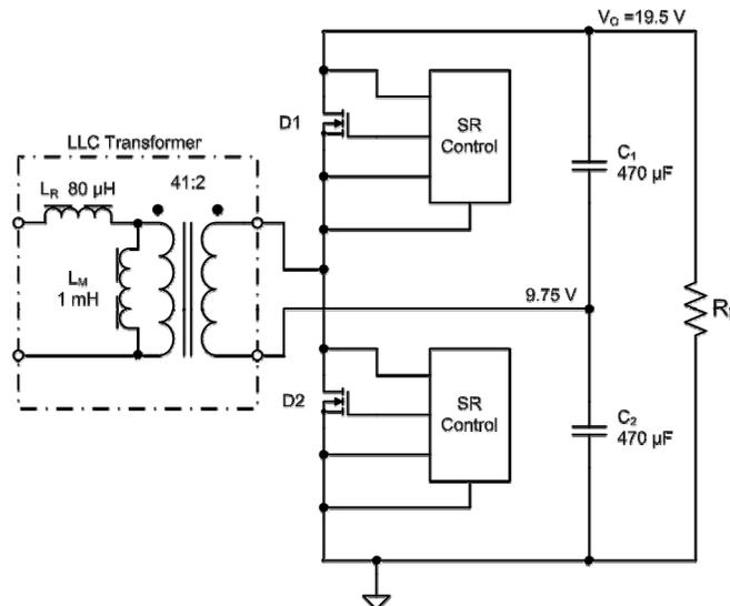
**Figure 2 Voltage-Doubling Rectifier Circuit with Synchronously Switched MOSFETs**
