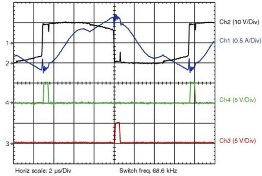
**Figure 27 Upper and Lower SR Gate Signals at 340-VDC Input and 1-A Load <sup>(5)</sup>**
