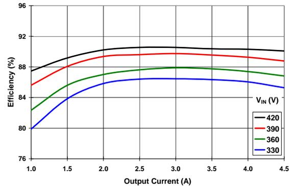
Figure 9 Operating Efficiency with MBR1645 Schottky Rectifiers
