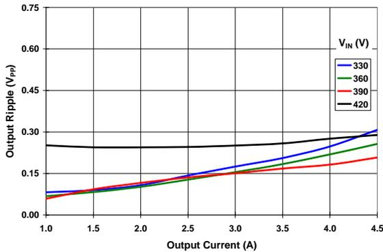
Figure 12 Output AC-Ripple with UCC24610 Rectifier Controllers and FETs <sup>(2)</sup>
