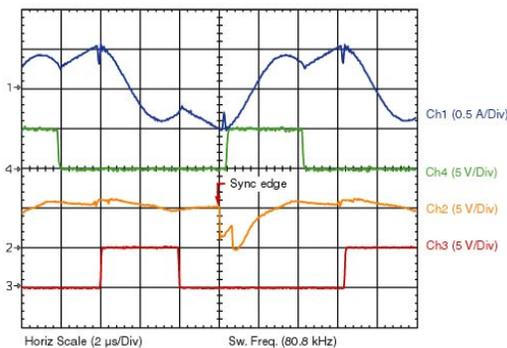
**Figure 18** Upper/Lower SR Gate and Lower SYNC Signals at 340-VDC Input and 1-A Load <sup>(1)</sup>
