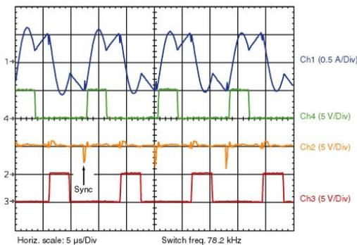
**Figure 24** Upper/Lower SR Gate and Lower SYNC Signals at 340-VDC Input and 1-A Load <sup>(3)</sup>
