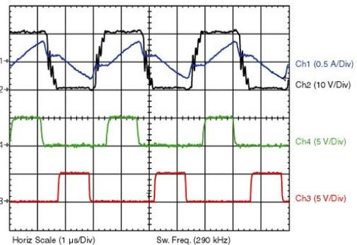
**Figure 17** Upper and Lower SR Gate Signals at 420-VDC Input and 1-A Load ( $f_{SW} > f_R$ )
