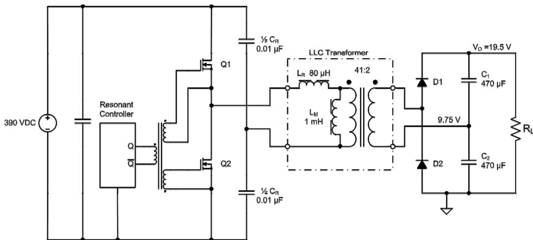
**Figure 1 LLC Series-Resonant Converter**
