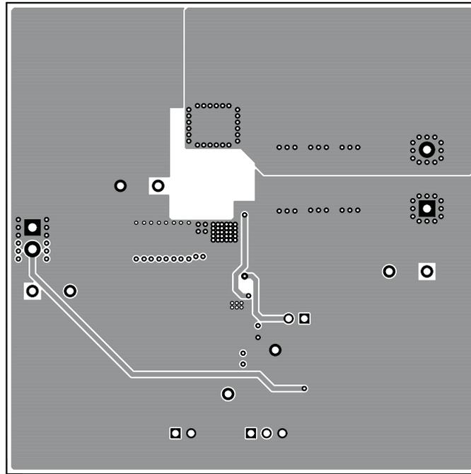
**Figure 15. CSD86350Q5DEVM-604 Internal Copper Layer 1 (X-Ray Top View)**
