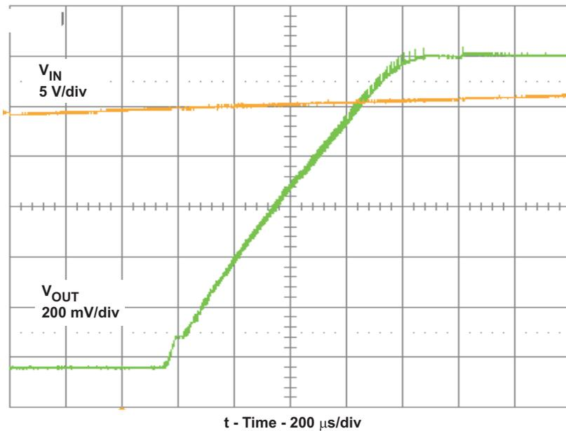
$V_{IN} = 12V$ ,  $V_{OUT} = 1.2V$ ,  $I_{OUT} = 25A$
