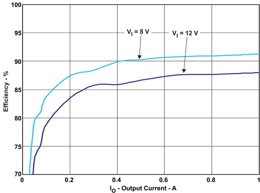
$V_{IN} = 8V$  &  $12V$ ,  $V_{OUT} = 1.2V$ , MODE = GND, no airflow
