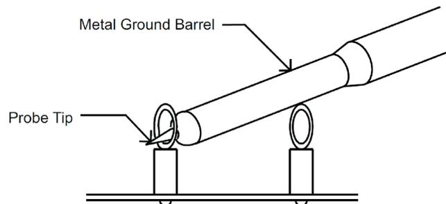
Figure 3. Tip and Barrel Technique
