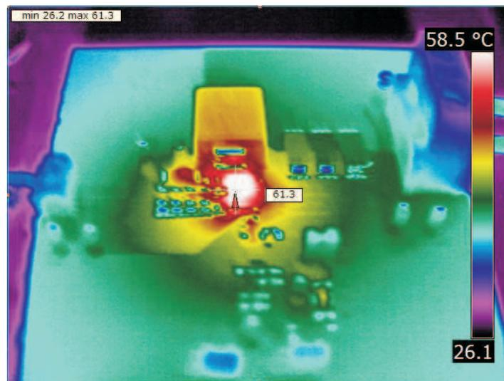
$V_{IN} = 12V, V_{OUT} = 1.2V, I_{OUT} = 25A, \text{no air flow}$
