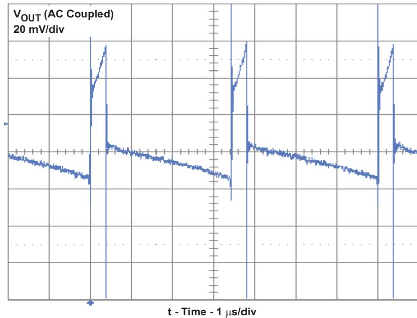
$V_{IN} = 12V$ ,  $V_{OUT} = 1.2V$ ,  $I_{OUT} = 25A$ , measured at TP7 and TP8 using the tip and barrel measurement technique shown in Figure 3. Since the probe picks up substantial radiated noise, this method is not recommended to measure the output voltage ripple.
