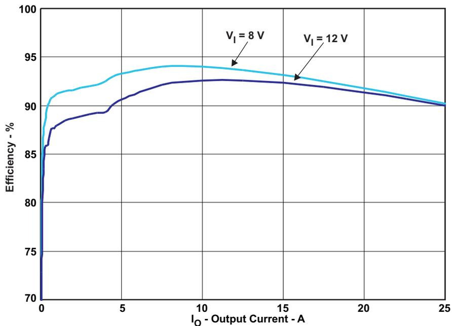
$V_{IN} = 8V$  &  $12V$ ,  $V_{OUT} = 1.2V$ , MODE = GND, no airflow
