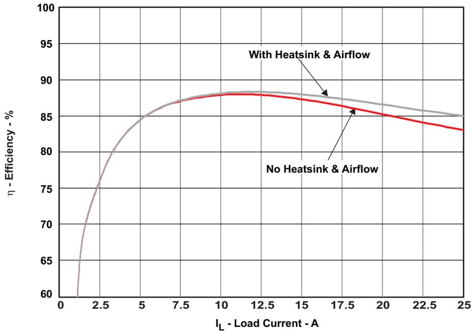
With and without a heatsink at  $V_{IN} = 12V$ ,  $V_{OUT} = 1.2V$ ,  $I_{OUT} = 0A - 25A$
