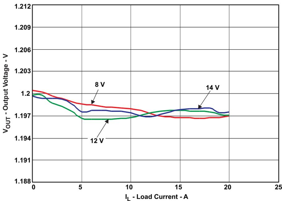
$V_{IN} = 8V - 14V$ ,  $V_{OUT} = 1.2V$ ,  $I_{OUT} = 0A - 20A$
