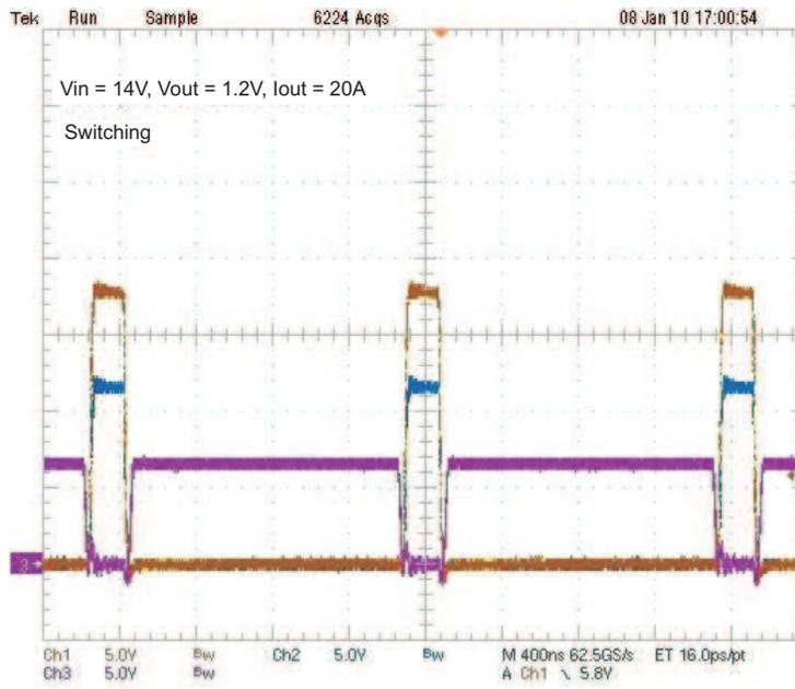
$V_{IN} = 12V, V_{OUT} = 1.2V, I_{OUT} = 20A$
