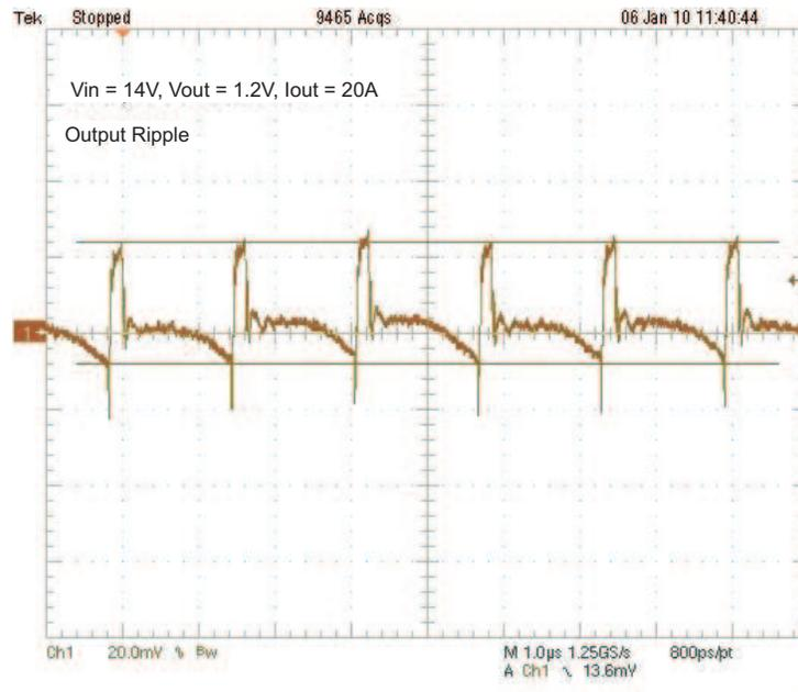
$V_{IN} = 14V, V_{OUT} = 1.2V, I_{OUT} = 20A$
