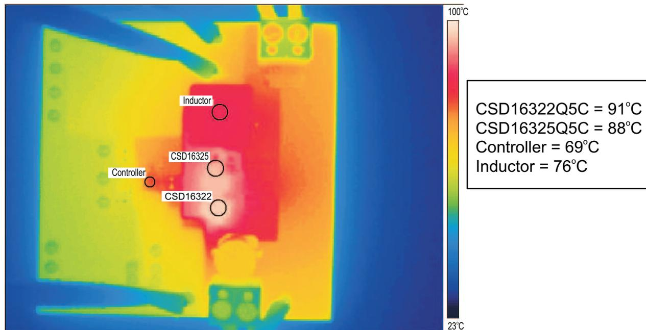
$V_{IN} = 12V$ ,  $V_{OUT} = 1.2V$ ,  $I_{OUT} = 20A$
