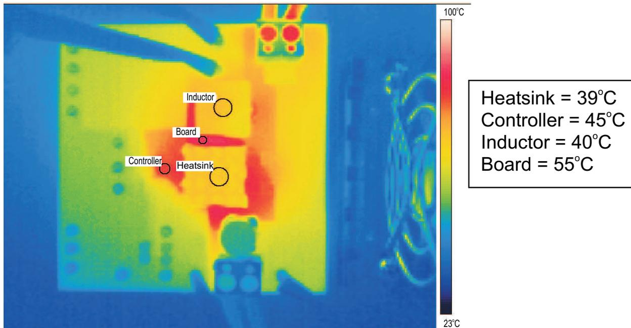
$V_{IN} = 12V$ ,  $V_{OUT} = 1.2V$ ,  $I_{OUT} = 25A$
