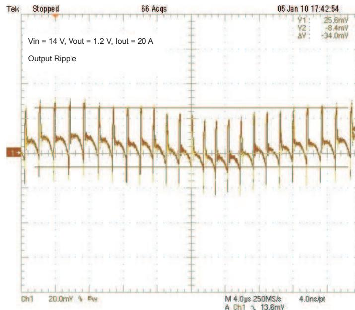
Figure 12. CSD163CEVM-591 Output Ripple with FSS Enabled
