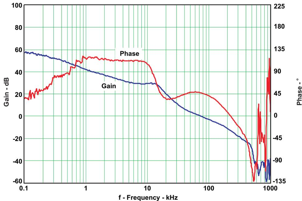
$V_{IN} = 14V$ ,  $V_{OUT} = 1.2V$ ,  $I_{OUT} = 20A$ , Bandwidth: 73kHz, Phase Margin: 47°
