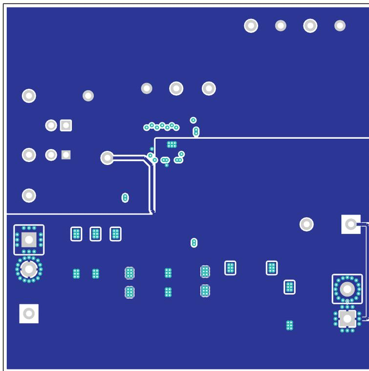
Figure 17. CSD163CEVM-591 Internal 1 (X-Ray Top View)
