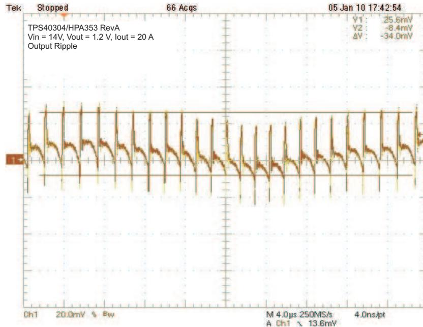
Figure 10. TPS40304EVM-353 Output Ripple with FSS Enabled
