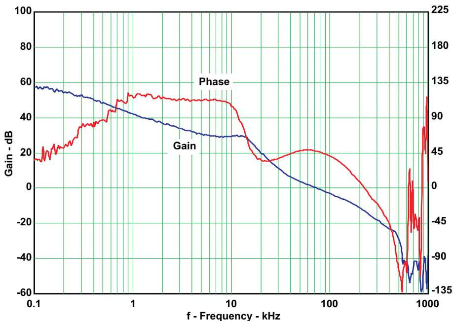
$V_{IN} = 14V$ ,  $V_{OUT} = 1.2V$ ,  $I_{OUT} = 20A$ , Bandwidth: 73kHz, Phase Margin: 47°
