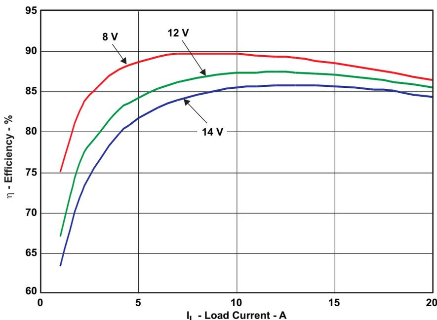
$V_{IN} = 8.0V - 14V$ ,  $V_{OUT} = 1.2V$ ,  $I_{OUT} = 0A - 20A$
