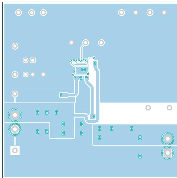
**Figure 16. TPS40304EVM-353 Internal 2 (X-Ray Top view)**
