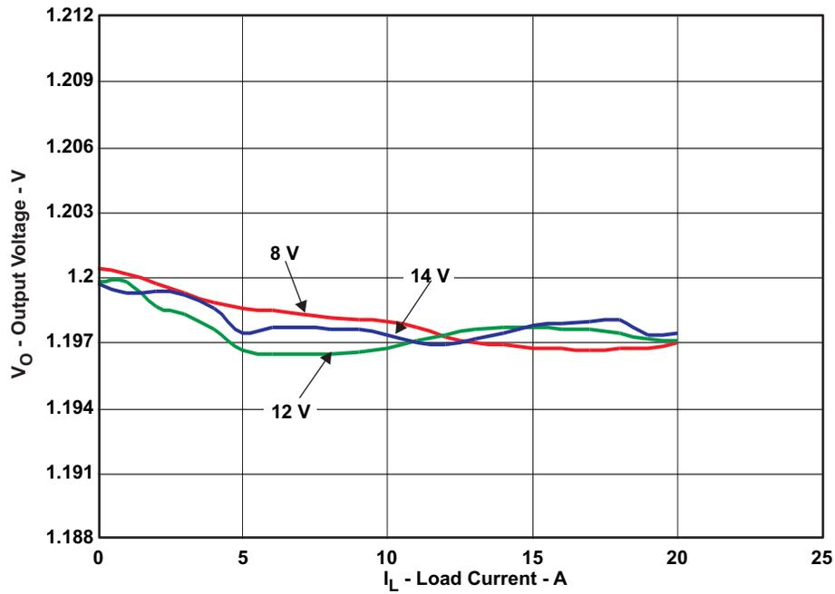
$V_{IN} = 8.0V - 14V$ ,  $V_{OUT} = 1.2V$ ,  $I_{OUT} = 0A - 20A$
