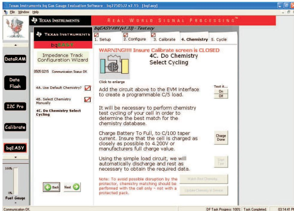
Figure 18. Chemistry Cycling Test
