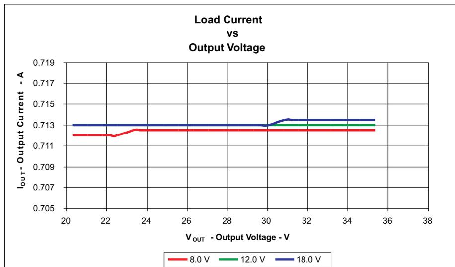
Figure 5. TPS40211EVM-352 Load Current versus Output Voltage
