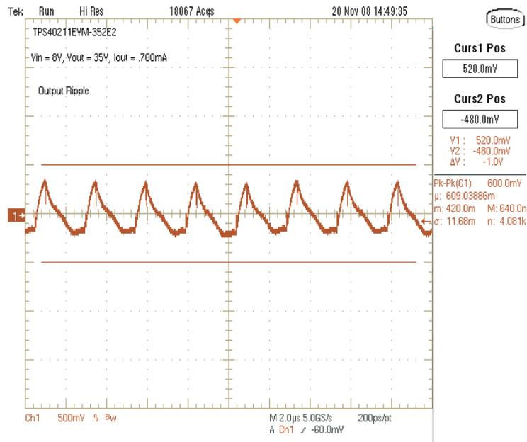
**Figure 6. TPS40211EVM-352 Output Voltage Ripple**
