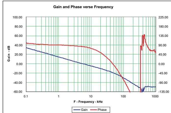
**Figure 8. TPS40211EVM-352 Gain and Phase versus Frequency**
