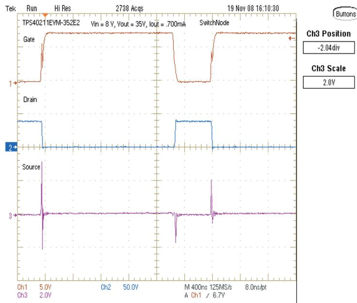
**Figure 7. TPS40211EVM-352 Switching Waveforms**
