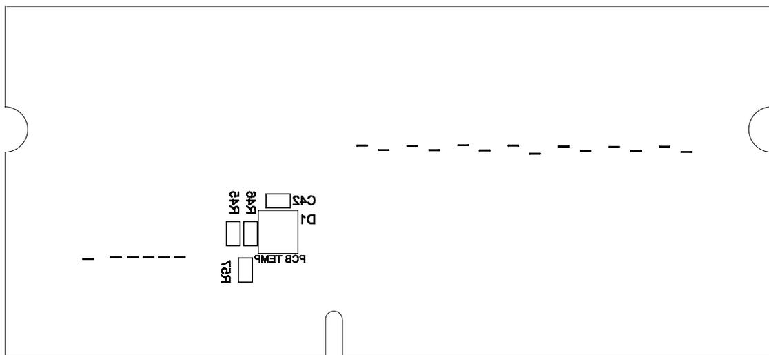
Figure 13. DIMM Bottom Silk Screen with Outlines
