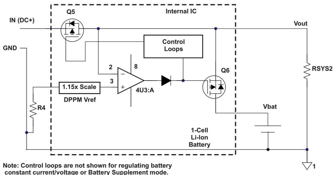
Figure 1. DPPM – Manages Battery Current Based on Output Voltage
