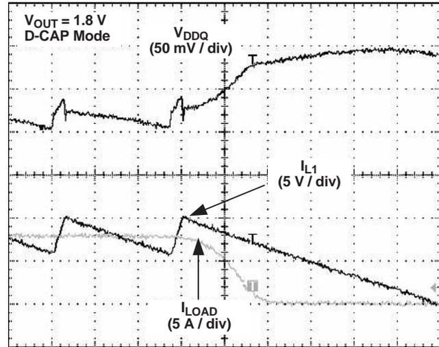
**Figure 6. TPS51116EVM - 8-A to 0-A Load Transient Response**
