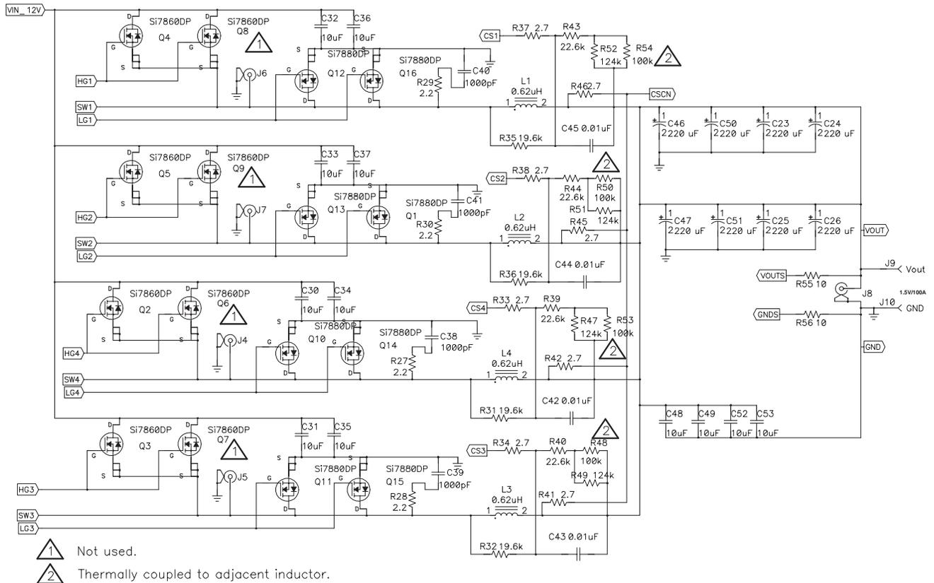
Figure 3. TPS40090EVM-002 Schematic Part 3 – Power Stage
