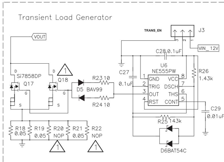
Figure 2. TPS40090EVM-002 Schematic Part 2 – Driver Circuit and Load Transient Generator
