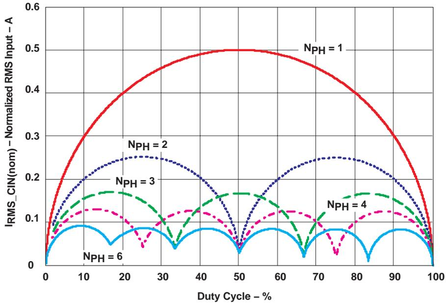
Figure 4. Input Ripple Current RMS Value Overload Current
