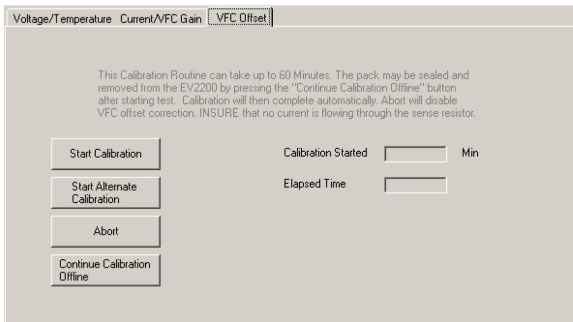
**Default VFC Offset:** To select this offset method click on | Start Calibration |. This method will apply an internal short (inside the bq2060) across the sense resistor. With the sense resistor shorted inside the bq2060 there is less chance that an external current can cause a poor offset calculation. This method does not compensate for slight offsets induced by the circuit board.
