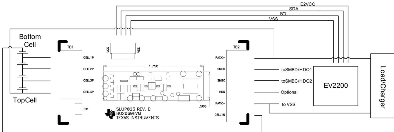
Figure 5-2. Circuit Module Connection to NiMH Cells and System Load/Charger
