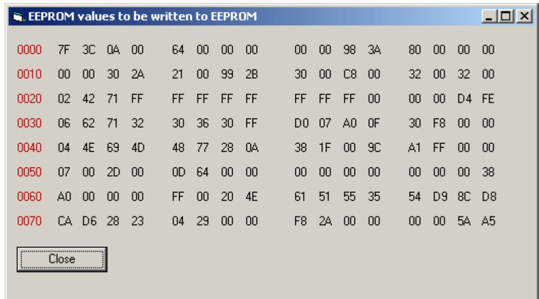
All data required for calibration is also held in the EEPROM for the bq2060, as highlighted in the following figure.
