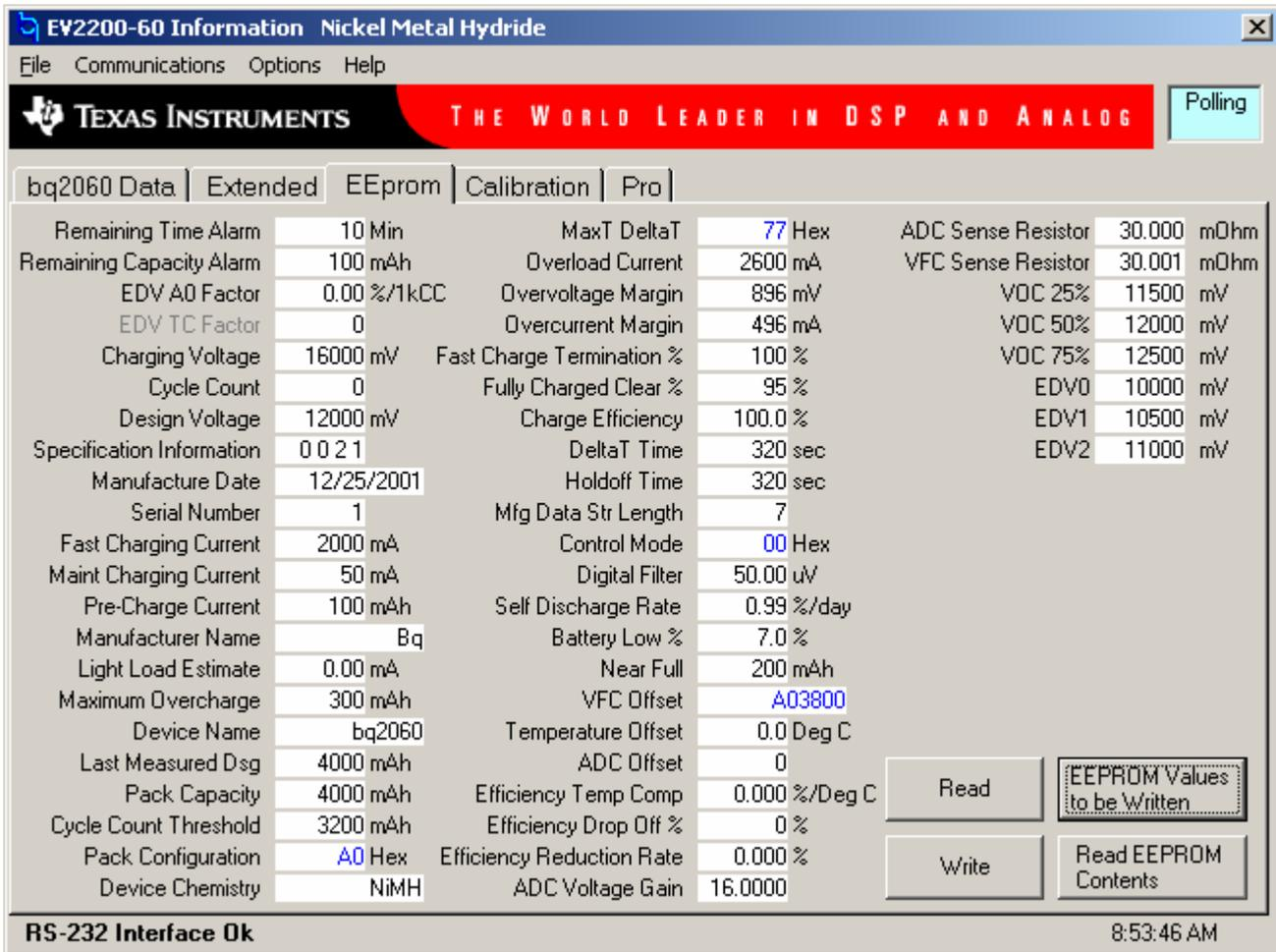
To read all the data from the bq2060 EEPROM, click on | Read |. To write to a selected location click on the desired location, type in the desired data, and hit the ENTER key. After a moment the next location will be highlighted. The entire EEPROM can be written this way.
