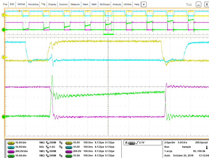
Figure 8-6. SiC MOSFET Switching Waveforms
