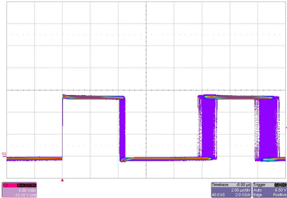
The photo below shows the switch node voltage (TP6) of the 82V converter. The dithering circuit has been disabled. The outputs were loaded to max loads.  $V_{in} = 14V$ . (5V/DIV, 2 $\mu$ S/DIV)
