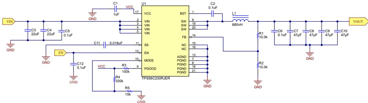
Figure 1-1. TPS56C230 Typical Application Schematic
