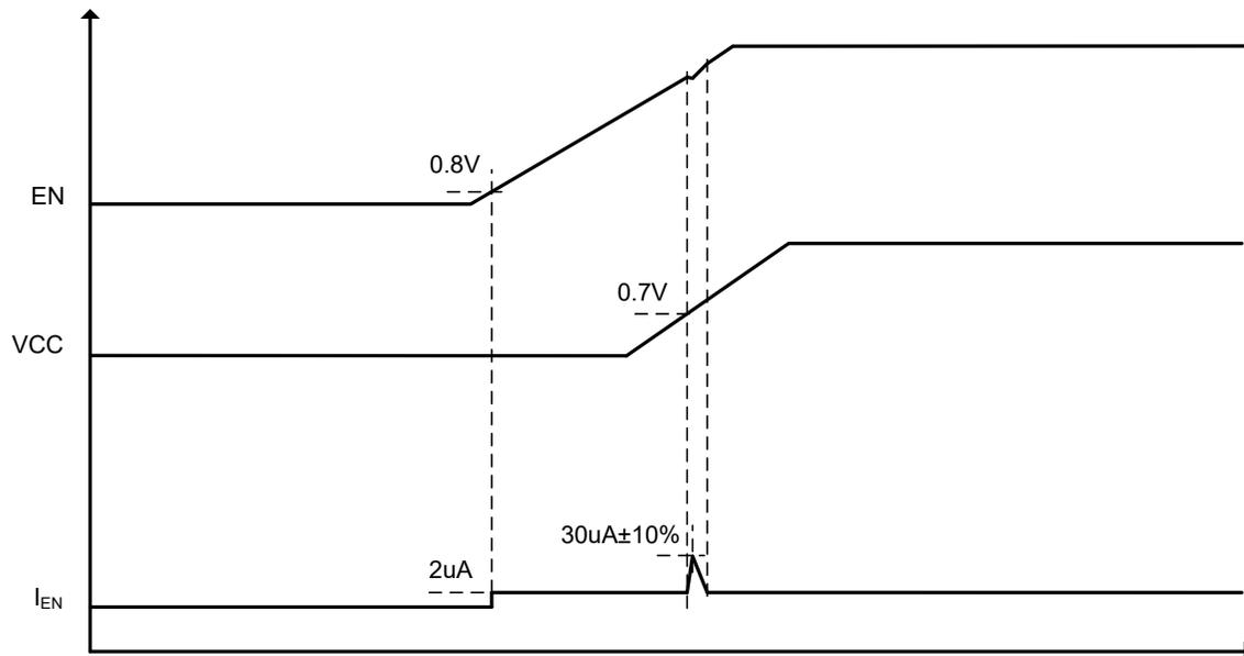
Figure 3-1. EN Internal Pull-down Current
