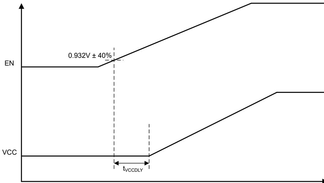
Figure 2-1. EN to VCC Start-up Delay
