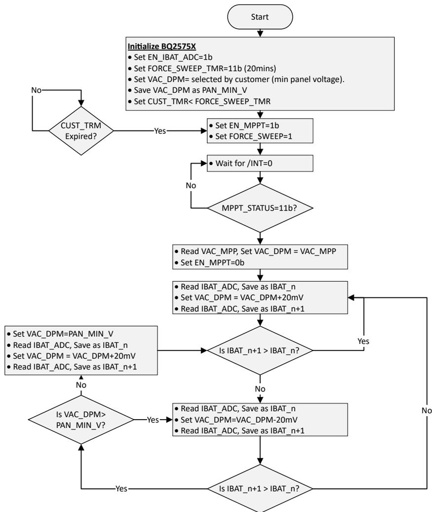
**Figure 3-2. External P&O MPPT Control Algorithm for BQ2575x**
