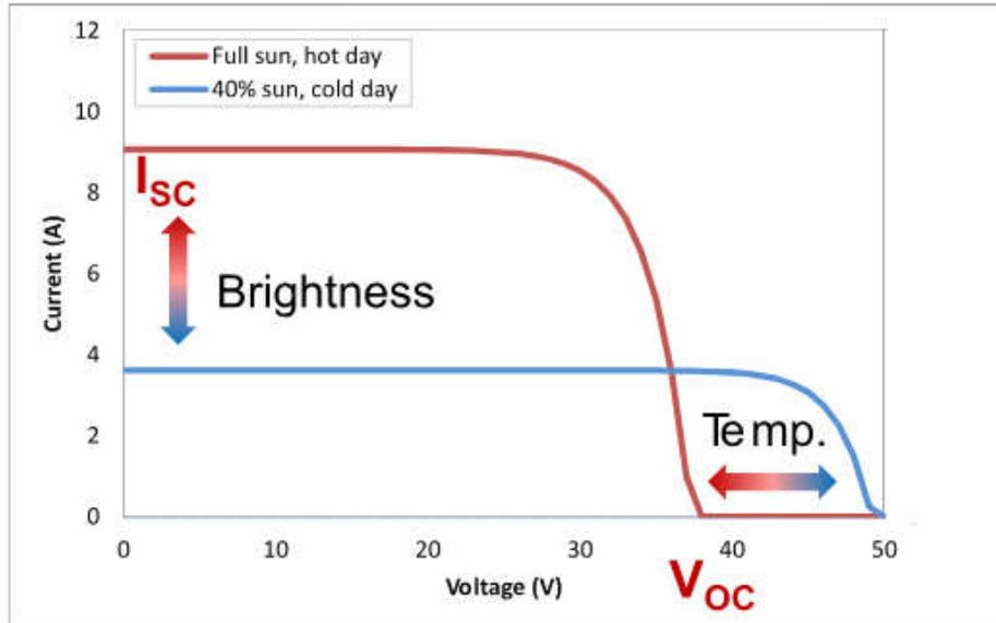
**Figure 1-1. Excellent Solar PV Operating Curves**
