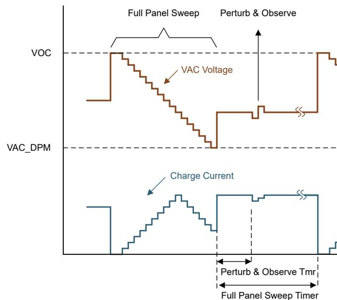
**Figure 3-1. External P&O MPPT Algorithm Operation**
