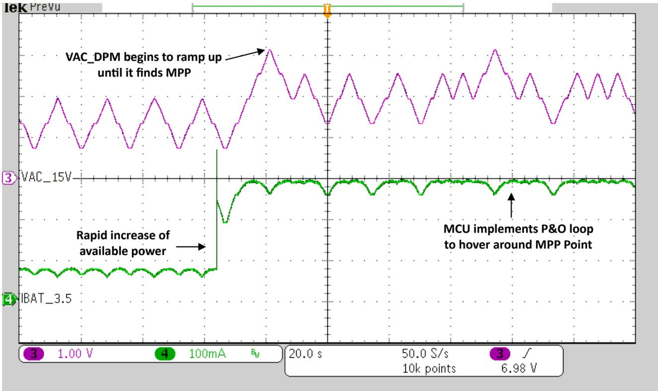
Figure 4-2. P&O MPPT Response to Sudden Increase in Available Solar Power
