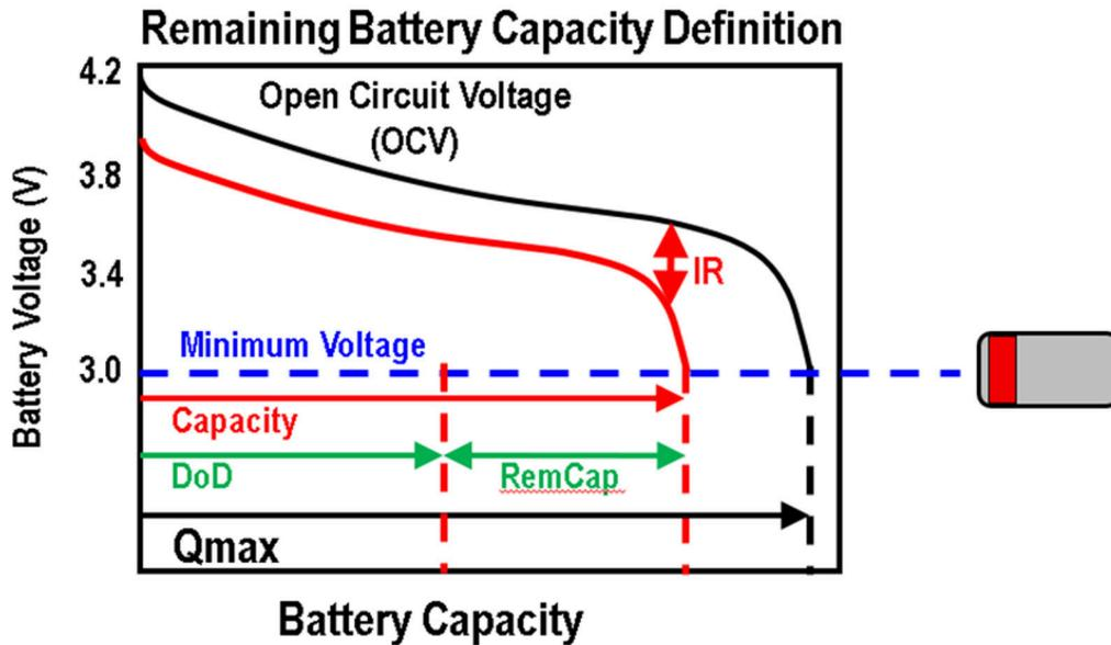
Figure 4-1. Remaining Capacity Prediction
