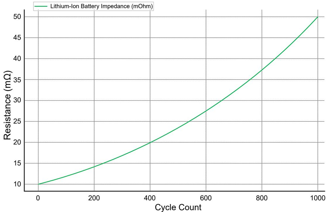
**Figure 3-2. Battery Resistance vs. Age**
