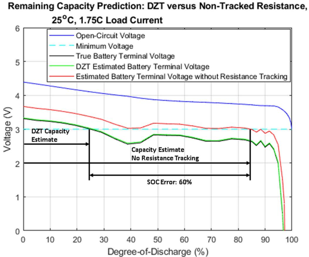
**Figure 6-2. Remaining Capacity Estimation Comparison: Dynamic Z-Track™ vs. No Resistance Update, 1.75 C Load**
