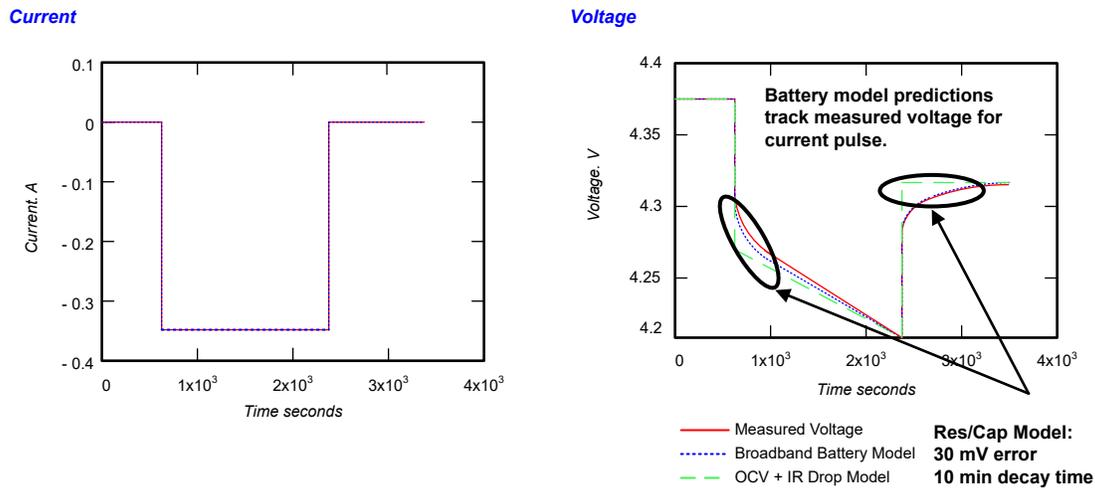
**Figure 5-1. Battery Transient Response**
