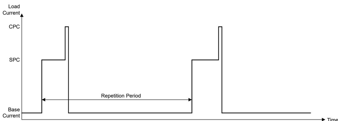
**Figure 2-1. Dynamic Battery Power Technology Example Load Current**
