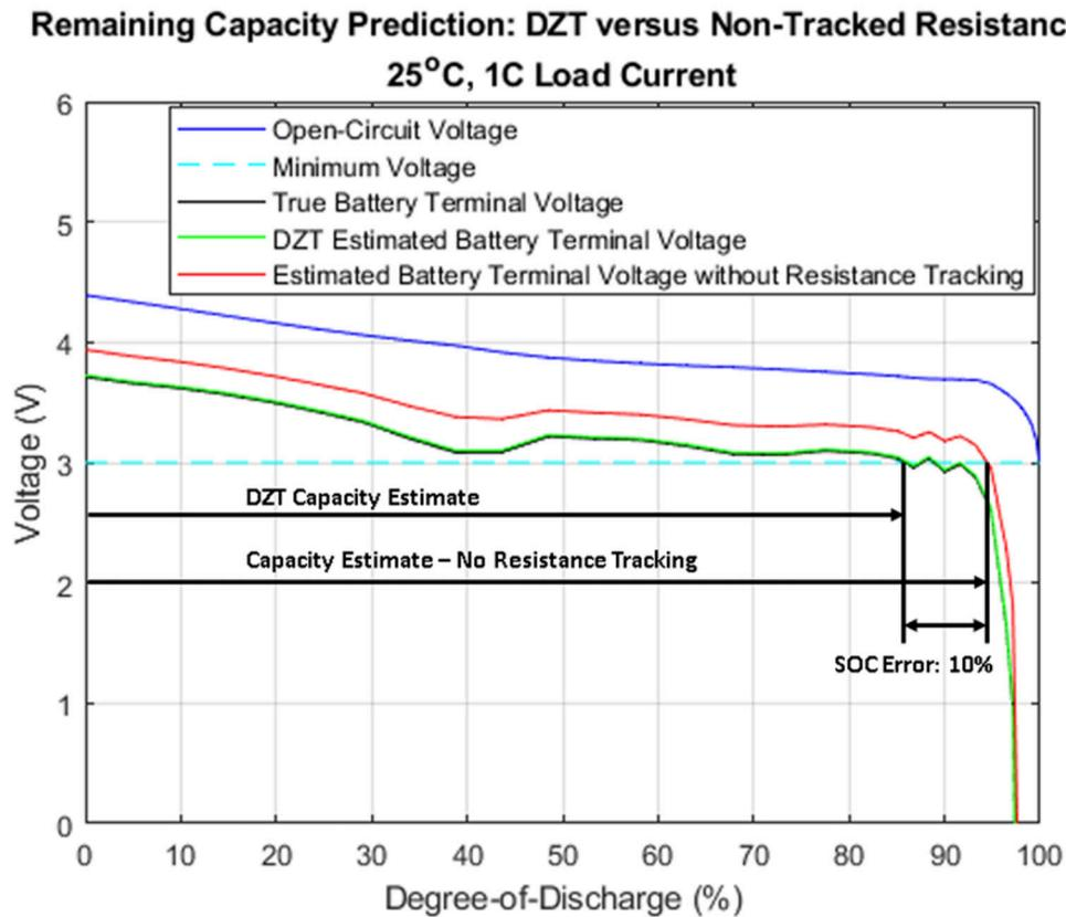
**Figure 6-1. Remaining Capacity Estimation Comparison: Dynamic Z-Track™ vs. No Resistance Update, 1C Load**
