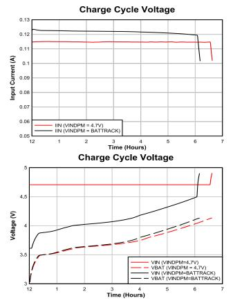
A higher charge current is achievable, resulting in a faster charge cycle and shorter charge duration. One additional benefit that can be calculated from the charge cycle characteristics is the improvement in efficiency. With less energy dissipated as heat, the charging process provides a charging with less heat concerns.
