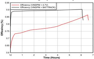
Using Battery Tracking VINDPM to Make the Most of Solar and High-Impedance Power Sources
