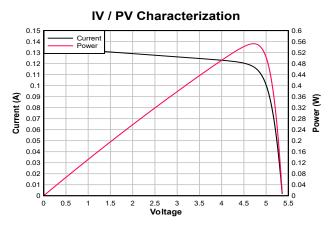
From the described characteristics, one can observe that the maximum power-point voltage can be found at approximately 4.75V. With this, the previously
