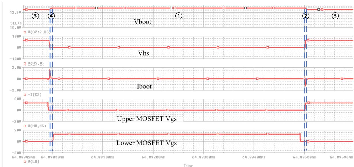
**Figure 3-6. Simulation Results (D=50%,  $C_{boot}$ =100nF)**
