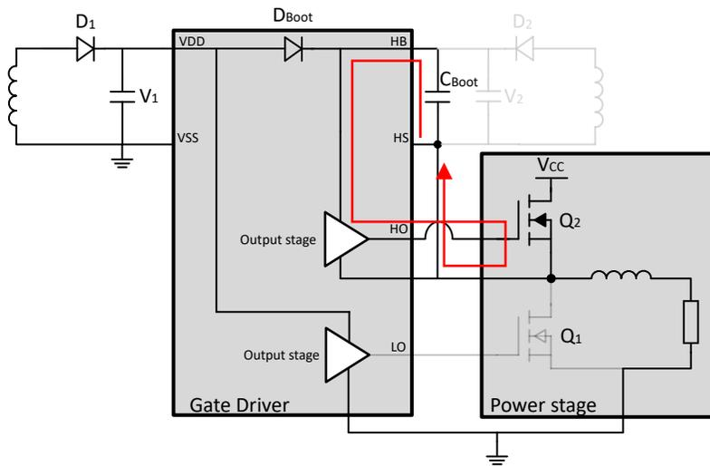
Figure 3-5. Equivalent Circuit in Mode 3
