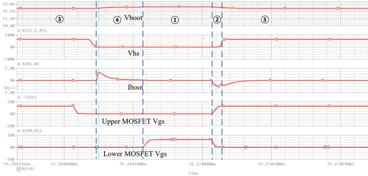
**Figure 3-7. Simulation Results (D=99%,  $C_{boot}=100nF$ )**
