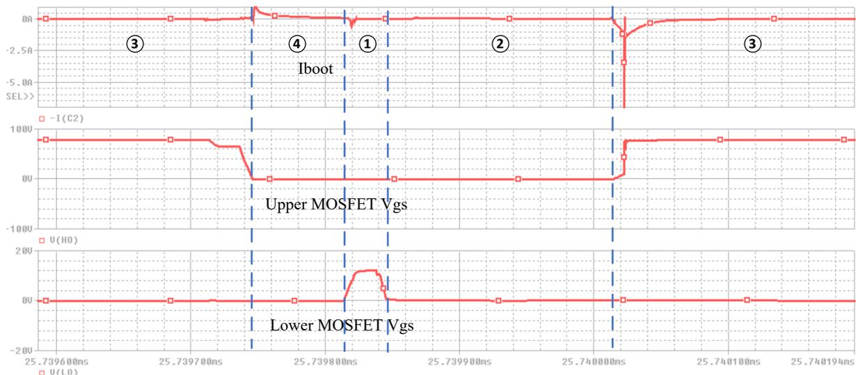
**Figure 3-8. Simulation Results (D=99% With Reverse Recovery Characteristic)**
