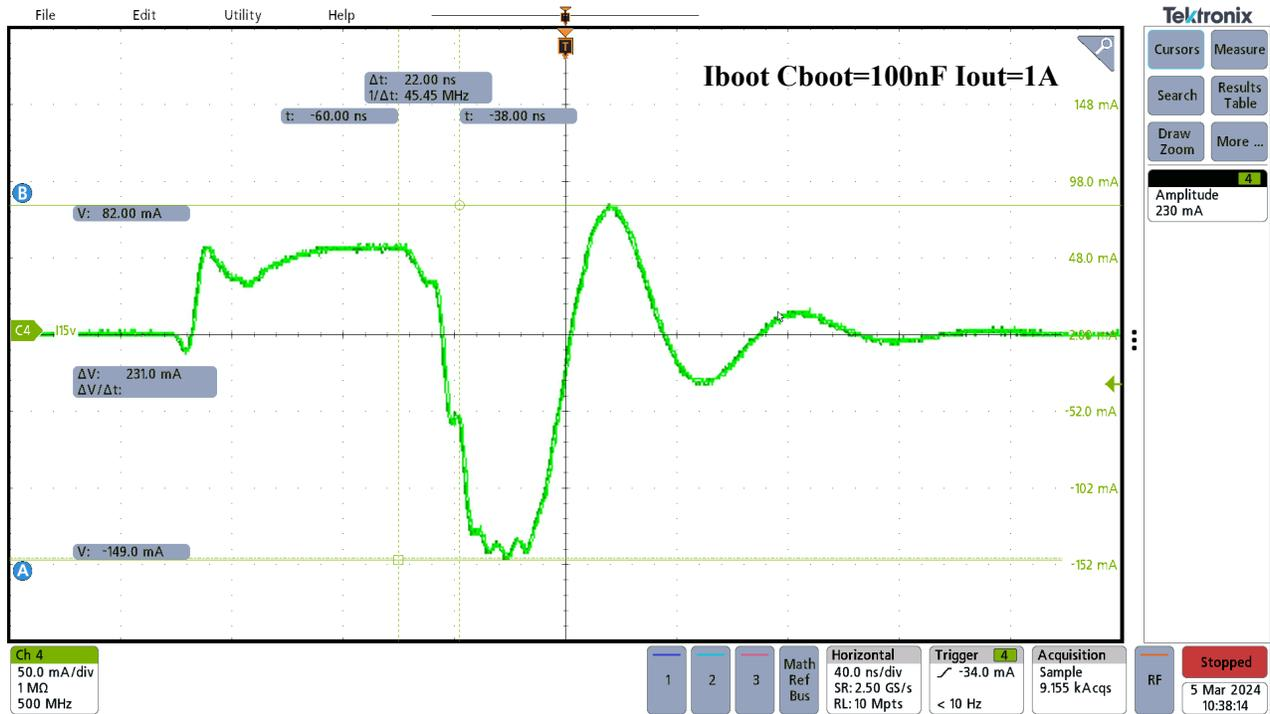
Figure 3-12. Experiment Results (100nF Bootstrap Capacitor)
