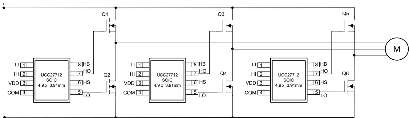
**Figure 3-1. Three-Phase Inverter Motor Drive with UCC27712**
