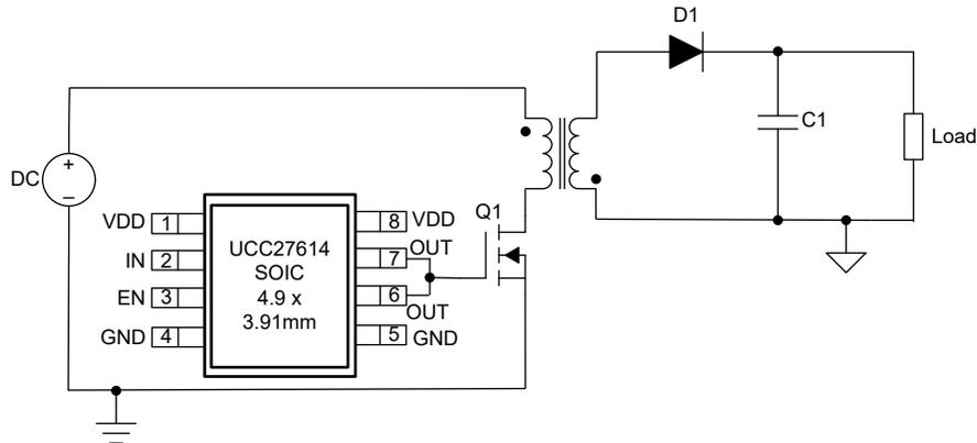
**Figure 4-2. Flyback Converter with UCC27614**
