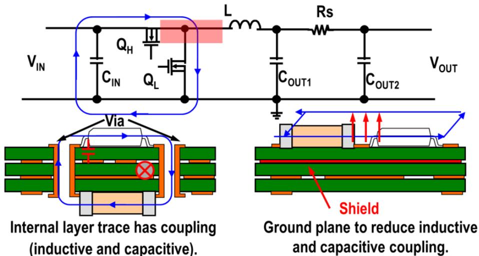
Figure 2-2. Power Stage Component Placement and Ground Layer
