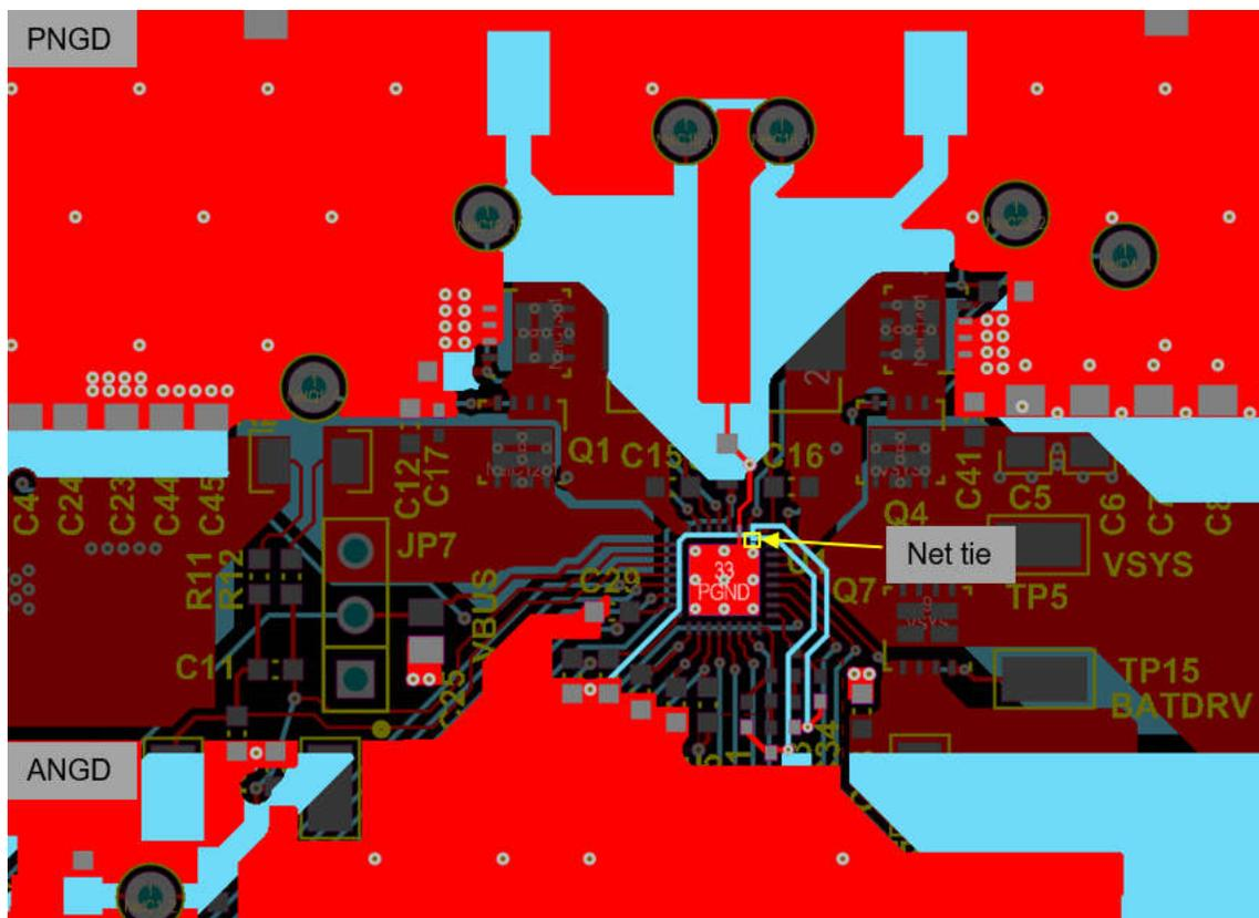
**Figure 2-8. Separating AGND and PGND With Net-Tie**
