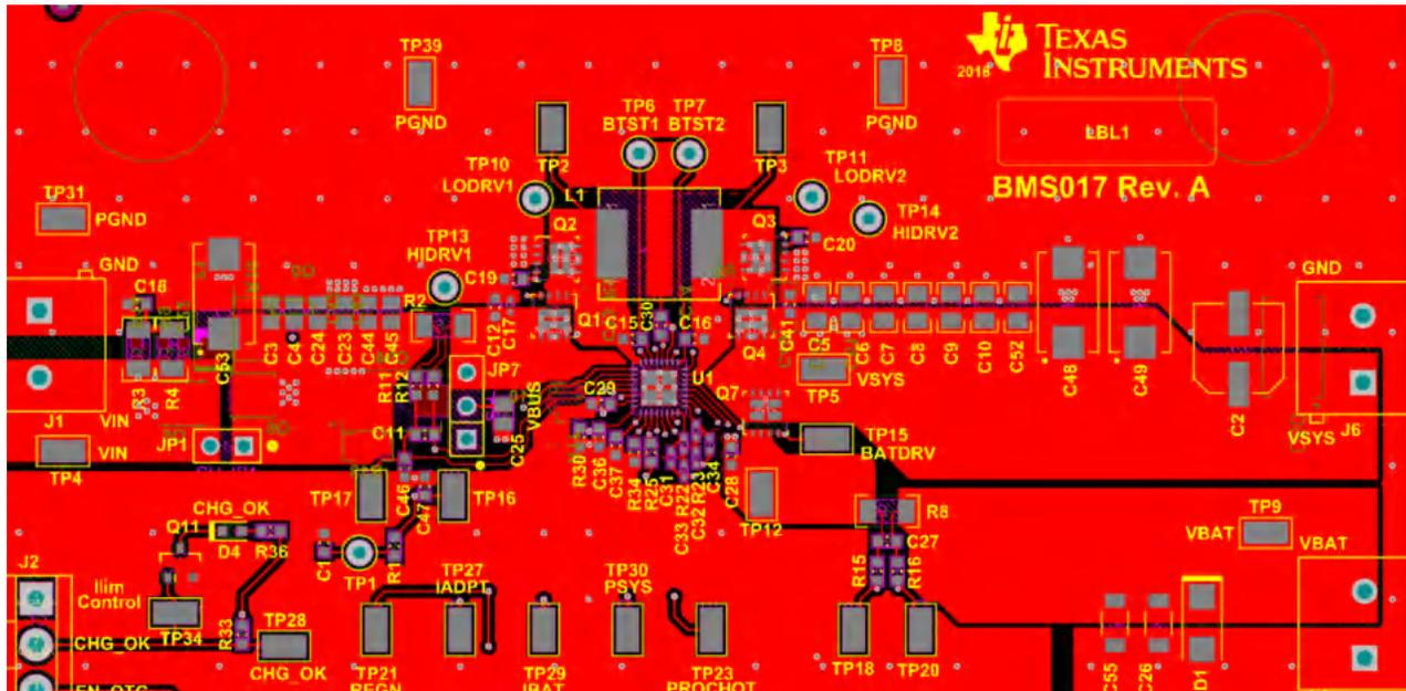
**Figure 2-4. Power Components Placement on Top Layer**
