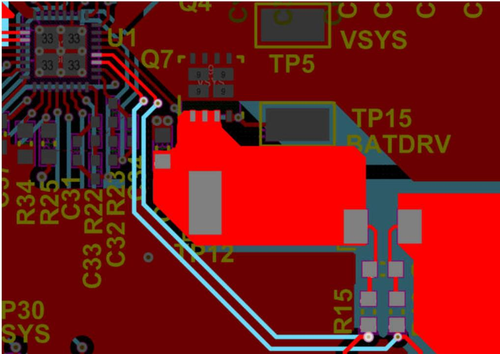
Figure 2-5. Kelvin Sensing Connections for  $R_{SR}$  Resistor
