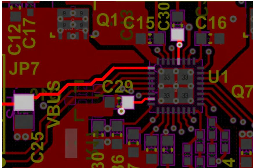
**Figure 2-6. Capacitors Placement for VBUS, VDDA, REGN**
