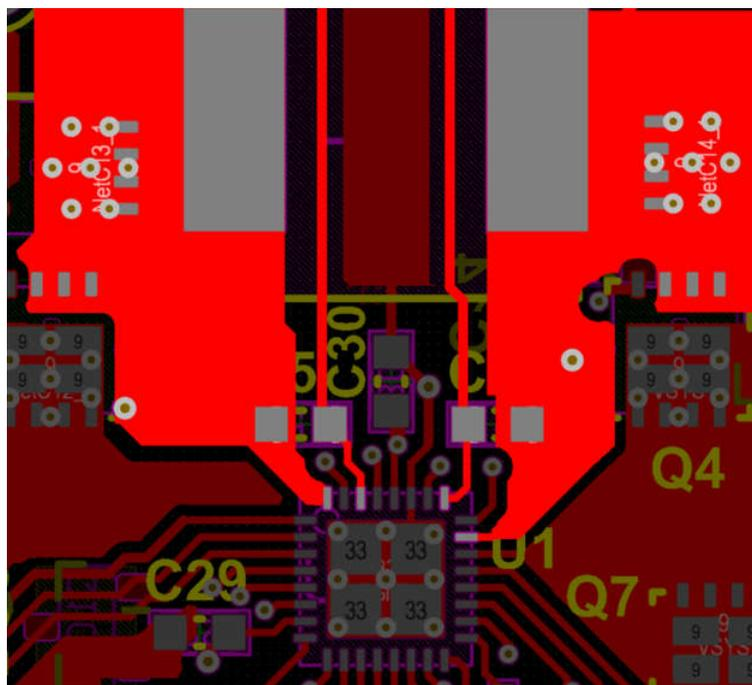
**Figure 2-7. Capacitors for BTST1/2 pins**
