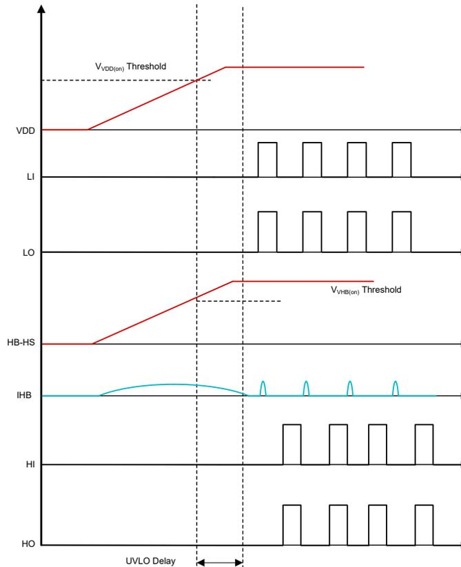
**Figure 1-2. Synchronous Buck Timing Diagram**
