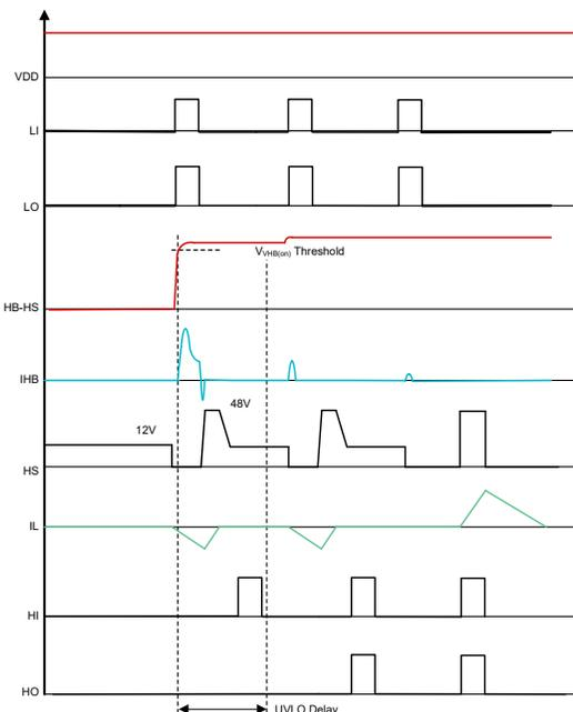
Figure 1-4. Timing Diagram of Inactive Phase Start-Up
