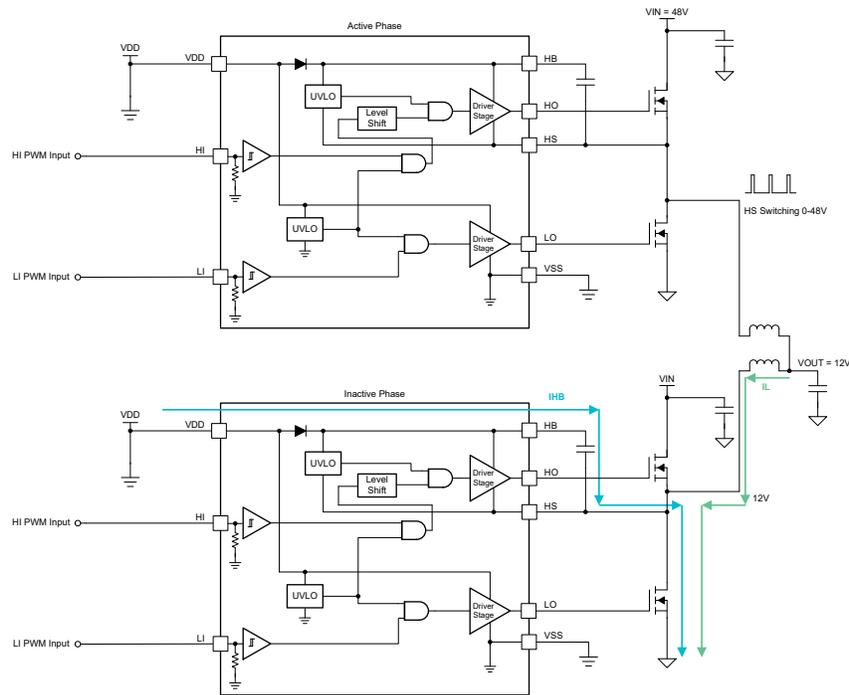
Figure 1-3. Multi-Phase Synchronous Buck-Boost HB Capacitor and Inductor Current Paths
