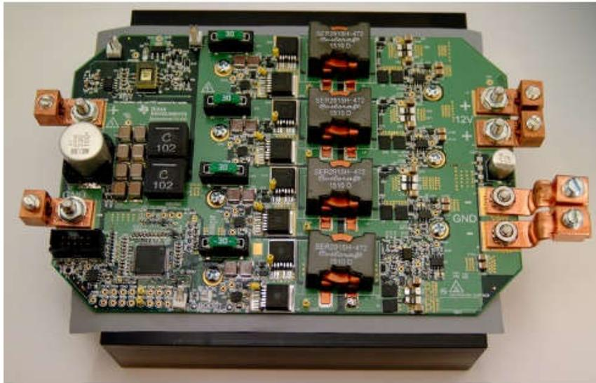
**Figure 9-6. TIDA-00653 Demonstrates Multiple Outputs Using One UCD3138128**
