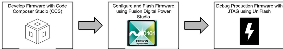
**Figure 8-1. UCD3138x Firmware Development Flow**
